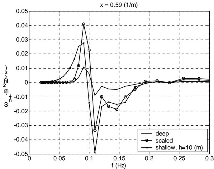
Fig. 3. Nonlinear transfer rates for a deep water JONSWAP spectrum with  $f_p=0.1$  Hz,  $\alpha=0.0175$ ,  $\gamma=3.3$  and a  $\cos^2(\theta)$ -directional spreading. Results for deep water, a depth of 10 m and the scaled nonlinear transfer rate.
