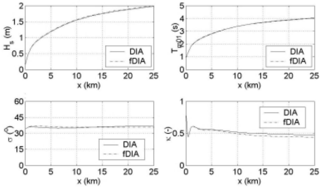
Fig. 6. Growth curves computed with the standard DIA (solid line) and finite depth DIA (fDIA, dashed line) for a constant water depth of 5 m and a wind speed of 25 m/s using the modified SWAN model.
