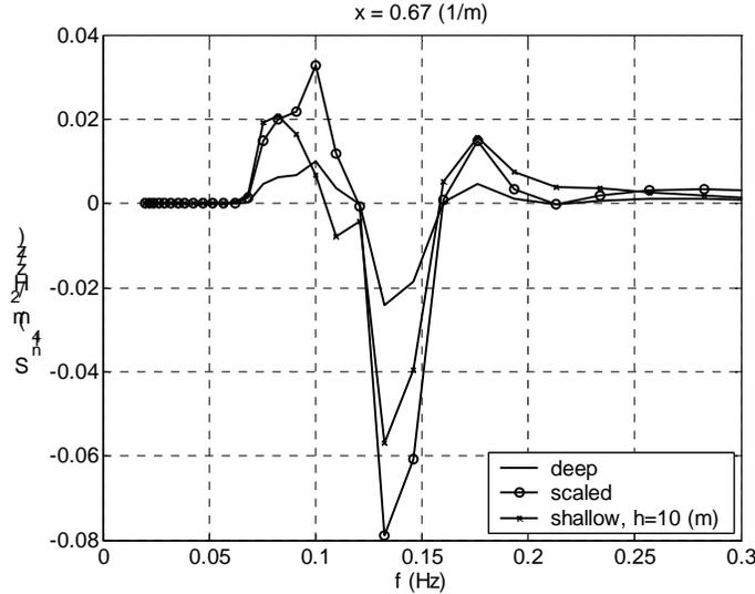
Fig. 5. Nonlinear transfer rate computed with the finite depth DIA for a deep water JONSWAP spectrum with  $f_p=0.1$  Hz,  $\alpha=0.0175$ ,  $\gamma=3.3$  and a  $\cos^2(\theta)$ -directional spreading. Results for deep water, a depth of 10 m and the scaled nonlinear transfer rate.
