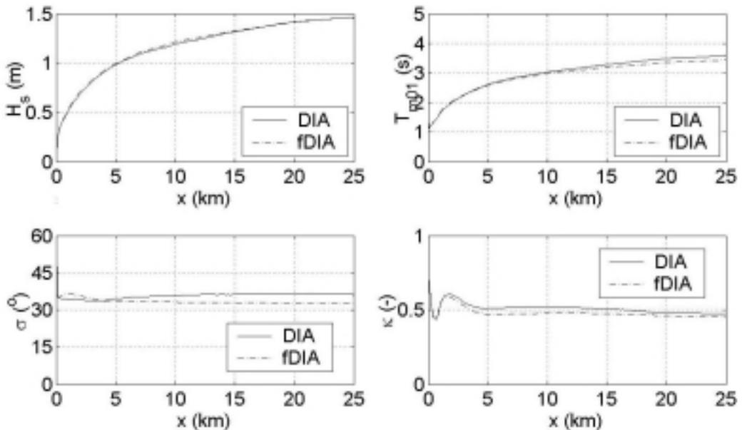
Fig. 7. Growth curves computed with the standard DIA (solid line) and finite depth DIA (fDIA, dashed line) for a constant water depth of 2 m and a wind speed of 25 m/s using the modified SWAN model.
