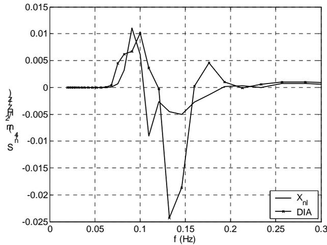
Fig. 2. Comparison of nonlinear transfer rate computed with an exact method (solid line) and with the DIA (solid line with crosses) for a deep water JONSWAP spectrum with  $f_p=0.1$  Hz,  $\alpha=0.0175$ ,  $\gamma=3.3$  and a  $\cos^2(\theta)$ -directional spreading.
