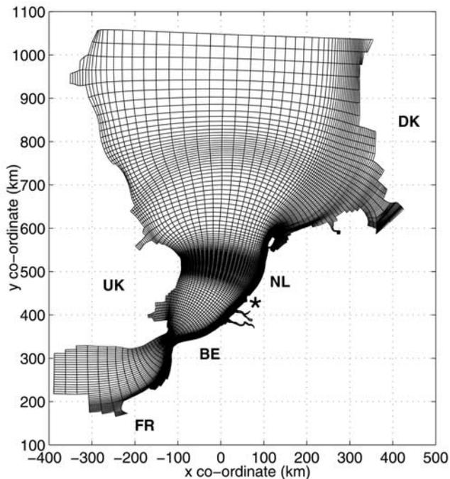
**Figure 4.** Large-scale computational grid from the PROMISE project. Port of Rotterdam is indicated by the asterisk.
