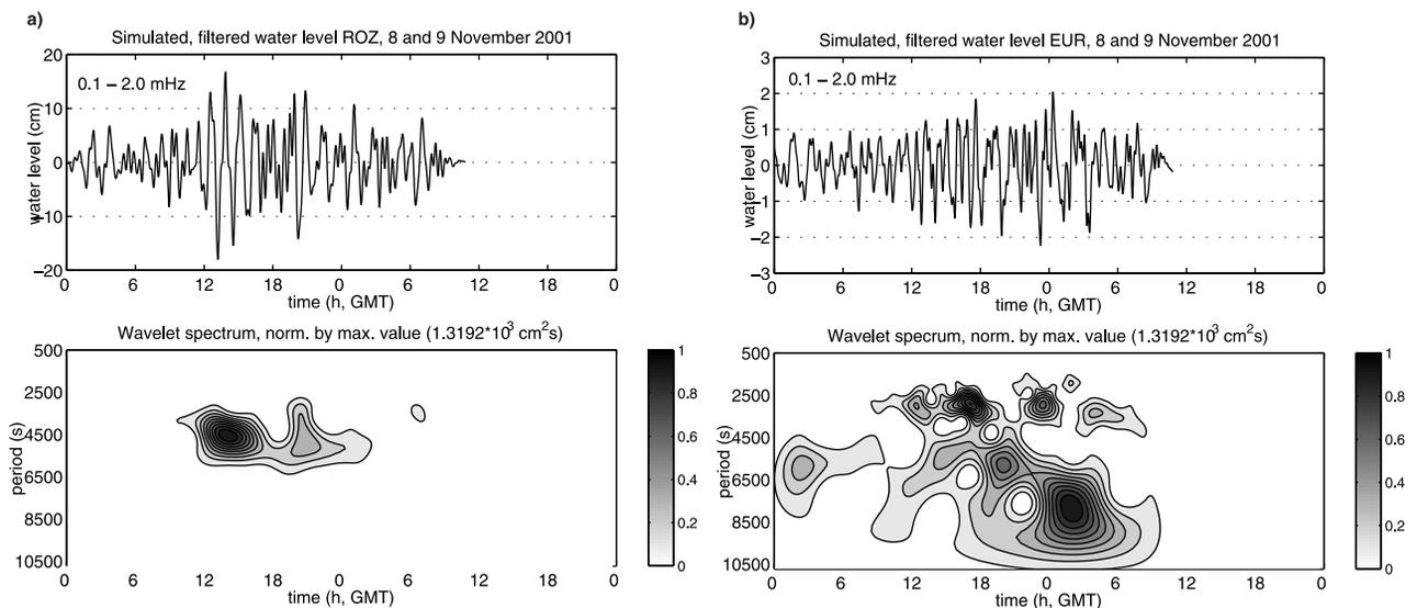
**Figure 12.** (left) (top) Simulated water level from ROZ (8 and 9 November 2001) and (bottom) the corresponding wavelet spectrum. (right) (top) Simulated water level from EUR (8 and 9 November 2001) and (bottom) the corresponding wavelet spectrum.
