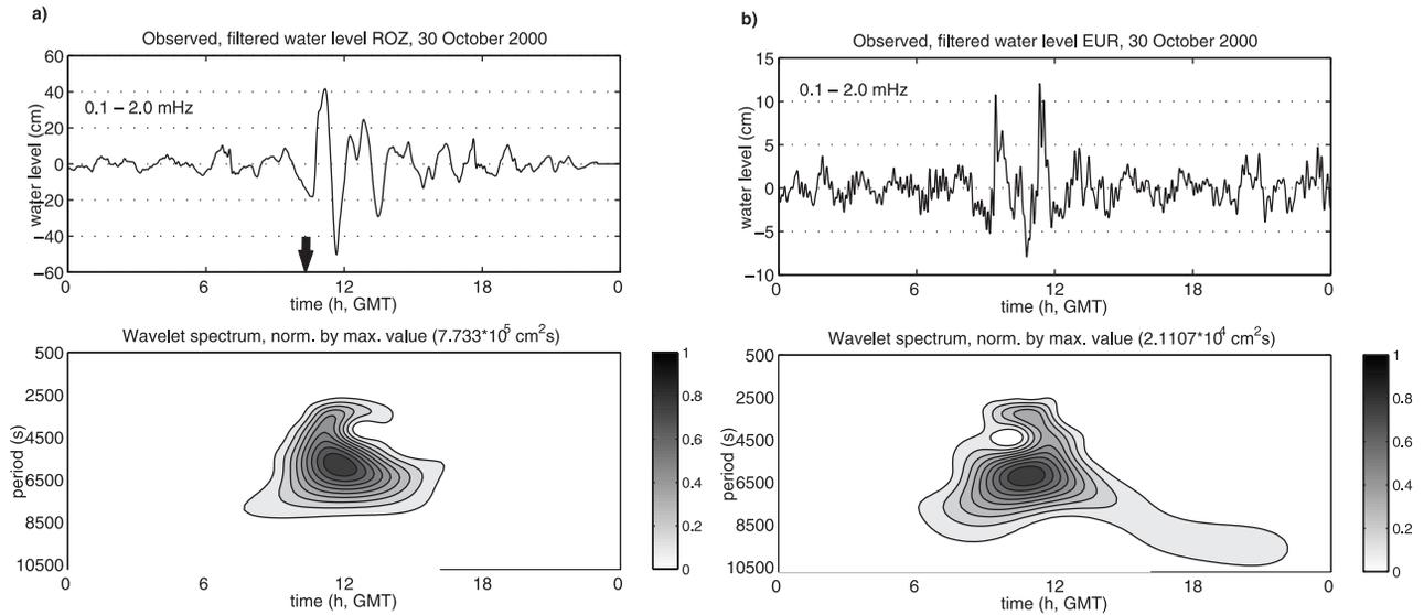
**Figure 9.** (left) Filtered observed surface elevation at ROZ on 30 October 2000 ((top) Arrow indicates the approximate time of the front passage over the harbor area) and (bottom) the corresponding wavelet spectrum. (right) Filtered observed surface elevation at sea ((top) location EUR, 30 October 2000) and (bottom) the corresponding wavelet spectrum.
