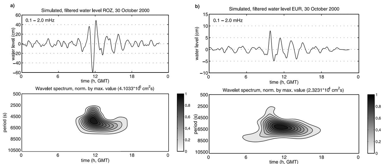
**Figure 10.** (left) (top) Simulated seiche at ROZ (30 October 2000) and (bottom) the corresponding wavelet spectrum. (right) (top) Simulated water level at EUR (30 October 2000) and (bottom) the corresponding wavelet spectrum.
