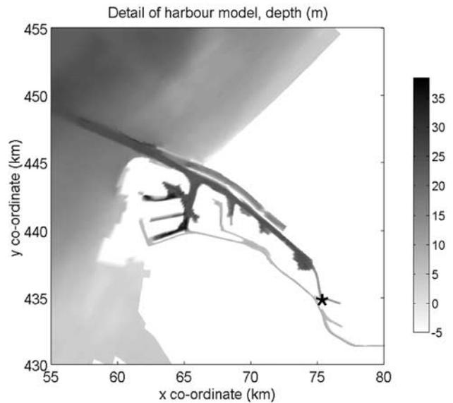
**Figure 6.** Detail of small-scale computational grid, showing depth values in meters. The location of ROZ is indicated by the asterisk.
