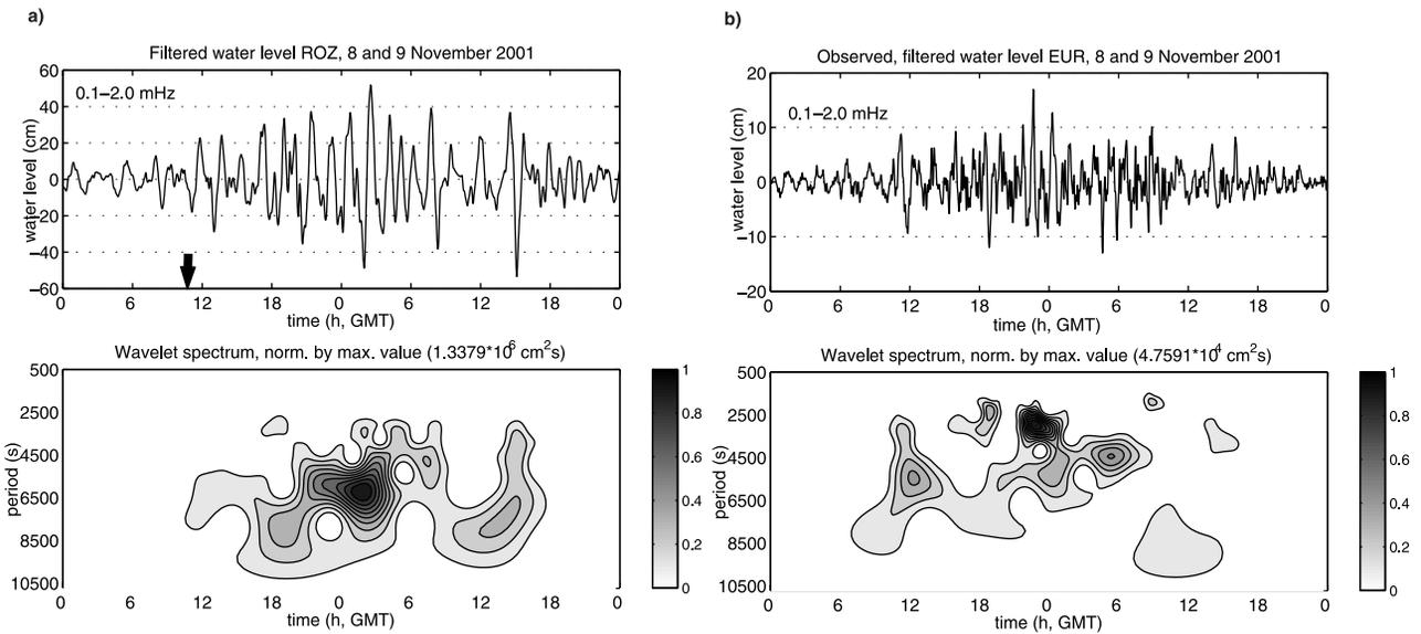
**Figure 11.** (left) Filtered observed surface elevation measurements at ROZ on 8 and 9 November 2001 ((top) Arrow indicates the approximate time of the front passage over the harbor area) and (bottom) the corresponding wavelet spectrum. (right) (top) Filtered observed surface elevation measurements from EUR (8 and 9 November 2001) and (bottom) the corresponding wavelet spectrum.
