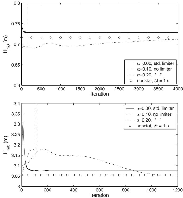
Fig. 5. Convergence behaviour of  $H_{m0}$  in deep-water, fetch-limited simulations for wind speeds  $U_{10}=10$  (top panel) and 30 m/s (bottom panel), at fetch=12.5 km. Results for SWAN without limiter ( $\gamma=\infty$ ) and various large under-relaxation factors ( $\alpha=0.10$ – $0.20$ ). Also shown are stationary SWAN with  $\gamma=0.1$  and  $\alpha=0$ , and nonstationary SWAN with  $\Delta t=1$  s.
