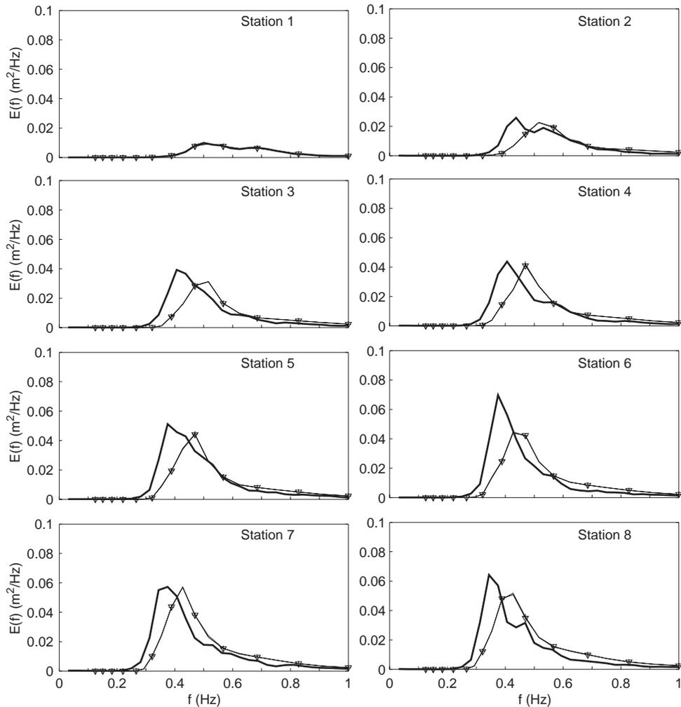
Fig. 7. Lake George field experiment of near-idealized, depth-limited wave growth. 1D spectra obtained with  $\alpha=0.0$  and  $\gamma=0.1$  after 500 iterations (plusses), with  $\alpha=0.05$  and  $\gamma=0.5$  after 500 iterations (triangles) and observations of Young and Verhagen (1996) (thick line). Note: all plusses virtually coincide with the triangles and for that reason are not separately visible.
