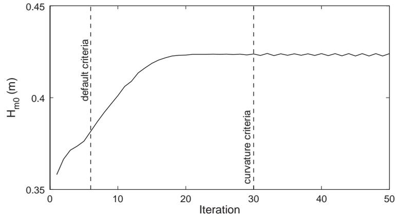
Fig. 9. Lake George field experiment of near-idealized, depth-limited wave growth (Station 8). Iteration behaviour of SWAN with  $\alpha=0.0$  and  $\gamma=0.1$  with positions of run termination using default stopping criteria (14) and (15) with  $\varepsilon_{H^r}=\varepsilon_T^r=0.02$ ,  $\varepsilon_{H^a}=0.02$  m and  $\varepsilon_T^a=0.2$  s (6 iterations) and criteria (14) and (22) with  $\varepsilon_{H^r}=0.02$ ,  $\varepsilon_{H^a}=0.02$  m and  $\varepsilon_C=0.0001$  (30 iterations).
