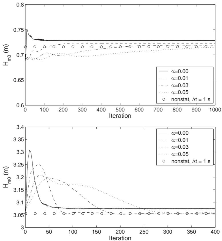
Fig. 3. Convergence behaviour of  $H_{m0}$  in deep-water, fetch-limited simulations for wind speeds  $U_{10}=10$  (top panel) and 30 m/s (bottom panel), at fetch=12.5 km. Results for SWAN with  $\gamma=0.1$  and  $\alpha=0.0-0.05$ . Also shown is nonstationary SWAN with  $\Delta t=1$  s.
