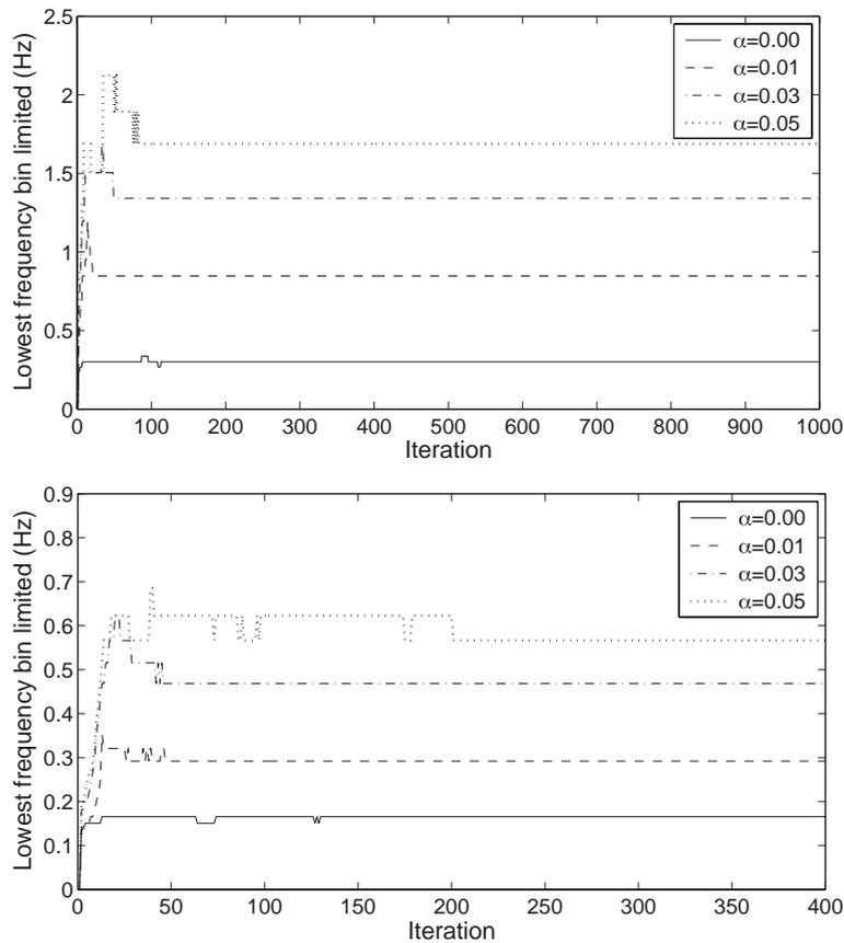
Fig. 4. Lowest frequency bin at which limiter is active, as a function of iteration level. Results for deep-water, fetch-limited simulations for wind speeds  $U_{10}=10$  (top panel) and 30 m/s (bottom panel), with  $\gamma=0.1$  and  $\alpha=0.0-0.05$ .
