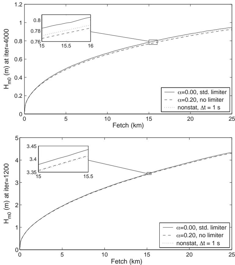
Fig. 6. Growth curves of  $H_{m0}$  in deep-water, fetch-limited simulations for wind speeds of  $U_{10}=10$  (top panel) and 30 m/s (bottom panel). Results for stationary SWAN with limiter, for  $\alpha=0.20$  without limiter and nonstationary SWAN with  $\Delta t=1$  s.
