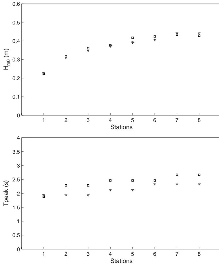
Fig. 8. Lake George field experiment of near-idealized, depth-limited wave growth. Wave height and peak period obtained with  $\alpha=0.0$  and  $\gamma=0.1$  after 500 iterations (plusses), with  $\alpha=0.05$  and  $\gamma=0.5$  after 500 iterations (triangles) and observations of Young and Verhagen (1996) (squares). Note: all plusses virtually coincide with the triangles and for that reason are not separately visible.
