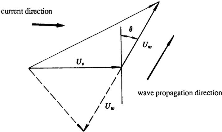
Fig. 2. Wave and current propagation directions and vector summation of velocities.
