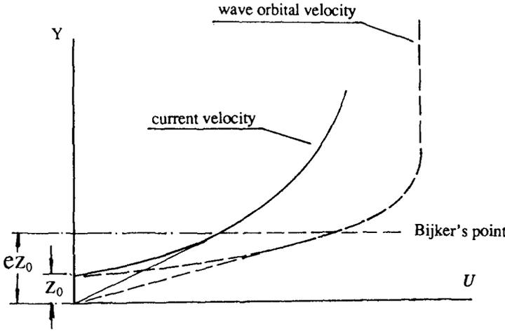
Fig. 1. Schematic diagram of wave and current velocity distributions considered by Bijker (1966).
