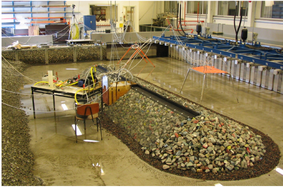
Fig. 3. Layout in shallow water wave basin at Aalborg University for testing waves with wave obliquity equal to 0° and 10°. From Lykke Andersen and Burcharth (2004).
