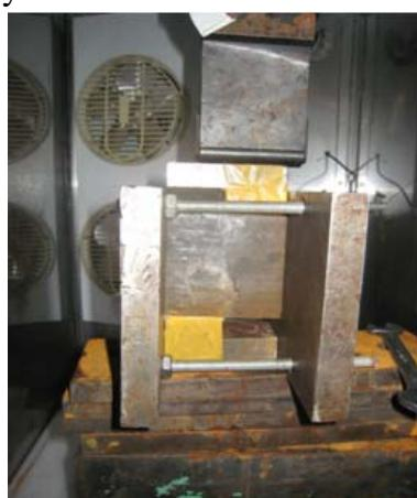
**Figure 2.**Sea ice shear test systems.
