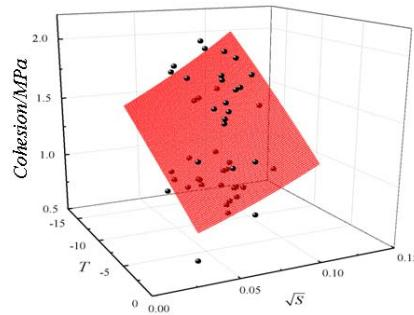
**Figure 6.**Cohesion with temperature and salinity.
