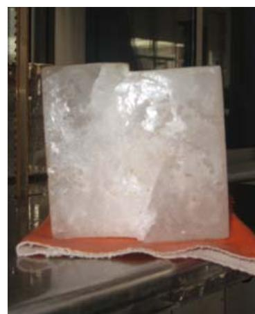
**Figure 3.**Sea ice shear failure.
