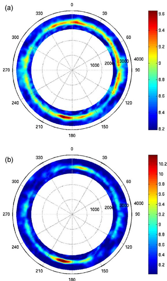
**Fig. 10.** (a) Noise power from beamforming analysis in January 2004, for the period band 10–20 s. The noise mainly arrives from the south–southwest and from between the north–northwest and east–southeast. The apparent velocity is around 3200 m/s. (b) Noise power from beamforming analysis in July 2004, for the period band 10–20 s. The noise mainly arrives from the south–southwest. The apparent velocity is around 3200 m/s.
