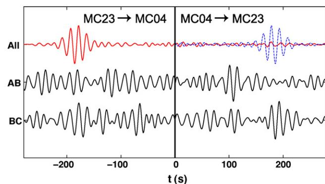
Fig. 7. EGFs (black traces) in the period band 10–20 s for MC04–MC23 from surface wave coda of the large earthquakes ( $m_b \geq 5$ , red dots in Fig. 3d) in two different time windows (AB and BC, each with 800 s length) shown at the left side of each black trace. The detailed definition of these two coda windows is given in Fig. 2 and Section 3.4. The coda in the window AB and BC is the earlier and later part of surface wave coda, respectively.
