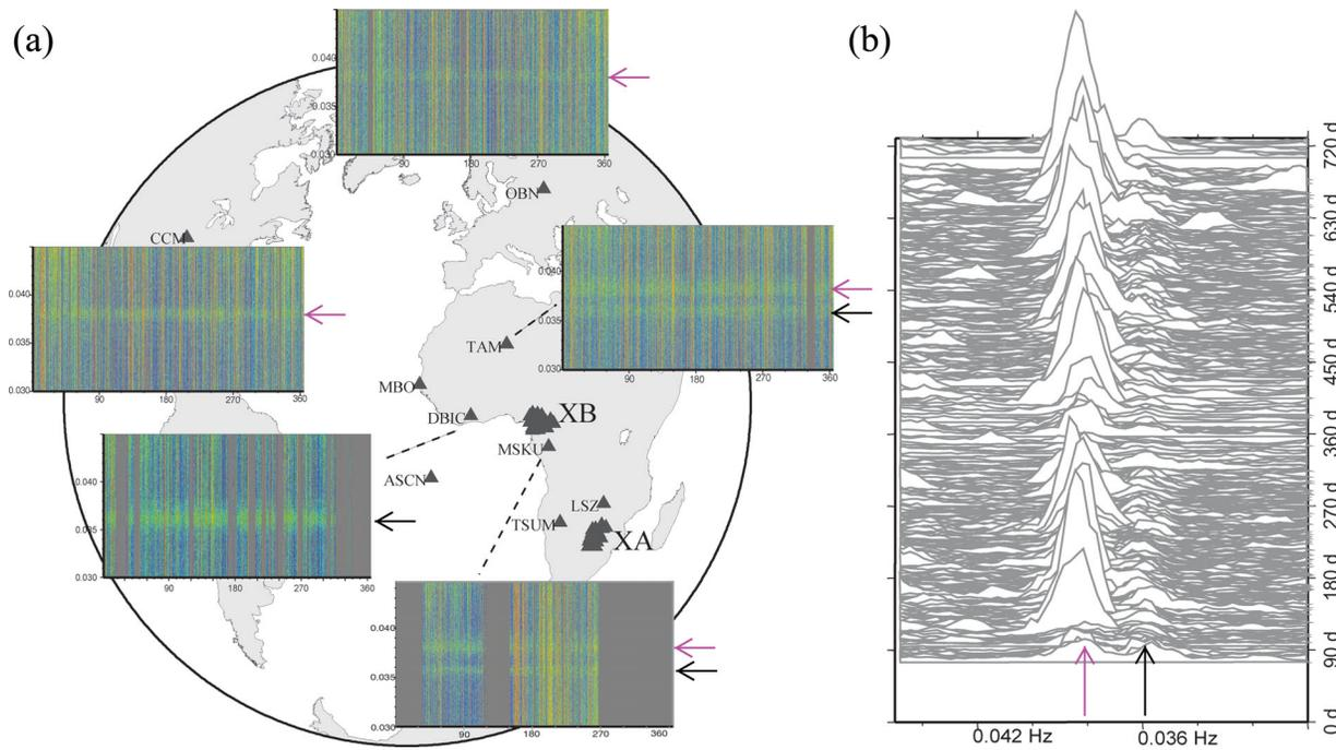
**Figure 1.** (a) Broad-band seismograph stations (triangle, station CM03 is in temporal array XB) and spectrograms at five stations for year 1999. The 0.038 Hz microseism (indicated with pink arrow) and 0.036 Hz microseism (black arrow) are continuous, demonstrating their persistent nature. (b) Temporal variation of spectral amplitude at TAM in years 1997 and 1998.
