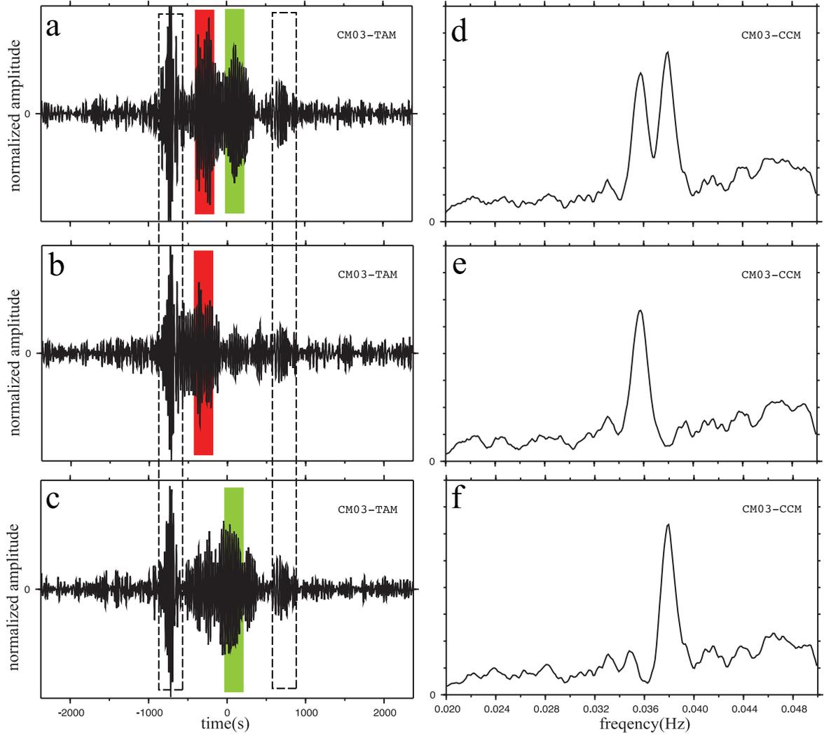
**Figure 2.** NCFs between TAM and CM03 for Band1 (a), Band2 (b) and Band3 (c) (see text for definition of Band1,2 and 3). The energy packet associated with the 0.036 Hz microseism is indicated with red box, and the 0.038 Hz with green box. The Rayleigh wave signal from the ambient seismic noise is indicated with grey boxes. (d,e and f) Spectra of the NCFs in panels (a, b and c), respectively.
