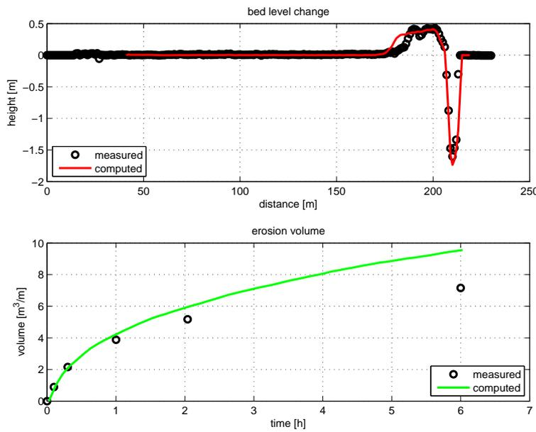
Figure 4.50: Erosion pattern and volumes and retreat distance during test DP01
