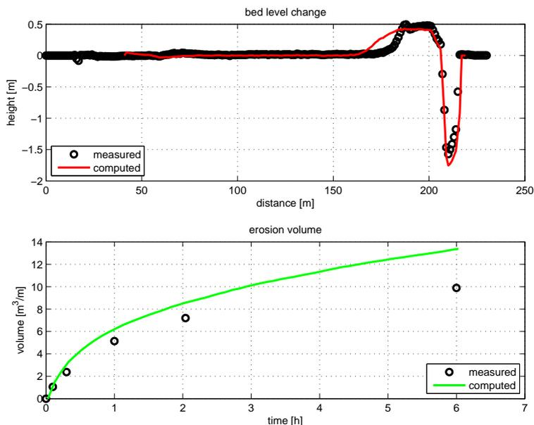
Figure 4.44: Erosion pattern and volumes and retreat distance during test T03
