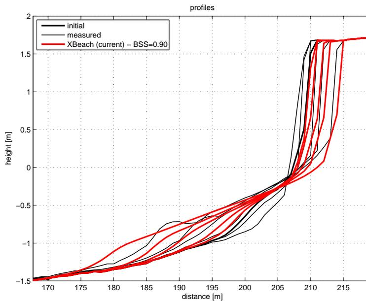
Figure 4.39: Profile development during test T01
