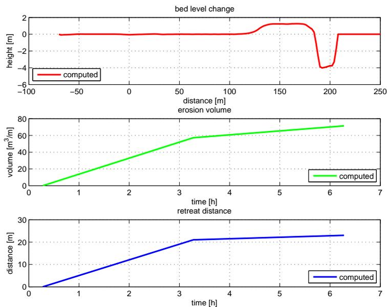
Figure 4.19: Development of erosion volumes during test 5
