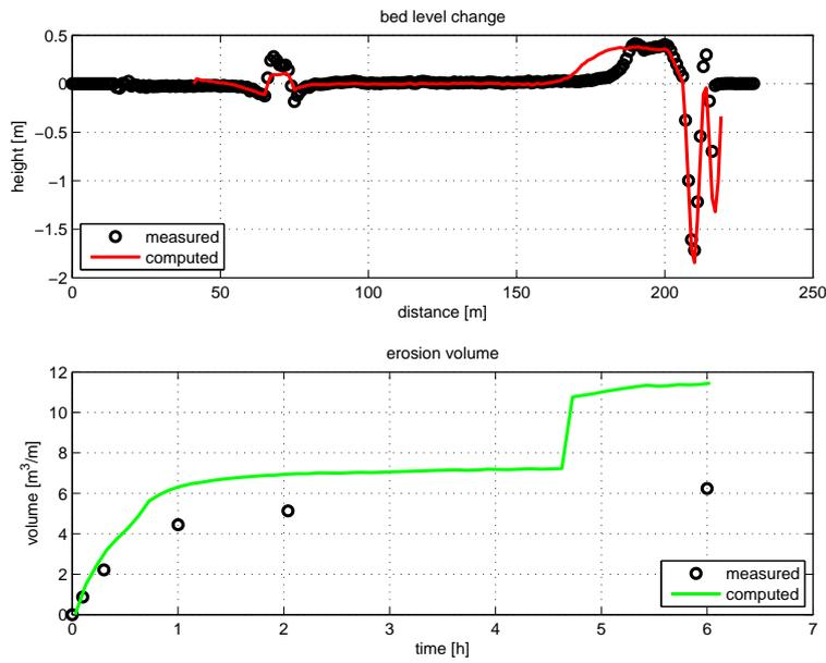
Figure 4.55: Erosion pattern and volumes and retreat distance during test T04
