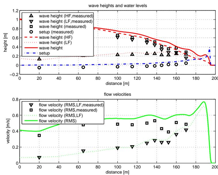
Figure 4.26: Hydrodynamics during test 1B
