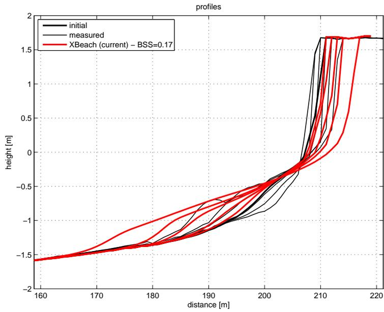
Figure 4.49: Profile development during test DP02
