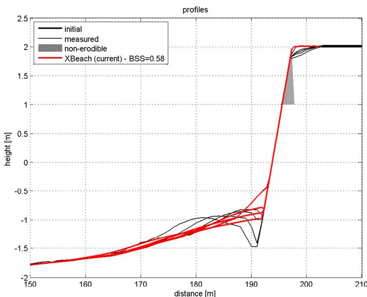
Figure 4.20: Profile development during test T1
