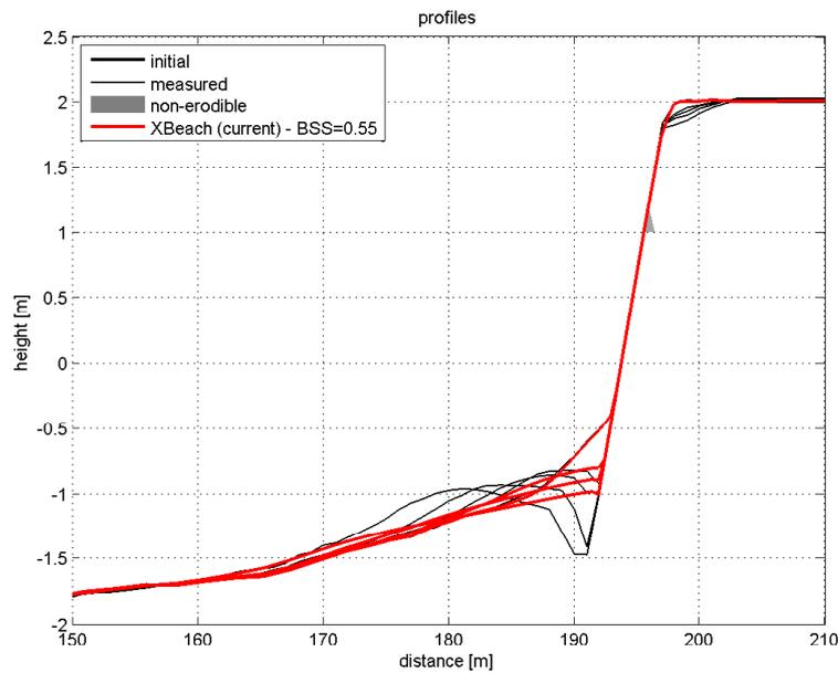
Figure 4.21: Profile development during test T2
