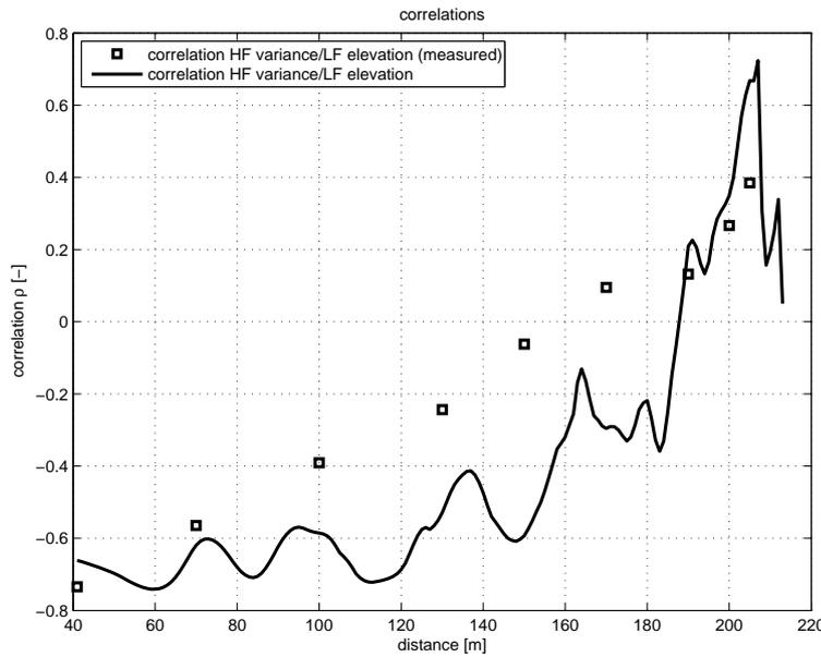
Figure 4.31: Correlation between short wave variance and long wave surface elevations
