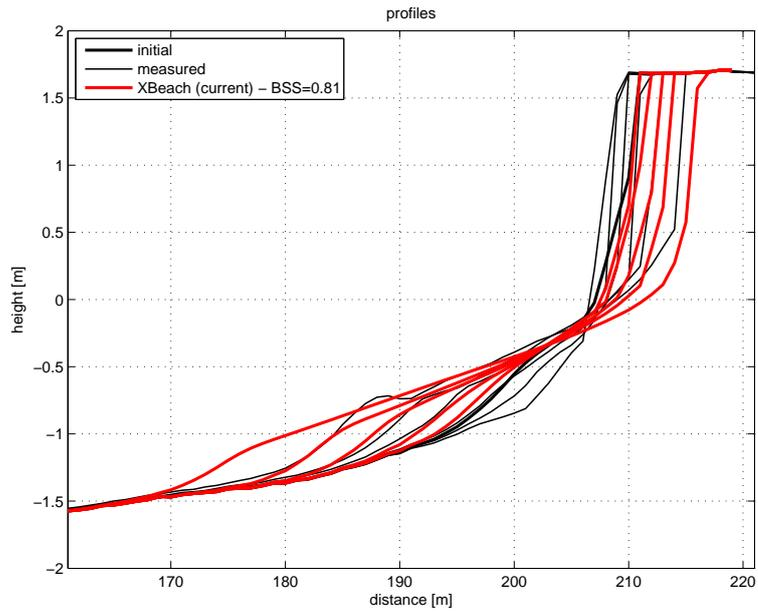
Figure 4.40: Profile development during test T02
