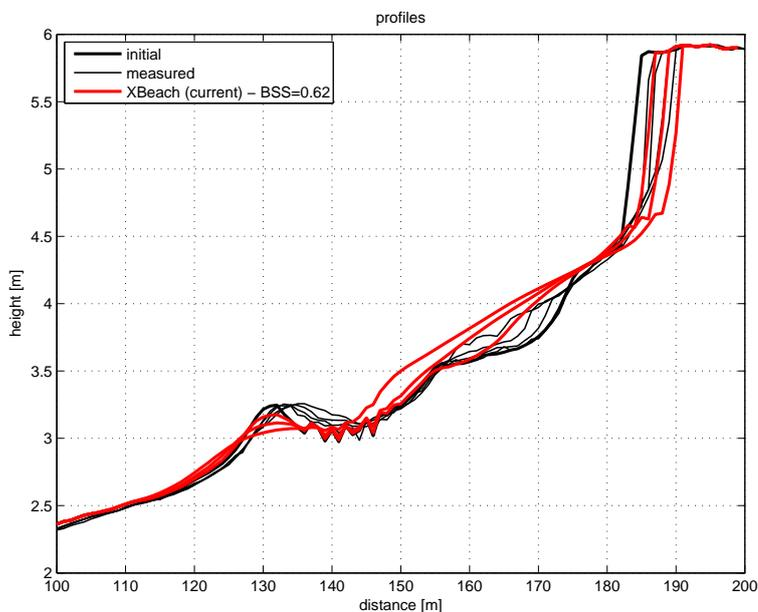
Figure 4.25: Profile development during test 2E
