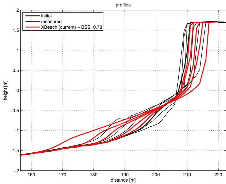
Figure 4.41: Profile development during test T03
