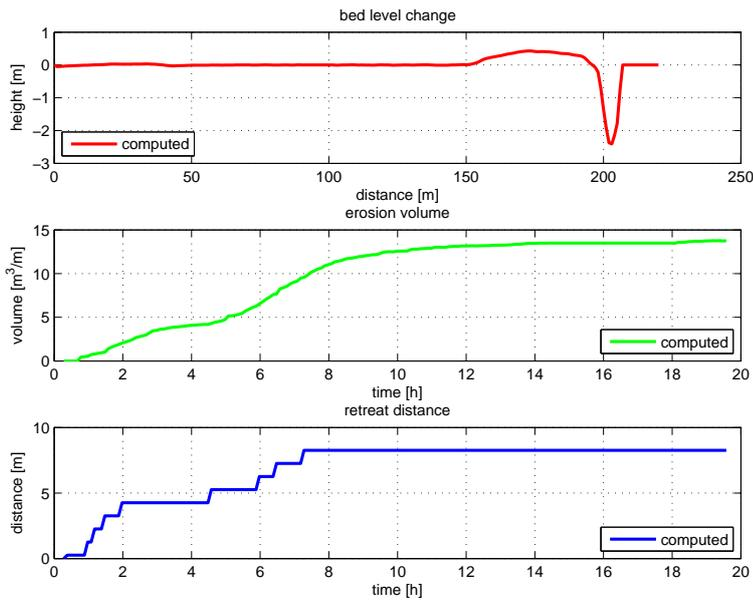
Figure 4.17: Development of erosion volumes during test 3
