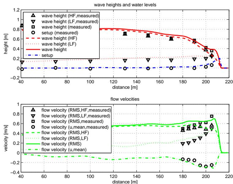
Figure 4.52: Hydrodynamics during test DP01
