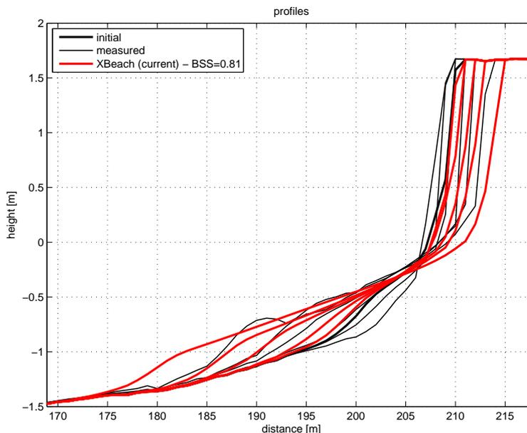
Figure 4.48: Profile development during test DP01
