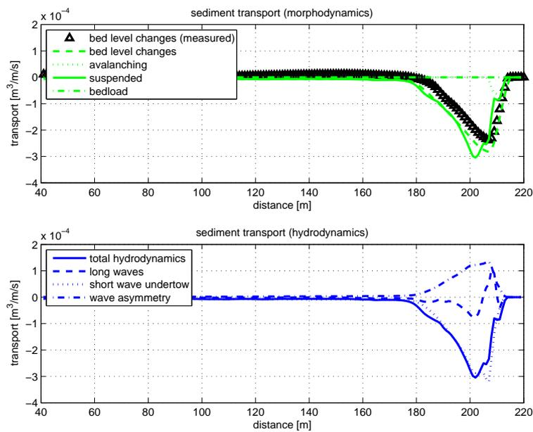
Figure 4.36: Sediment transports by transport type and forcing
