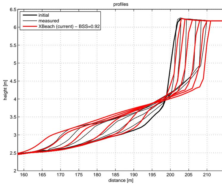
Figure 4.10: Profile development during test 2
