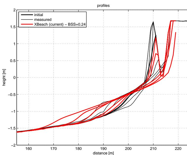
Figure 4.54: Profile development during test T04
