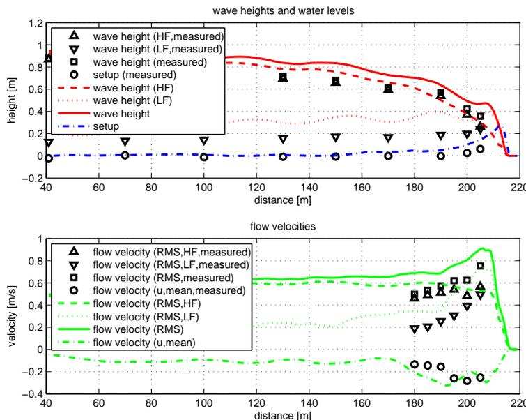
Figure 4.53: Hydrodynamics during test DP02
