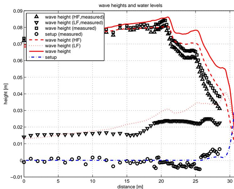
Figure 3.7: Wave height transformations during Boers 1C experiment
