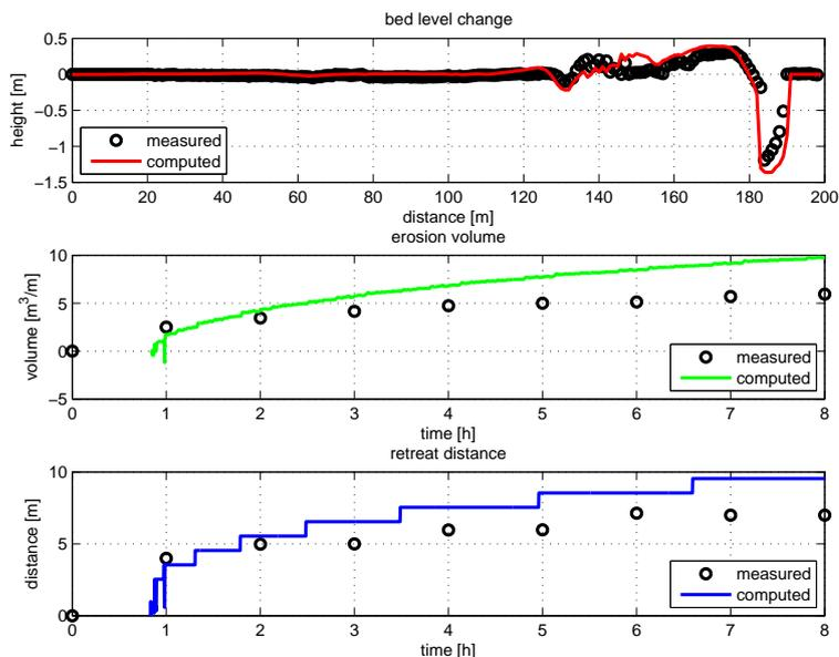
Figure 4.24: Morphodynamics during test 2E
