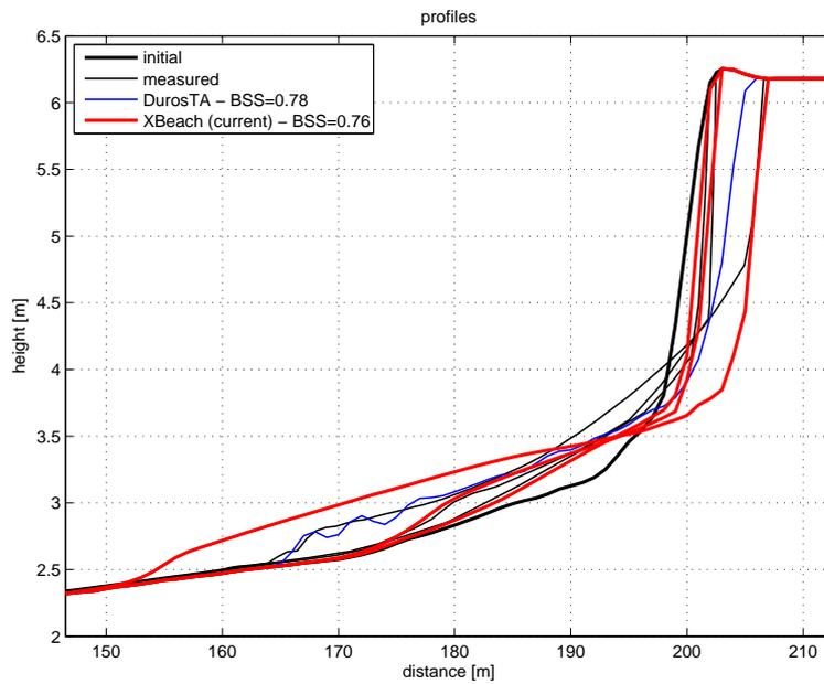
Figure 4.11: Profile development during test 3
