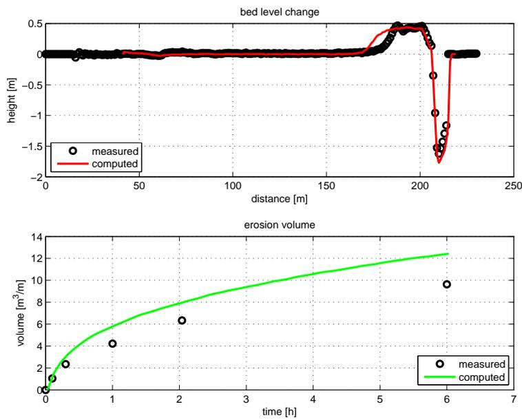
Figure 4.43: Erosion pattern and volumes and retreat distance during test T02
