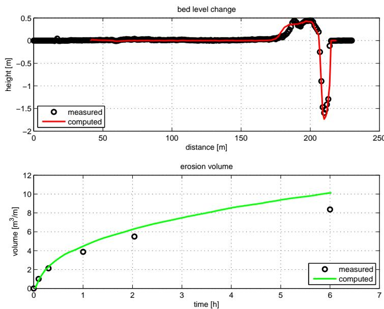
Figure 4.38: Bed level changes and erosion volumes
