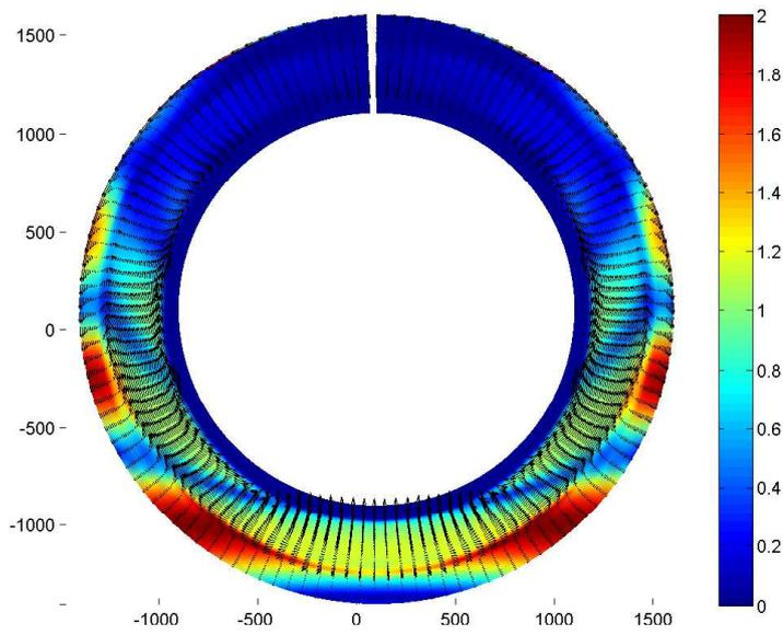
Figure 7.6: Snapshot of the RMS wave height and the flow velocity field in the last time step
