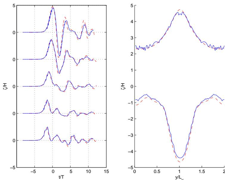
Figure 3.5: Normalized vertical runup in time (panel 1) and maximum and minimum values (panel 2)
