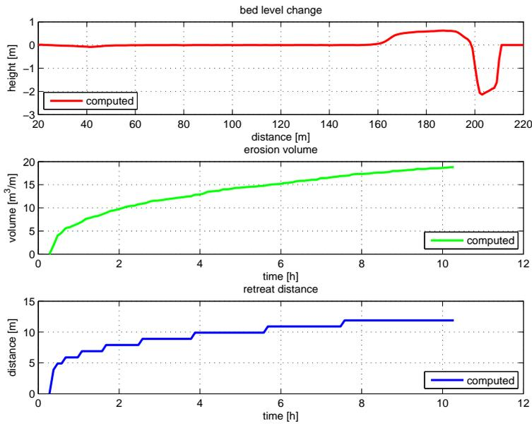
Figure 4.16: Development of erosion volumes during test 2
