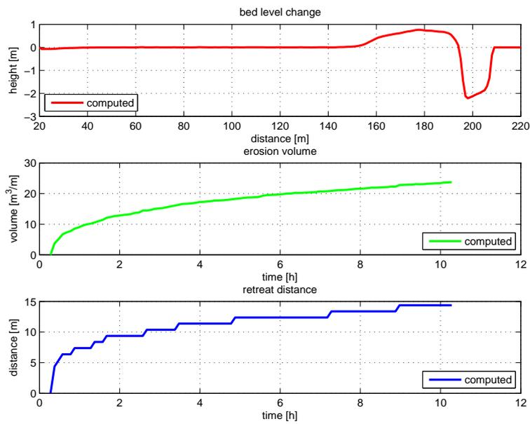
Figure 4.15: Development of erosion volumes during test 1
