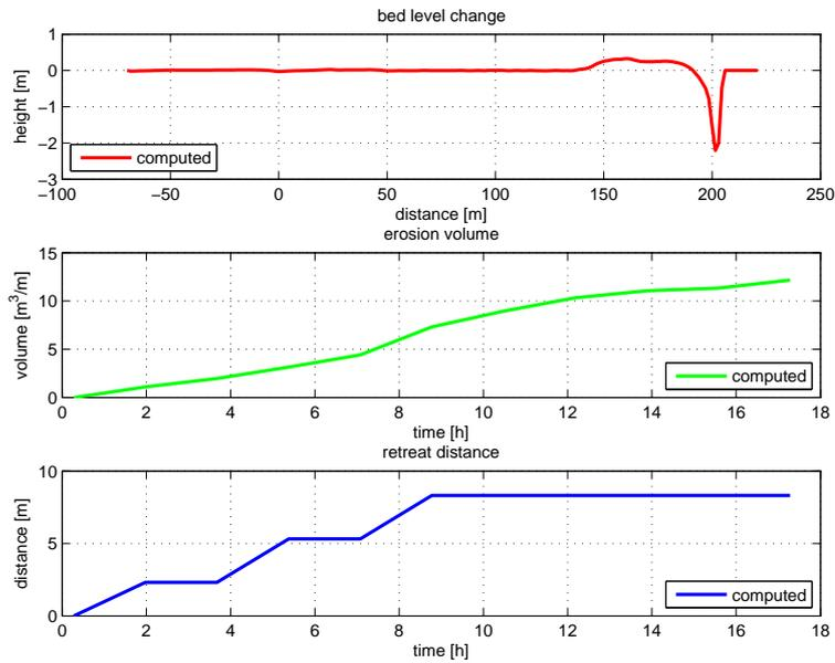
Figure 4.18: Development of erosion volumes during test 4
