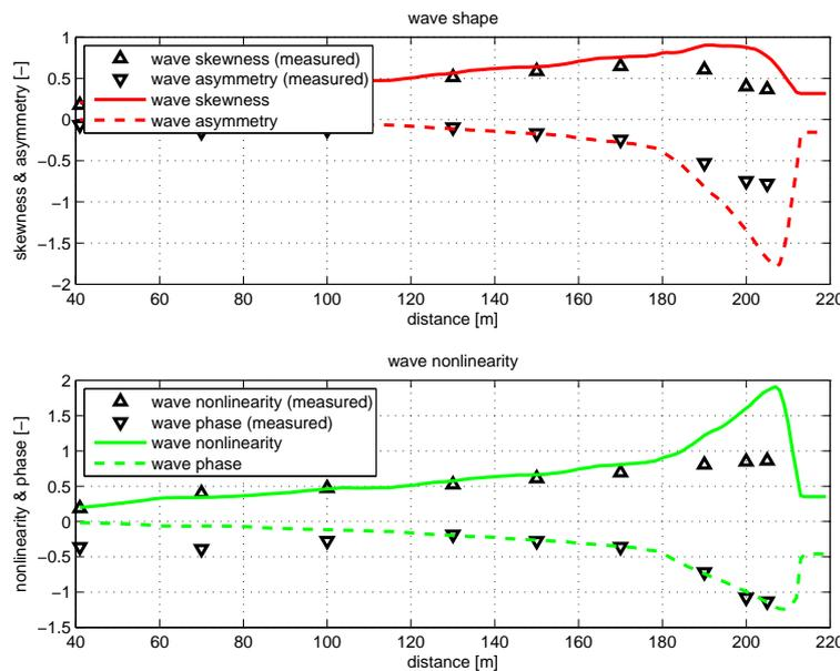
Figure 4.32: Wave shape and nonlinearity
