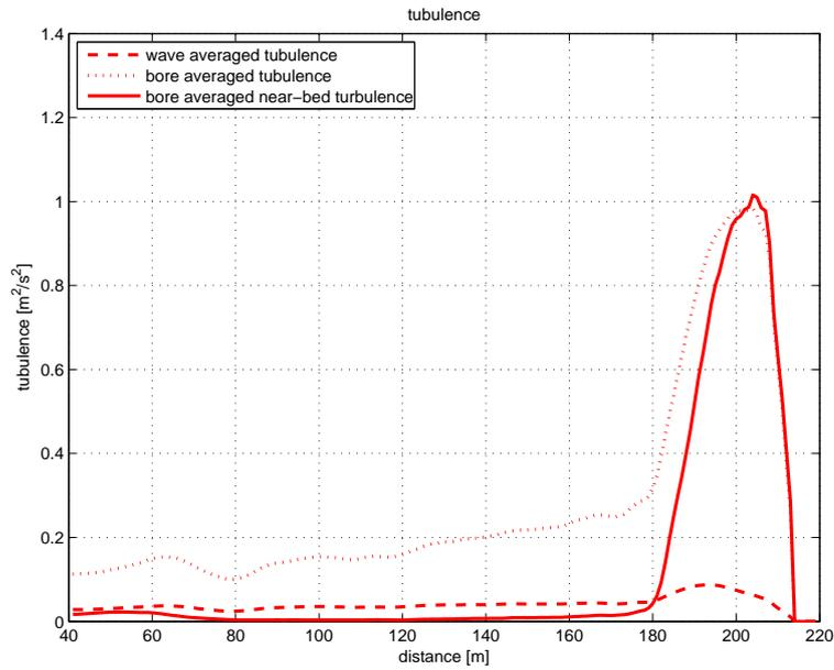
Figure 4.35: Wave induced turbulence
