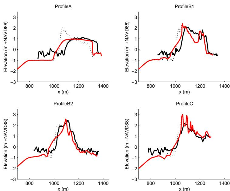
Figure 5.6: Pre-storm profiles (black dotted line), measured post-storm profiles (black solid line) and modelled post-storm profiles (red solid line). Upper left panel: profile A. Upper right panel: profile B1. Lower left panel: profile B2. Lower right panel: profile C. The seaward side is on the left in all panels. Note that the measured post-storm profiles contain only the sea surface and emerged topography and no submerged topography.
