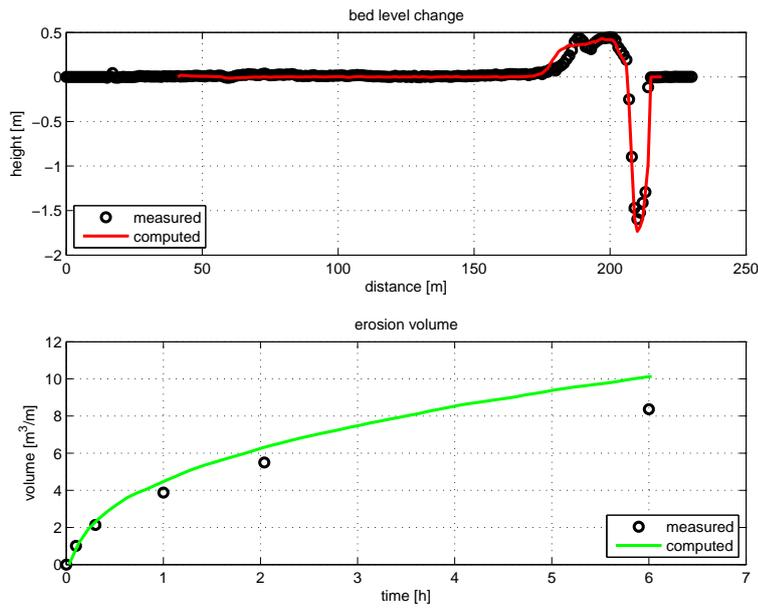
Figure 4.42: Erosion pattern and volumes and retreat distance during test T01
