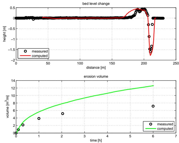
Figure 4.51: Erosion pattern and volumes and retreat distance during test DP02
