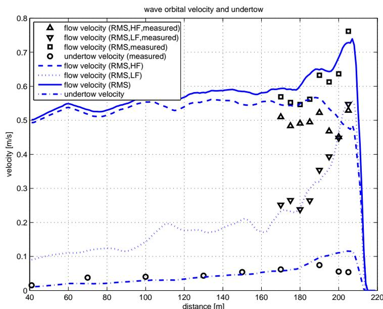
Figure 4.33: Wave motion velocities and undertow
