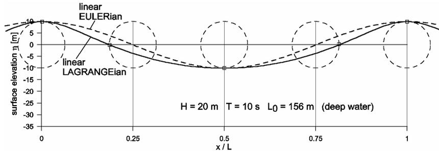
Figure 1: Surface of a regular deepwater wave ( $H = 20$  m,  $T = 10$  s) from LAGRANGEian treatment of linear wave theory
