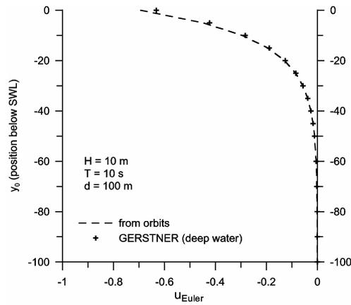
Figure 6: Negative EULERian current from closed orbits and mass transport according to the theory of Gerstner
