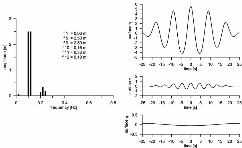
Figure 9: Second order results according to Sand and Mansard, 1986 and Sand, 1982
