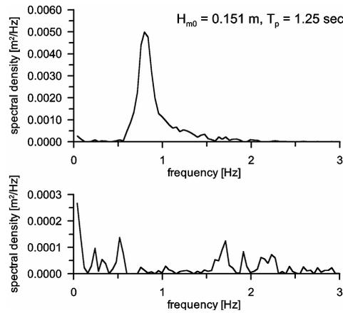
Figure 11: Non-linear spectrum from LAGRANGEian superposition
