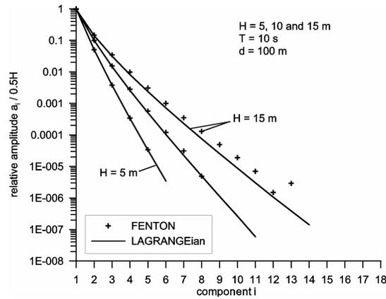
Figure 3: Comparison of (relative) higher order components after Fenton (Aces 1992) with results from LAGRANGEian treatment of linear wave theory (deepwater,  $H = 5$  m,  $10$  m and  $15$  m,  $T = 10$  s)
