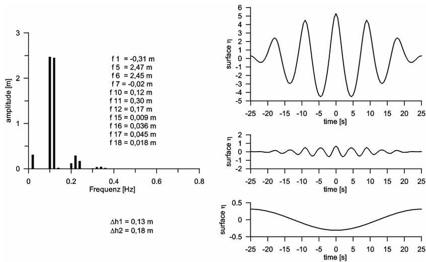
Figure 8: LAGRANGEian superposition of two linear waves
