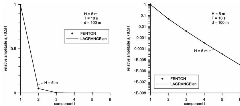
Figure 2: Comparison of (relative) higher order components after FENTON (ACES 1992) with results from LAGRANGEian treatment of linear wave theory (deepwater) ( $H = 5$  m,  $T = 10$  s)
