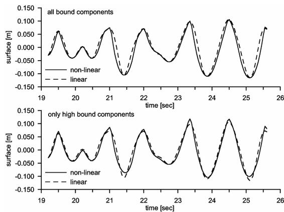
Fig. 13: Time-series from LAGRANGEian and linear superposition top: all bound components bottom: bound higher components only
