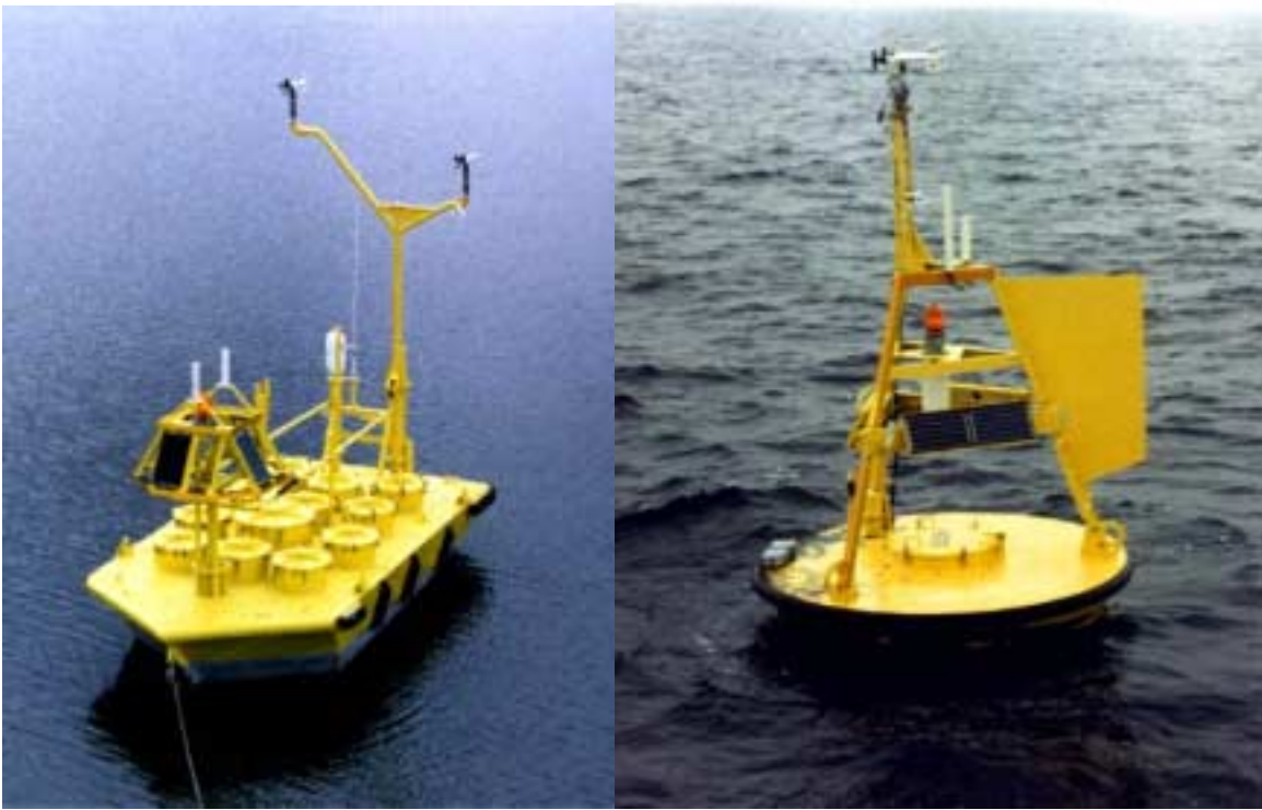
Figure 2.4. Different types of NDBC buoys. The buoy on the left is a 6-meter nomad non-directional buoy and the one on the right is a 3-meter discus buoy, which can be directional or non-directional.
