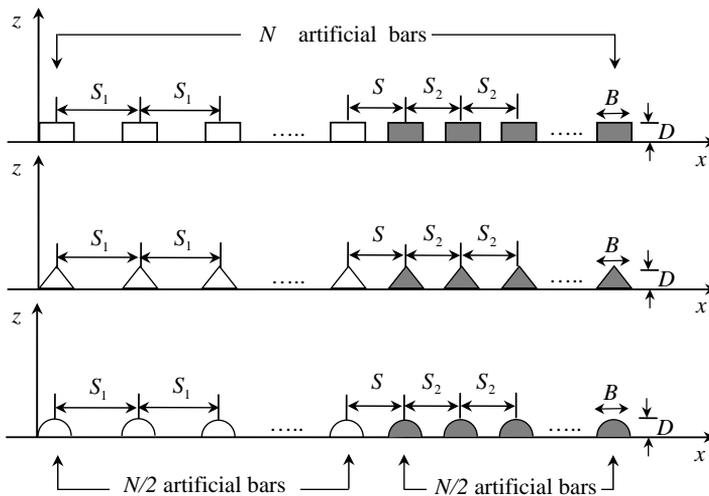
Fig. 1. Shapes of doubly composite artificial bars with different spacings: (a) rectangular bar; (b) triangular bar; and (c) rectified cosine bar.
