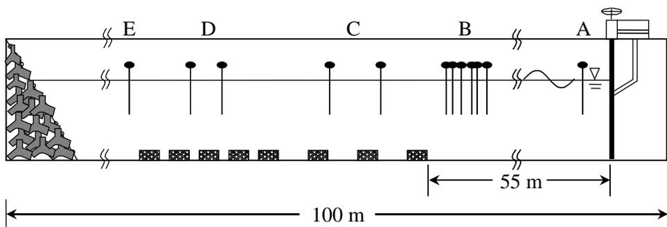
Fig. 2. Wave flume system and bar field placement.
