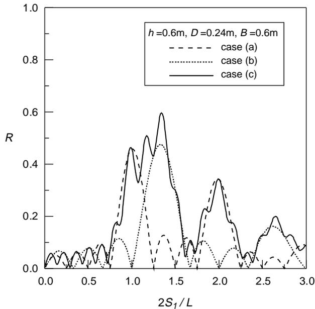
Fig. 4. Reflection coefficients with doubly composite rectangular artificial bars: (a)  $N=4$ ,  $S=2.4$  m; (b)  $N=4$ ,  $S=1.8$  m; (c)  $N_1=4$ ,  $N_2=4$ ,  $S_1=2.4$  m,  $S_2=1.8$  m.
