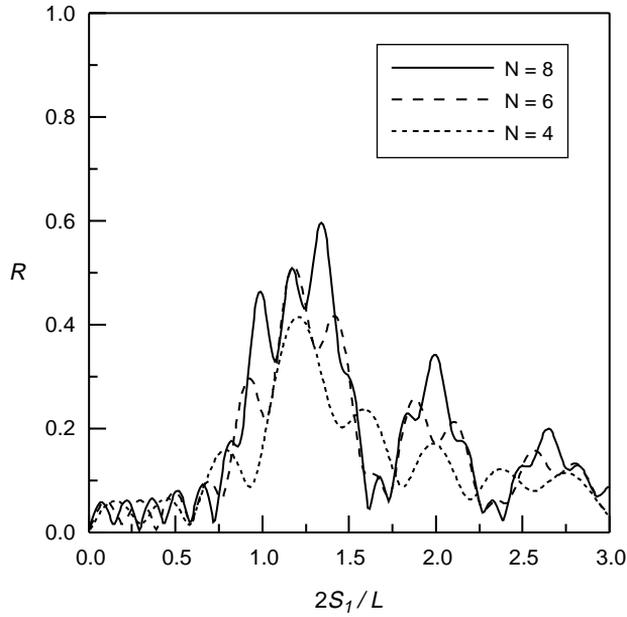
Fig. 10. Reflection coefficients with doubly composite rectangular artificial bars with different number of bars ( $S_2/S_1=0.75$ ,  $D/h=0.25$ , and  $B/S_1=0.25$ ).
