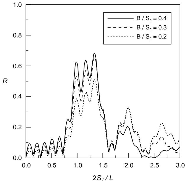
Fig. 12. Reflection coefficients with doubly composite rectangular artificial bars with different relative bar footprints ( $N=8$ ,  $S_2/S_1=0.75$ , and  $D/h=0.4$ ).
