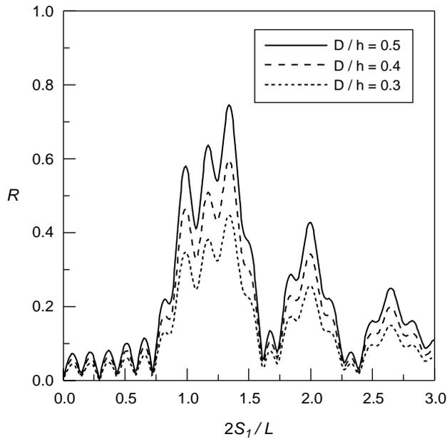
Fig. 11. Reflection coefficients with doubly composite rectangular artificial bars with different relative bar heights ( $N=8$ ,  $S_2/S_1=0.75$ , and  $B/S_1=0.25$ ).
