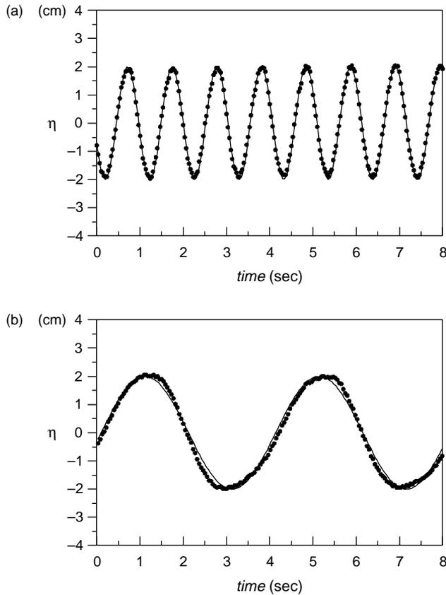
Fig. 3. Comparison of measured surface elevations with the linear wave theory: (a)  $T=1.03$  s; (b)  $T=4.03$  s; —, linear theory; ●, measurements.
