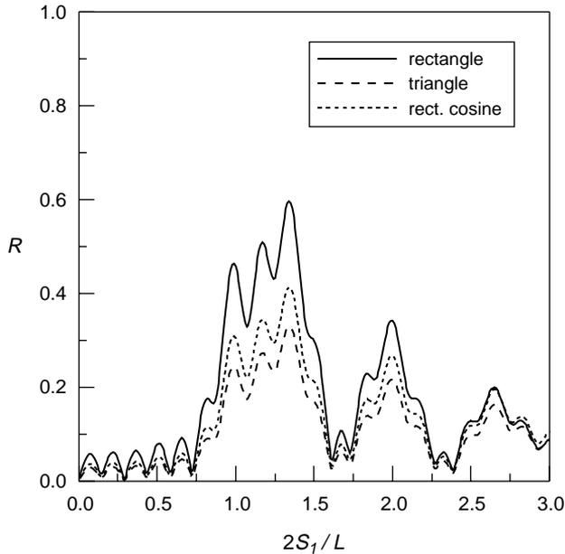
Fig. 14. Reflection coefficients of different shapes of doubly composite artificial bars ( $N=8$ ,  $S_2/S_1=0.75$ ,  $D/h=0.4$ , and  $B/S_1=0.25$ ).
