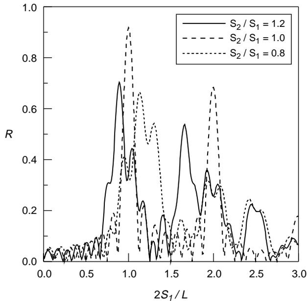
Fig. 13. Reflection coefficients with doubly composite rectangular artificial bars with different ratios of bar spacing ( $N=8$ ,  $D/h=0.4$  and  $B/S_1=0.25$ ).
