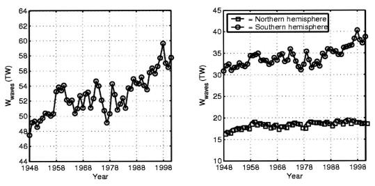
FIG. 5. Interannual variability of wind stress work on the surface waves for (left) global ocean and (right) both hemispheres (TW), calculated from (11).
