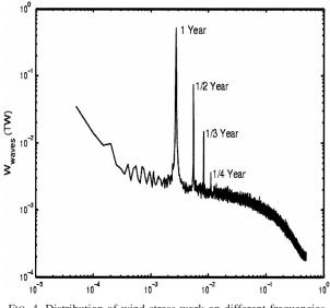
FIG. 4. Distribution of wind stress work on different frequencies (TW), calculated from (11).
