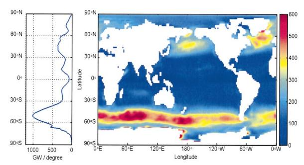
FIG. 3. (right) Distribution of wind stress work on the surface waves (mW m<sup>-2</sup>) calculated from (2) and (7), and (left) its latitudinal distribution.
