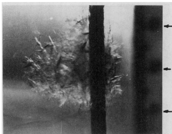
FIG. 7. A large cluster of ice crystals, which is fused to the metal support of the thermocouples at the level of the overcooled zone, 1–2 cm up from the middle of the density interface. The density interface is partly visible as a wavy shadow below the cluster. The scale is marked to the right, with distance between the marks indicating 1 cm.
