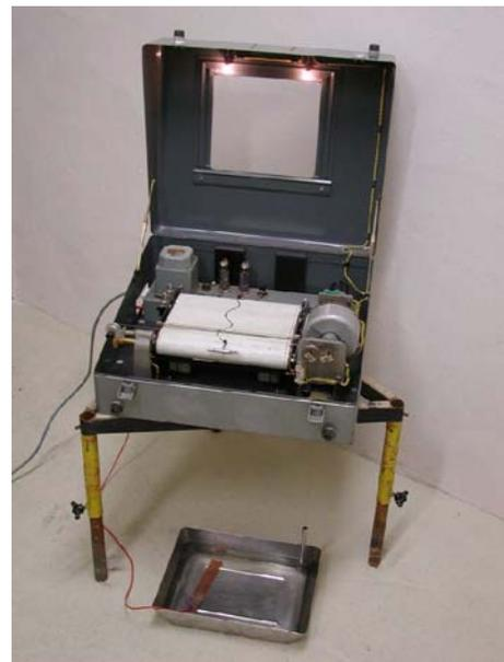
**Fig. 2** The experimental tide gauge used on the Coriolis rotating tank
