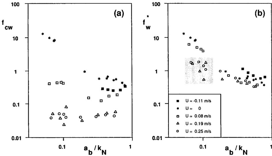
Fig. 1. Friction factors as recalculated from the data of Kemp and Simons (1982, 1983) and Simons et al. (1988). (a)  $f_{cw}$  of the integral approach; (b)  $f_w^*$  of the separate approach. The shaded area in (b) shows results of Simons et al. for  $T_a=0.7$  s and  $U > 0.08$  m/s.
