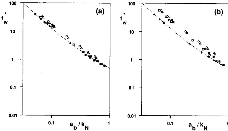
Fig. 2. Friction factors of the separate approach for the experimental conditions of Kemp and Simons (1982, 1983) and Simons et al. (1988) as predicted by (a) the model of Grant and Madsen, 1979, (Christoffersen, 1982) and by (b) Jonsson's (1966b) interpolation formula (15). Symbols as in Fig. 1; dotted line = Eq. 14 (no currents).
