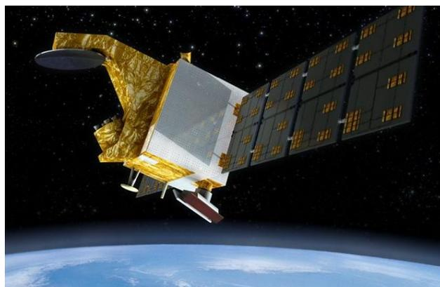
**Figure 1. Artist view of the CFOSAT satellite. SWIM antenna is on the left and SCAT antenna on the bottom right. Other antennas on Earth face are for TM/TC. © CNES/ Gekko.**
