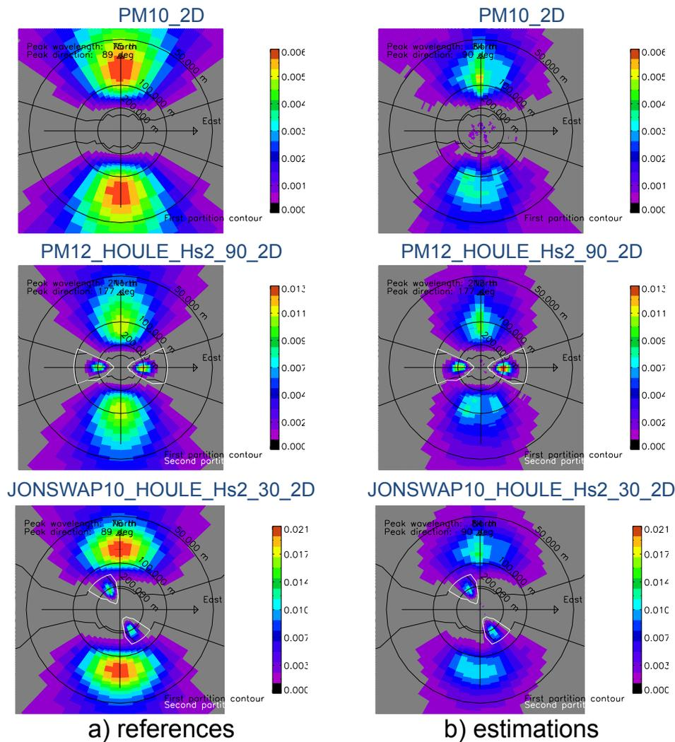
**Figure 3.** Examples of wave spectra simulations (1st column = references coming from analytical models, 2nd column = SWIM simulations) for three sea state conditions (wind sea Pearson-Moskowitz (PM) and mixed sea swell/wind sea with PM and JONSWAP). The spectra are in polar coordinate and they are automatically partitioned (black and white lines).
