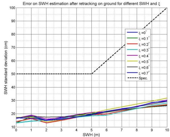
**Figure 2. Expected error (standard deviation) on the SWH as a function of SWH (from 0m to 9m) and to the mispointing  $\xi$  (from 0° to 0.7°, different color, see insert).**
