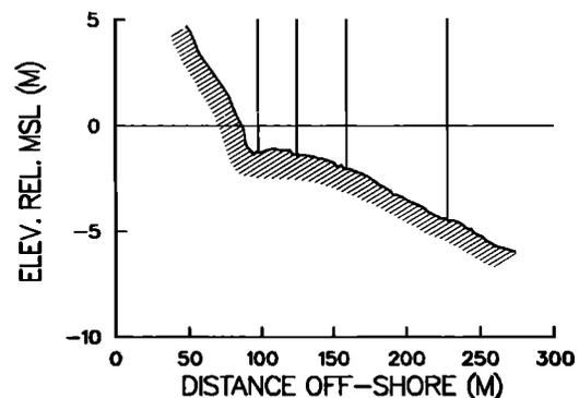
Fig. 9. Beach profile at Soldiers Beach, California on August 24, 1981. Vertical lines indicate measurement locations.
