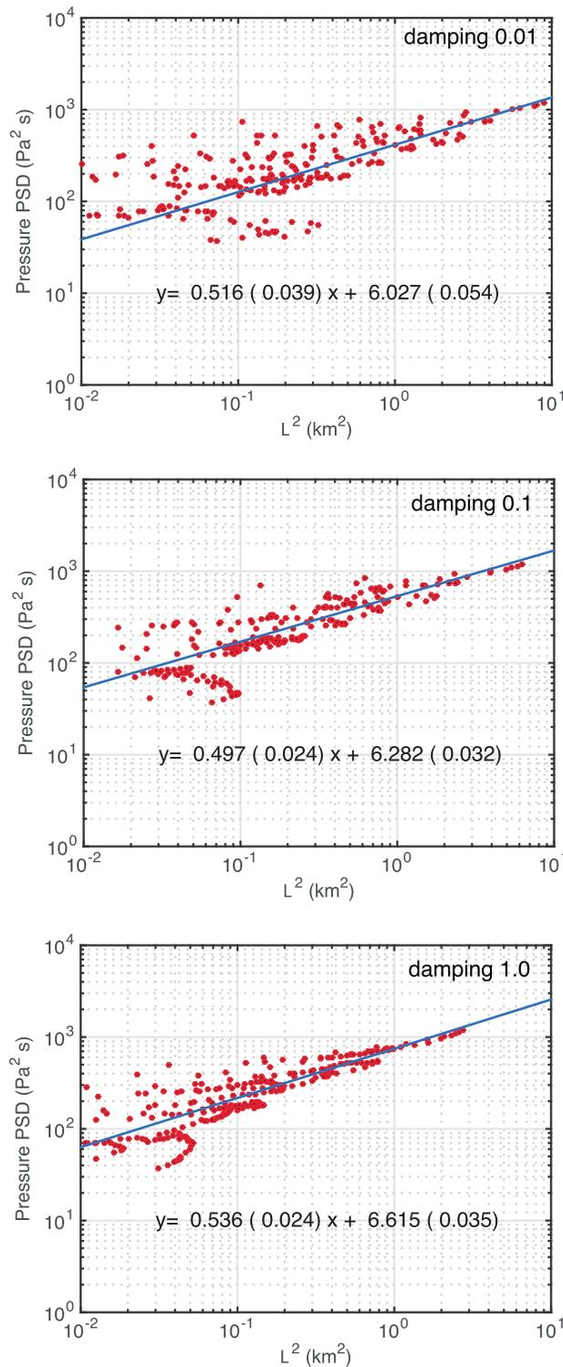
**Figure 12.** Plot of the correlation lengths versus the pressure PSD for three different cases of damping parameters. (top to bottom) The damping parameter was varied by a factor of 100 (0.01-0.1-1.0). Lines are the least squares fit to data. The main point of this figure is the relatively stable coefficient of about 0.5 in the least squares formula. In this formula,  $y$  is the logarithm of pressure and  $x$  is the logarithm of  $L^2$ .
