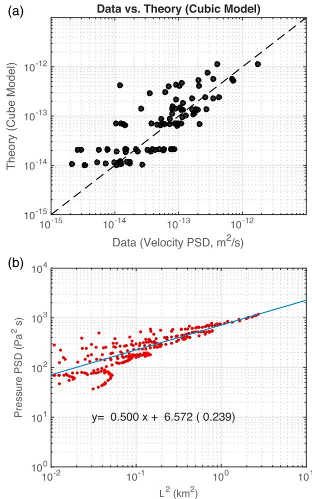
**Figure 13.** (a) Comparison between theory and data for the cubic model. There are some scatters but the cubic model seems to explain the overall trend in data. (b) The cubic model was rederived by fitting the data (same data with Figure 12, bottom) by fixing the gradient as 0.5. This means that there is a relation between the correlation length and pressure PSD as  $L = (1/714.8)S_p$  (see text).
