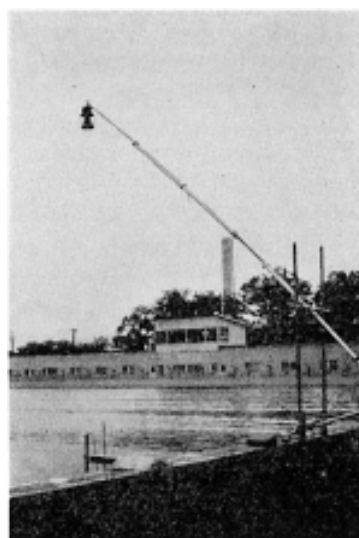
Fig. 4. Arrangement of wave sensors in the tank test.
