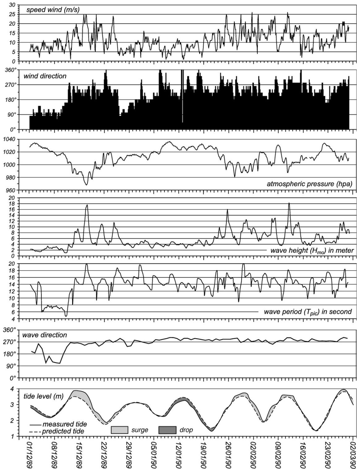
**Fig. 5.** Meteorological and oceanic characteristics (wave, wind, pressure and surge) recorded during the 1989–1990 winter storms. Wave data obtained from measurements by buoy BEAIII off Ouessant Island (lat. 48°30'; long. 5°45'; 110 m depth), wind and pressure data obtained from meteorological station *Météo France* of Ouessant Island (Stiff lighthouse), tide data obtained from the tide gauge station of Le Conquet (SHOM – lat. 48°21'; long. 4°46').
