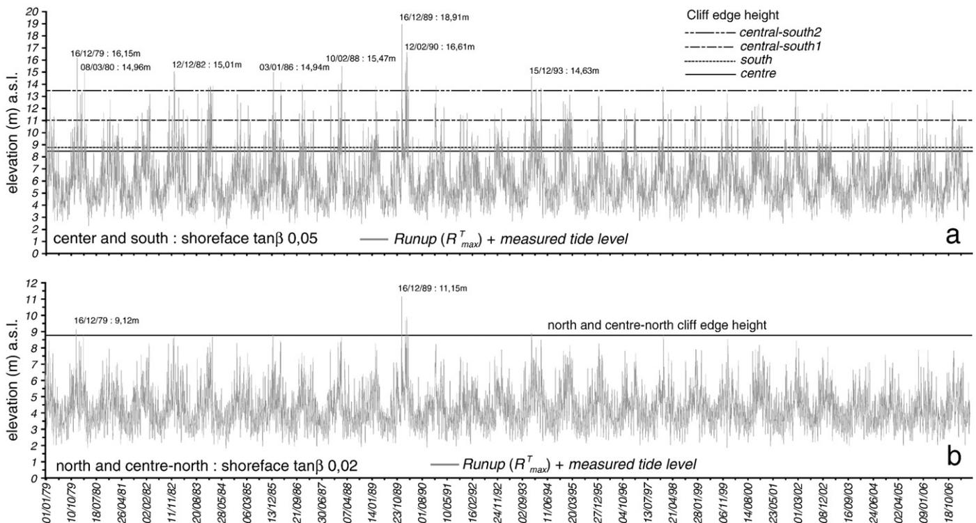
Fig. 13. Heights of extreme water levels (measured tide and runup) compared to sea-cliff heights from January 1st 1979 and June 7th 2007.
