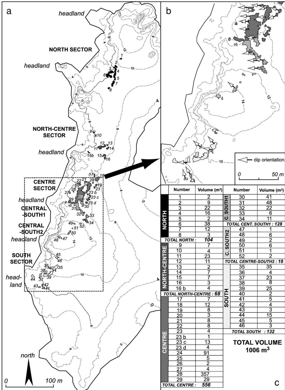
Fig. 7. Characteristics of clast deposits on Banneg Island. a) Location. b) Wave direction based on dip measurements. c) Volume of clast accumulations.
