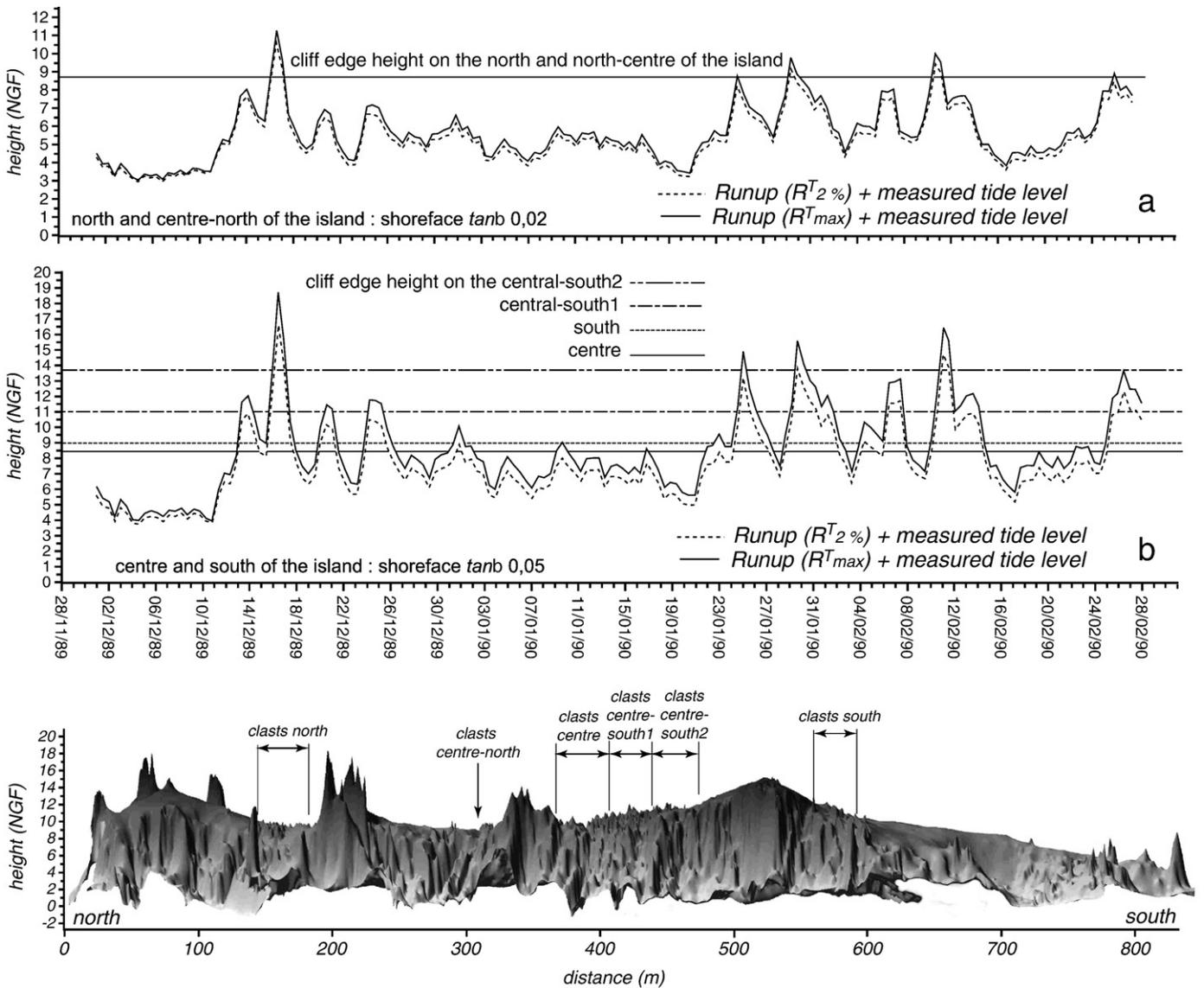
Fig. 11. Heights of extreme water levels (measured tide and runup) compared to sea-cliff heights during the 1989–1990 winter storms.
