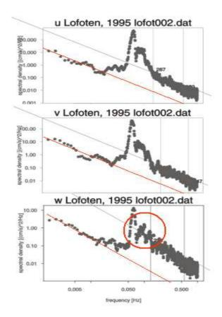
Figure 6. Example of energy spectra for the three velocity components. The red ring circles the range where the wind waves are damped out in the vertical component, due to the instrument depth of about 20 m. Note that the Y-axis scale of the figures are not equal.
