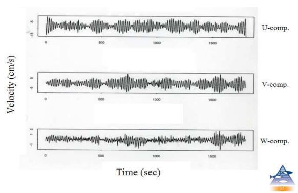
Figure 5. Example of a 20-minute time series for the three velocity components.
