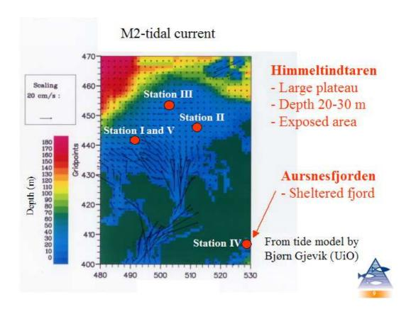
Figure 1. Overview of the investigation area. Colours indicate the depths at the location, arrows is the  $M_2$  modelled tidal current (courtesy of Bjørn Gjevik, University of Oslo, Norway). Red dots are the different stations where the tower was used. Note that station IV is at the end of a south-facing fjord.
