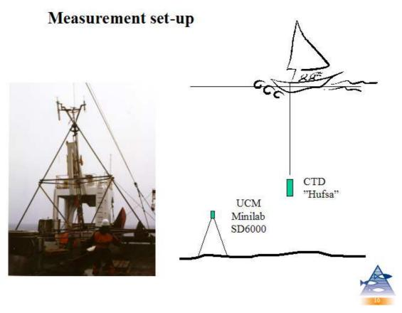
Figure 2. The left-hand picture shows the underwater tower before deployment (please note that the white structure in the background is a crane on the ship, and not part of the tower). The right-hand drawing is a sketch of the set-up.
