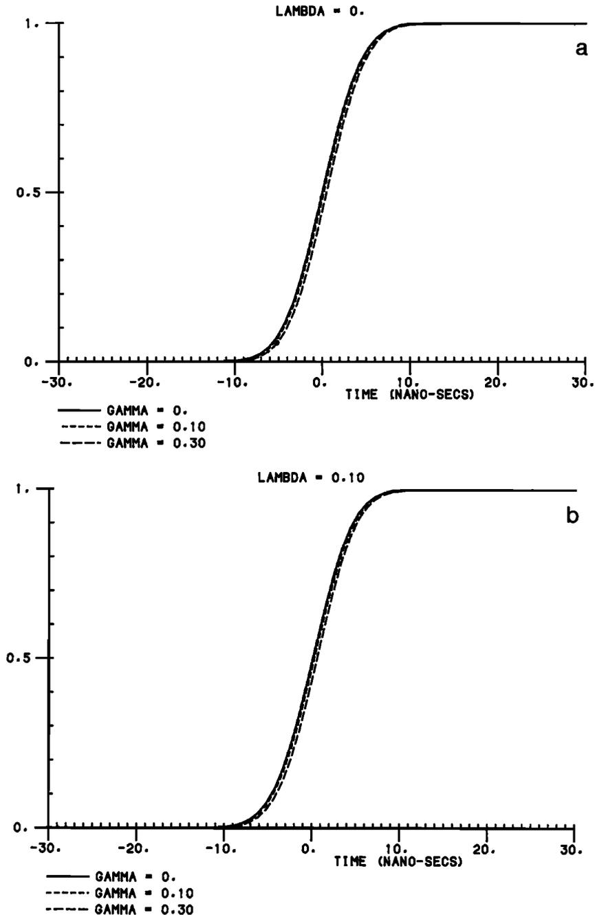
Fig. 3. Return pulse  $\sigma(t)$  for  $H_s = 2$  m and (a)  $\lambda_{300} = 0$ , (b)  $\lambda_{300} = 0.1$ , (c)  $\lambda_{300} = 0.3$ ; with (solid curve)  $\gamma = 0$ , (short-dashed curve)  $\gamma = 0.1$ , and (long-dashed curve)  $\gamma = 0.3$ .
