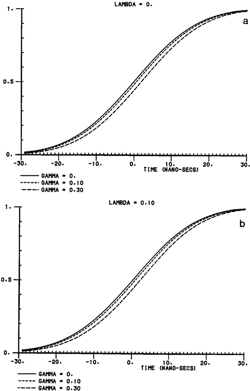
Fig. 4. Return pulse  $\sigma(t)$  for  $H_s = 8$  m and (a)  $\lambda_{300} = 0$ , (b)  $\lambda_{300} = 0.1$ , (c)  $\lambda_{300} = 0.3$ ; with (solid curve)  $\gamma = 0$ , (short-dashed curve)  $\gamma = 0.1$ , and (long-dashed curve)  $\gamma = 0.3$ .
