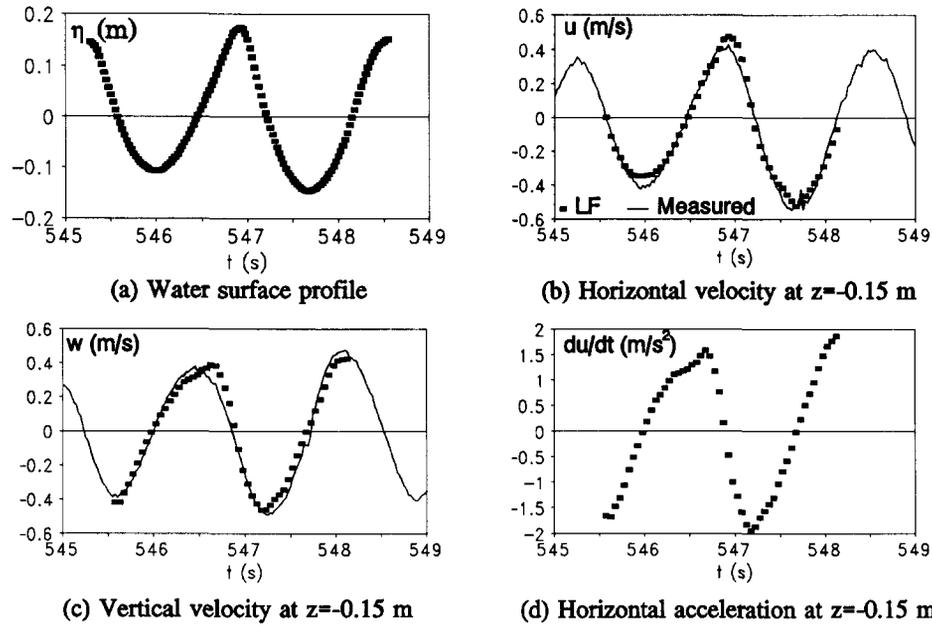
Fig. 6. Measured kinematics and LF predictions for a laboratory wave of Tørum and Skjelbreia.<sup>17</sup>
