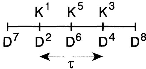
Fig. 1. Distribution of points and free surface boundary conditions within local window.
