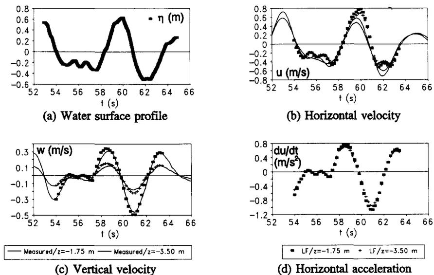
Fig. 7. Measured kinematics and LF predictions for a laboratory wave in Delft Hydraulics Delta Flume (1984).
