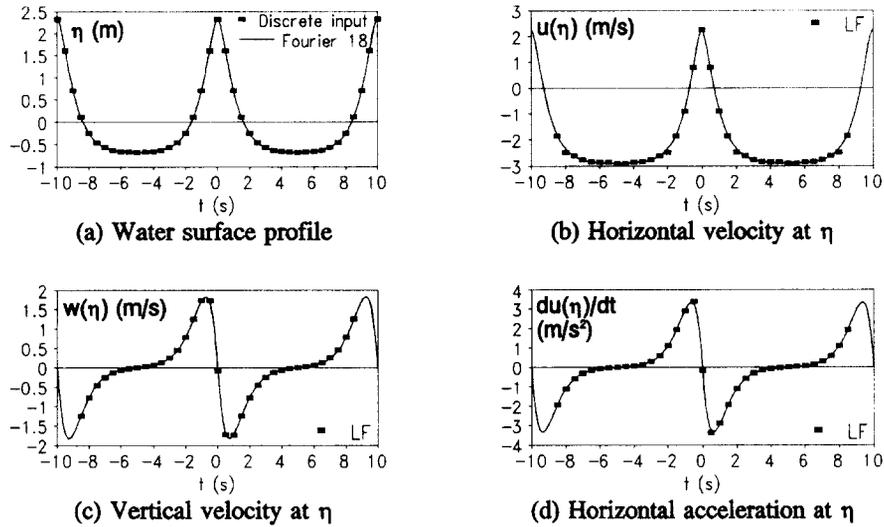
Fig. 4. Theoretical kinematics and LF predictions for the shallow-water regular wave.
