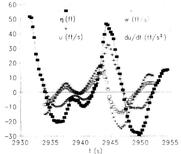
Fig. 8. LF predictions for a measured wave during Hurricane Camille (1969).
