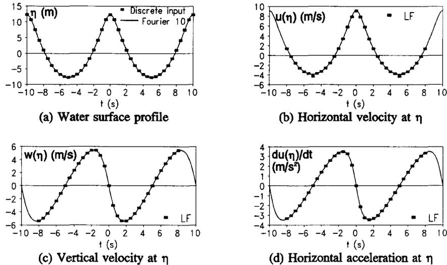
Fig. 2. Theoretical kinematics and LF predictions for the deep-water regular wave.
