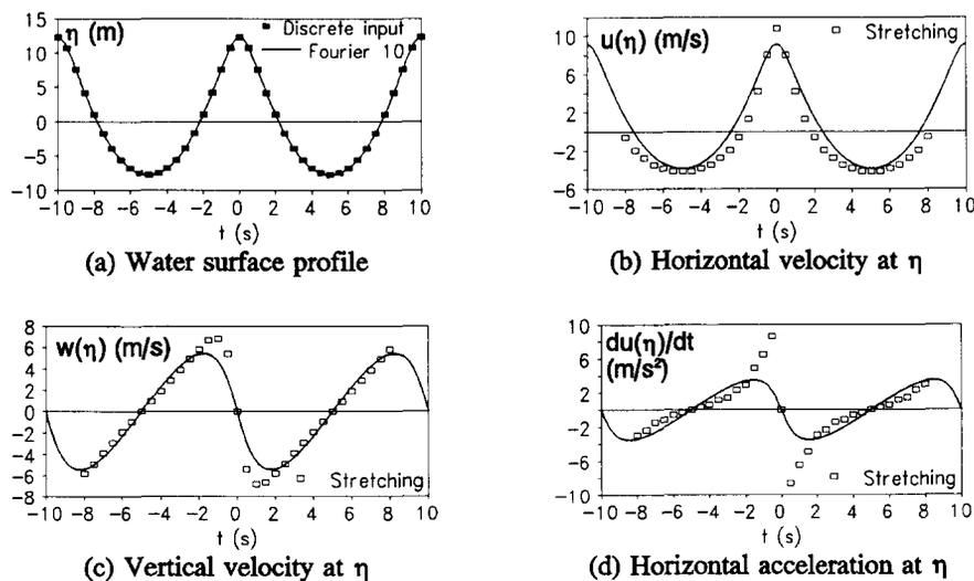
Fig. 3. Theoretical kinematics and Wheeler stretching predictions for the deep-water regular wave.
