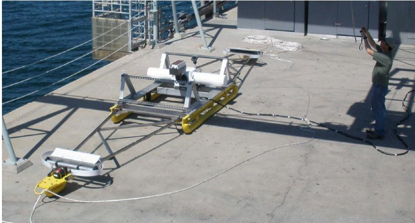
FIG. 5. The BiPADS and sled being prepared for deployment off the Scripps Pier by lead engineer Mike Goldin. The arms fold up vertically for deployment and then are lowered to a horizontal position on the sea floor, placing the transmitters 3.8 m to either side of the receiver array (small brown rectangle in the center).
