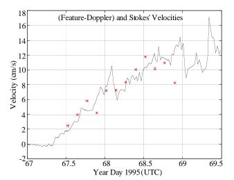
**Figure 5.** Comparison of feature-tracking velocities minus Doppler velocities from the sector-scan sonar data (stars) versus Stokes' drift (solid line). Stokes' drift is calculated by linear theory from directional wave-wire data. Only the along-axis component is compared. For this component the net feature–Doppler velocity difference matches the calculated Stokes' drift.
