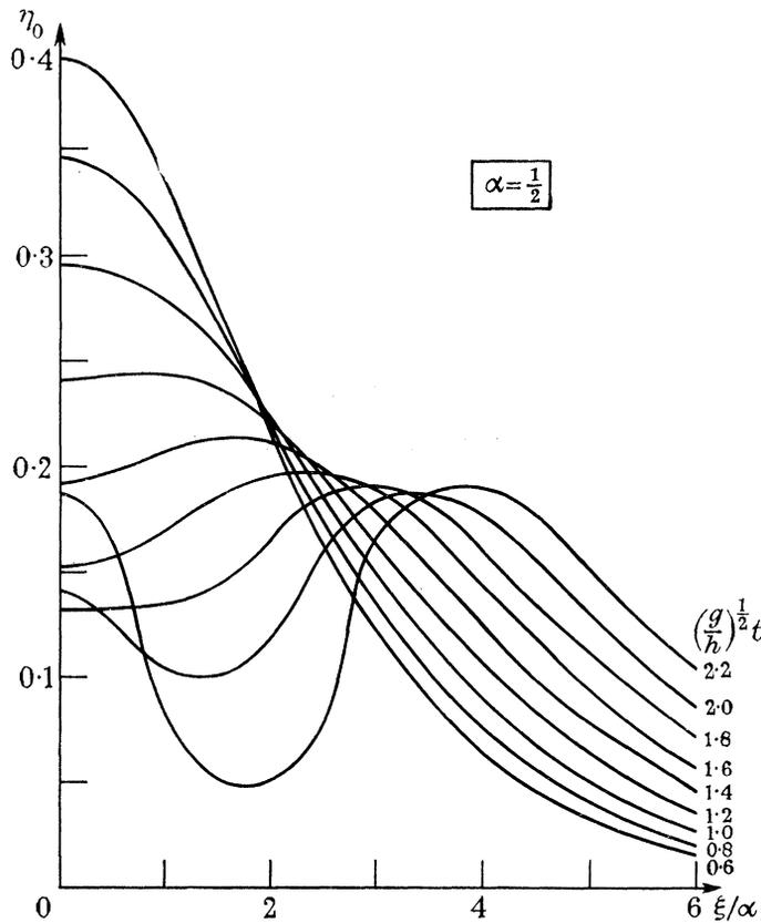
FIGURE 9. Development of first wave (incompressible fluid).
