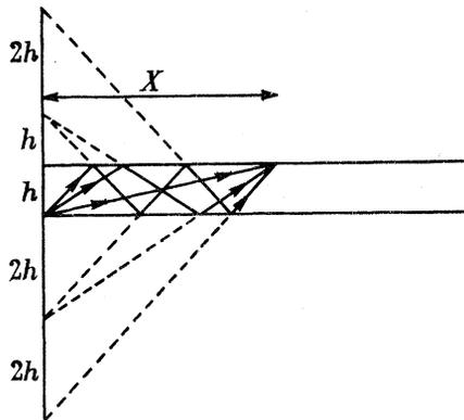
FIGURE 3. The image system for reflected arrivals.
