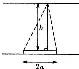
FIGURE 6. Direct arrival paths at point over the block.
