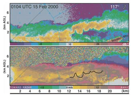
Fig. 9. RHIs from the Doppler on Wheels (DOW2) at  $0104~\rm UTC~15~\rm Feb~2000$  along the  $117^{\circ}$  azimuth: (a) radar reflectivity factor (dBZ); (b) radial velocity (m s<sup>-1</sup>). Solid black line in (b) represents approximate outline of mammatus in (a).
