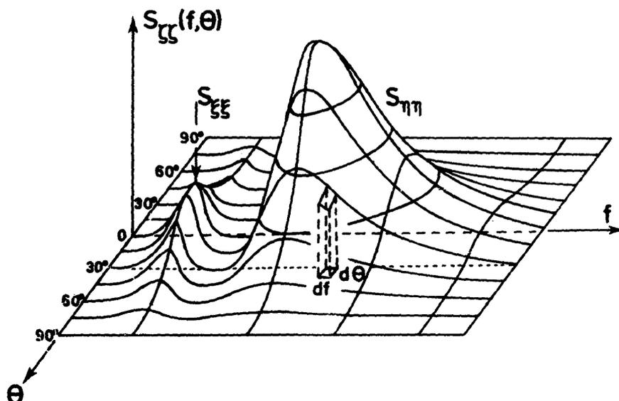
Fig. 8. Directional spectrum consisting of a short- and a long-wave part.
