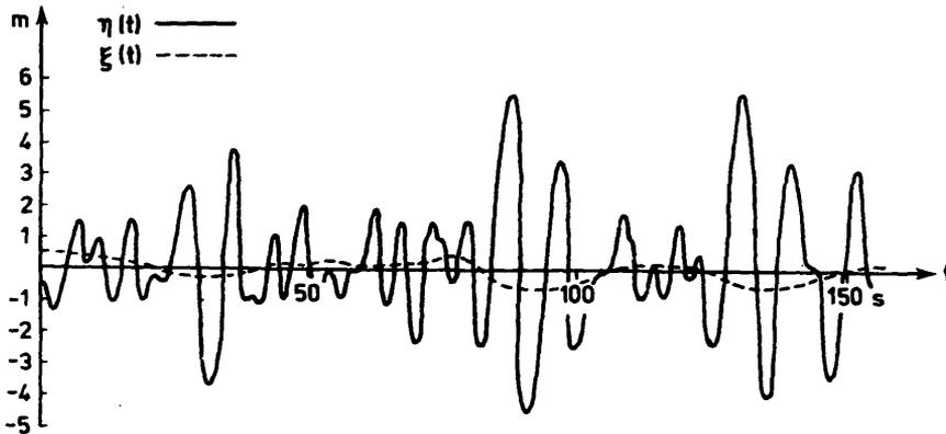
Fig. 1. Short- and long-wave measurements in the North Sea. The significant wave height was 6.5 m and the water depth 40 m. The long waves have been doubled for clearness.
