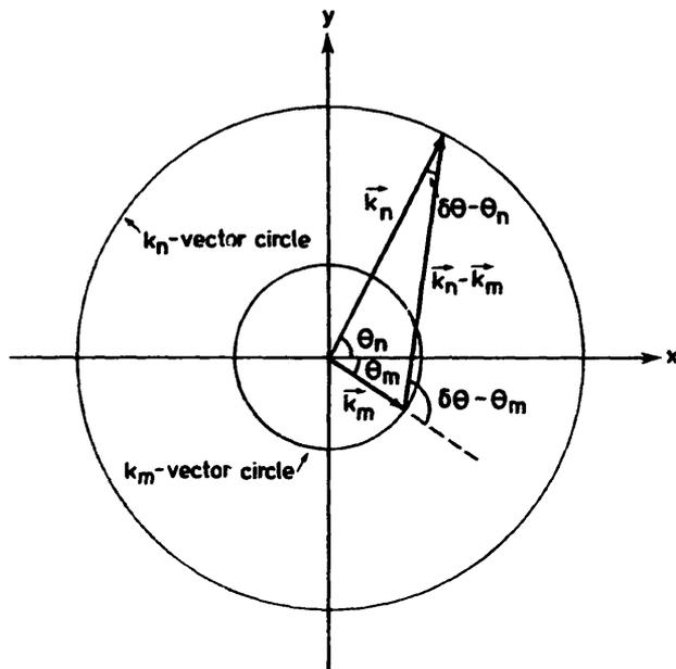
Fig. 3. Wave number vectors  $\vec{k}_n$ ,  $\vec{k}_m$  of two short-wave components, and the resulting long-wave vector  $\vec{k}_n - \vec{k}_m$ . The associated angles of travel are used for directional spectrum calculations.
