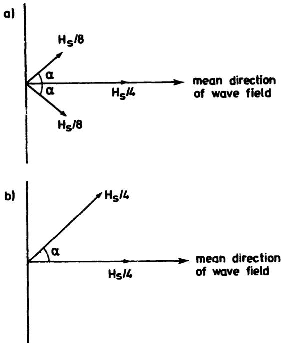
Fig. 6. a. Directional distribution approximated by three wave components. b. Equivalent distribution as regards long-wave amplitudes.
