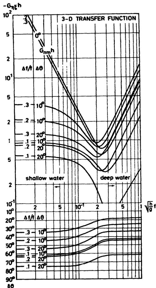
Fig. 4. The directional transfer function  $G_{\eta\xi}$  for a wave group consisting of two frequencies  $f_m = f$  and  $f_n = f + \Delta f$  with angle  $\Delta\theta$  between one another. Lower part indicates long wave direction of travel,  $\delta\theta$ , for short waves with  $\theta_n = -\theta_m$ .
