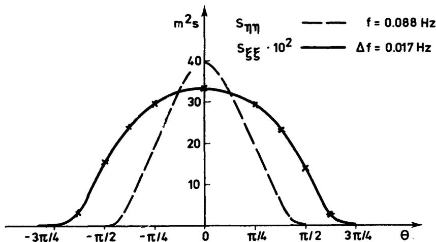
Fig. 5. A  $\cos^2\theta$  distribution applied to a North Sea wave spectrum with peak frequency  $f_p = 0.088$  Hz. The resulting long-wave spread is shown for the components with  $\Delta f = 0.017$  Hz.
