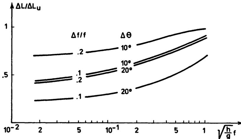
Fig. 7. Wave lengths,  $\Delta L$ , of directional long waves to wave lengths,  $\Delta L_u$ , of uni-directional long waves shown as function of a dimensionless frequency.
