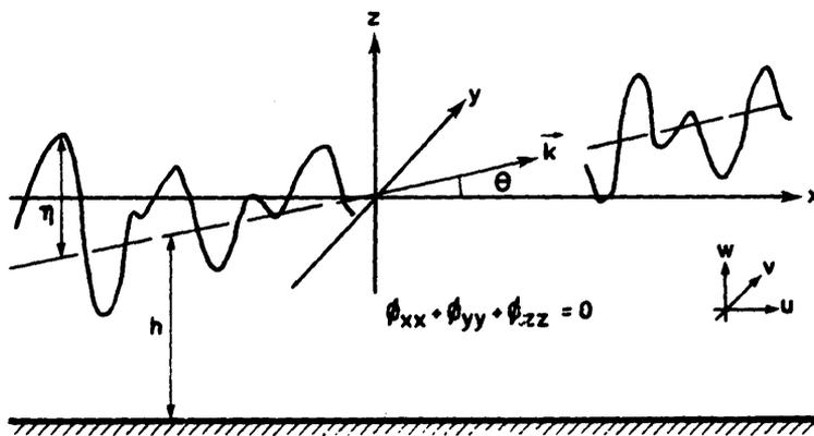
Fig. 2. Definition sketch showing a wave train with wave number  $\vec{k}$  in direction  $\theta$ .
