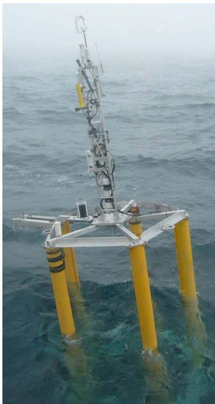
**Figure 1.** Photograph of the ASIS buoy taken on 10 March 2008 (YD 70), shortly after deployment from the R/V *Ronald Brown*. For reference the mast is 2.4 m high. Photo taken by David Ho.
