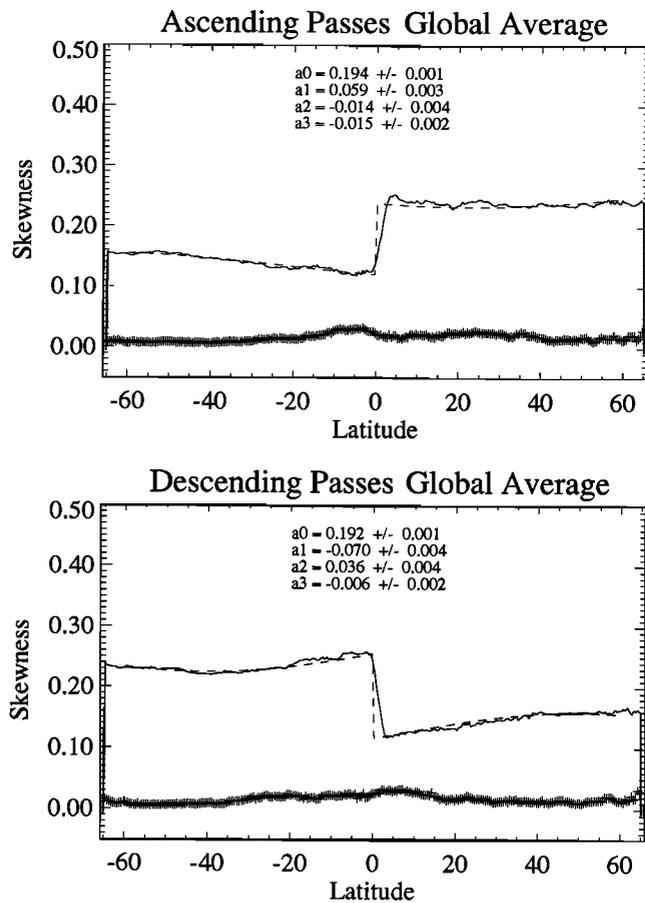
**Figure 7.** Mean (solid curve) and standard deviation (pluses) of latitudinal average of C band skewness estimates for (top) ascending and (bottom) descending passes. Dashed curves show fits as in Figure 5.
