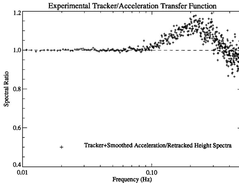
**Figure 4.** The ratio of the spectrum of the GDR height correction with the acceleration correction smoothed by a 5-s Hanning window to the spectrum of the retracked height correction. Result is similar to Figure 3b with no acceleration correction but shows decrease in ratio for frequencies less than 0.2 Hz.
