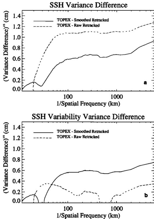
**Figure 15.** (a) Integral of height variance reduction spectrum for raw retracted data (dashed curve) and smoothed retracted data (solid curve). (b) Same as Figure 15a, but variability spectra instead of absolute height spectra. Note the consistency with results of Figures 13 and 14.
