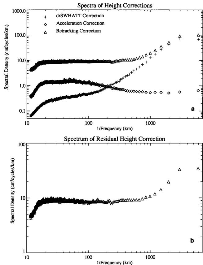
**Figure 12.** (a) Spectra of GDR SWH attitude, acceleration, and retracked height corrections versus inverse spatial frequency. (b) Spectrum of difference of total GDR correction and retracked spectrum.
