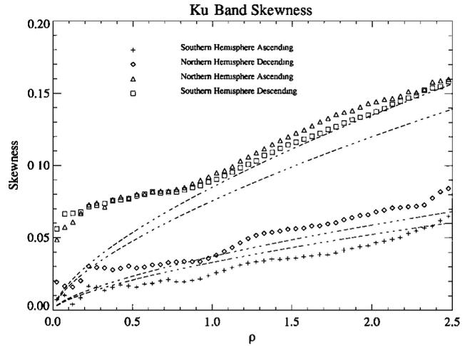
**Figure 6.** Ku band skewness estimates separated by north/south and ascending/descending and binned by parameter  $\rho$ . Theoretical bounds on expected skewness for a power law ocean with  $p = 4$  (long-dashed curve) and  $p = 3.5$  (short-dashed curve) are also shown. Note the relative consistency of the pre- and postequator parts of each pass. Though the absolute values of the skewness are just barely consistent with theory, the form of the  $\rho$  dependence is consistent.
