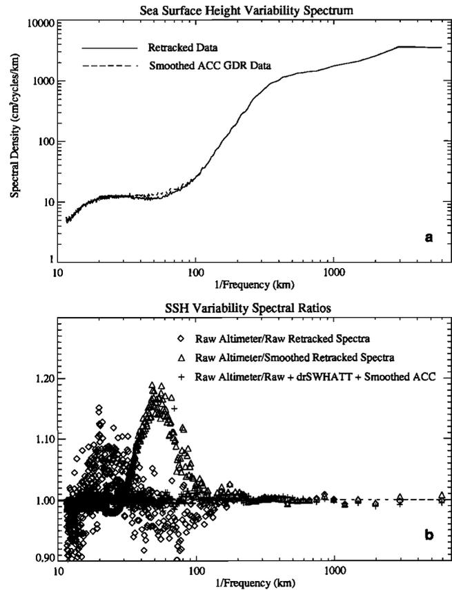
**Figure 14.** (a) Spectra of difference between retracked (solid curve) or GDR (dashed curve) sea surface height estimates and the mean height values at that position (variability spectrum). (b) Ratios of raw (uncorrected) altimeter height spectrum to raw retracked (diamonds), smoothed retracked (triangles), and GDR (pluses) height variability spectra. The greatest reduction in variability variance is achieved with the smoothed retracked data.
