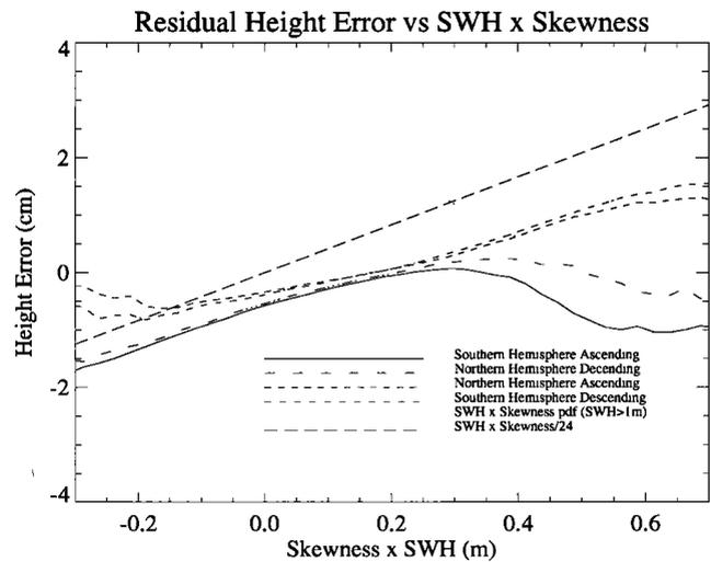
**Figure 10.** Comparison of height residuals with theoretical skewness bias of  $\lambda H_{1/3}$ . The change in the slope of the curves is due to a change in the tracking gate size, as discussed by Rodríguez [1988].
