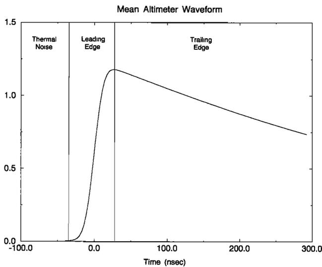
**Figure 1.** A typical altimeter waveform generated using the triple-convolution theory and TOPEX point target response approximated by 127 Gaussians. Other parameters are also consistent with TOPEX values.
