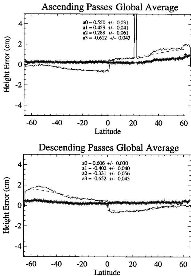
**Figure 11.** C band height correction residuals and standard deviations including acceleration correction for (top) ascending and (bottom) descending passes. Errors show peak-to-peak variation of 2 cm and jump of 1 cm at the equator. Anomalous value at 22° is due to a single point and may be ignored. Symbols are same as in Figure 7.
