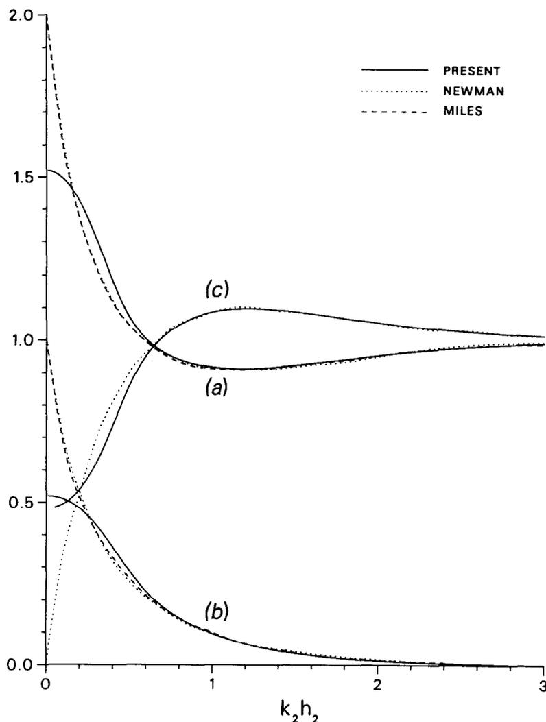
Fig. 2. First-order transmission and reflection coefficients for  $h_2/h_1 = 1/10$  (—), compared with Newman [4] (···) and Miles [5] (- - -): (a)  $|T_1|$  and (b)  $|R_1| (= |R_2|)$ . (c) is  $|T_2|$  for the case where an incident wave arrives from the shallow side with  $h_2/h_1 = 10/1$ .
