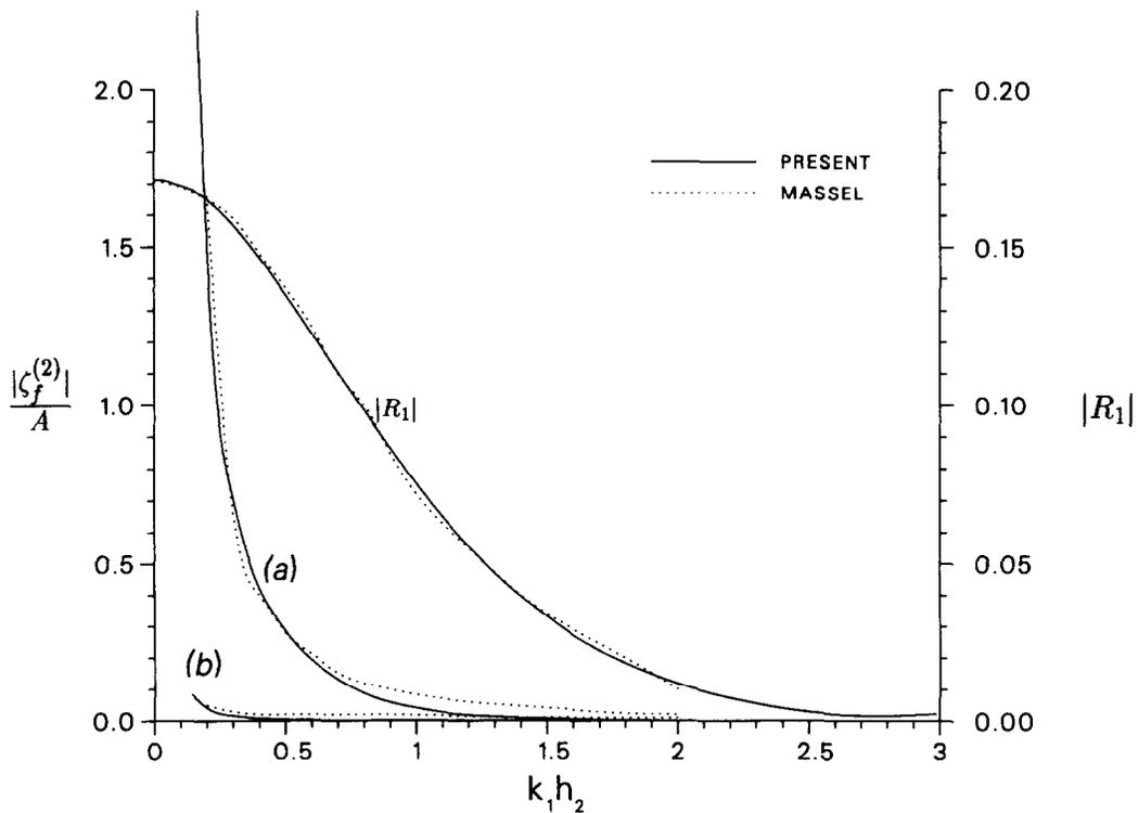
**Fig. 4.** Second-order free-wave amplitudes for  $h_2/h_1 = 1/2$ ,  $A/h_2 = 0.134$  and  $A = 0.134$  (—), compared with Massel[18] (···) on normal incidence ( $\theta = 0$ ): (a) at  $x = +\infty$  defined by eqn (45) and (b) at  $x = -\infty$  defined by eqn (44). Also shown is the comparison for first-order reflection coefficients  $|R_1|$ . Note that the parameter  $k_1 h_2$  is the same as  $kh_1$  in Massel's Fig. 6.
