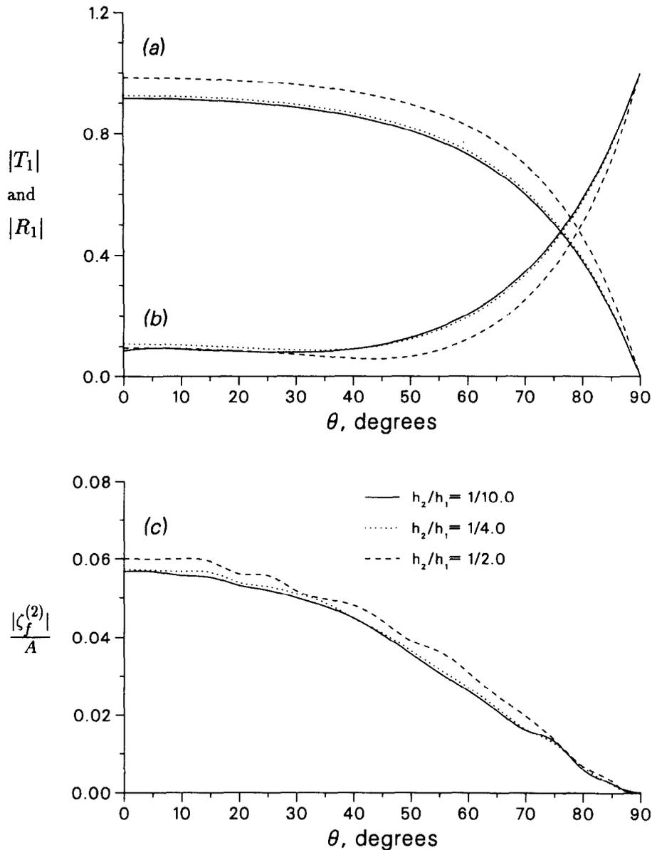
Fig. 5. Result for an oblique wave incident from  $x = -\infty$  ( $\theta = 0$  for normal incidence) with  $h_2/h_1 = 1/10$  (—),  $h_2/h_1 = 1/4$  (⋯) and  $h_2/h_1 = 1/2$  (- - -) ( $k_2h_2 = 1.0$ ,  $A/h_2 = 0.1$ ): (a) at the first-order transmission coefficient  $|T_1|$ , (b) the first-order reflection coefficient  $|R_1|$ , and (c) the second-order free wave at  $x = +\infty$  defined by eqn (45).
