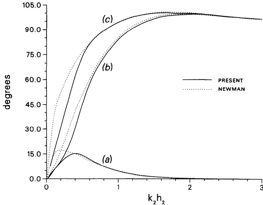
**Fig. 3.** Phase shifts of the first-order transmission and reflection coefficients for  $h_2/h_1 = 1/10$  (—), compared with Newman[4] (···): (a)  $\delta T_1$  ( $= \delta T_2$ ), (b)  $-\delta R_1$ , and (c)  $(\pi + \delta R_2)$  for the case where an incident wave arrives from the shallow side with  $h_2/h_1 = 10/1$ .
