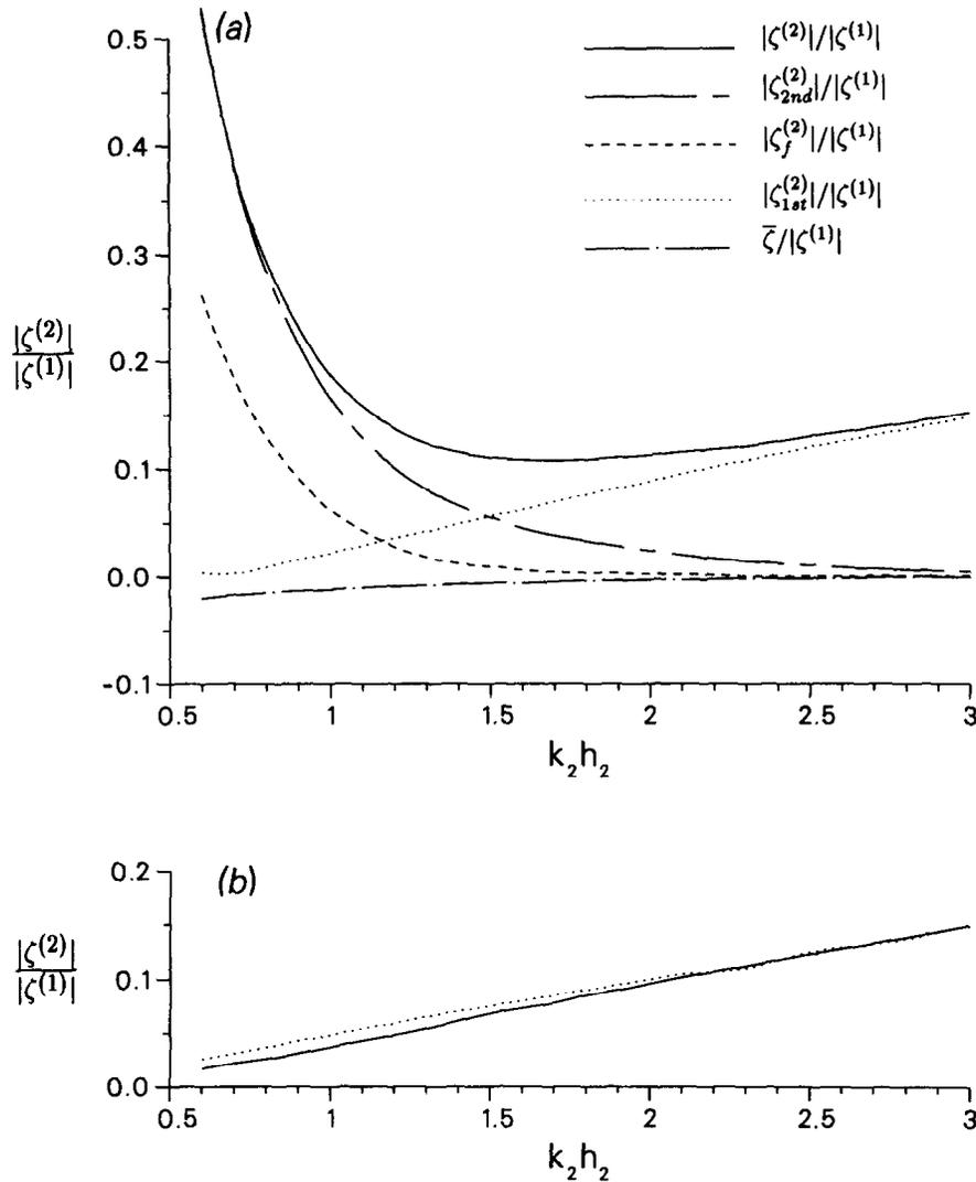
**Fig. 6.** Ratio of second- to first-order wave amplitude for normal incidence ( $\theta = 0$ ) with  $h_2/h_1 = 1/10$  and  $A/h_2 = 0.1$ , at (a)  $x = +\infty$  and (b)  $x = -\infty$ . (—)  $|\zeta^{(2)}|/|\zeta^{(1)}|$ ; (---)  $|\zeta_{2nd}^{(2)}|/|\zeta^{(1)}|$ ; (- - -)  $|\zeta_f^{(2)}|/|\zeta^{(1)}|$ ; (· · ·)  $|\zeta_{1st}^{(2)}|/|\zeta^{(1)}|$ ; (- · -)  $\bar{\zeta}/|\zeta^{(1)}|$ . Results are calculated from eqns (11)–(15) using the maximum amplitudes.
