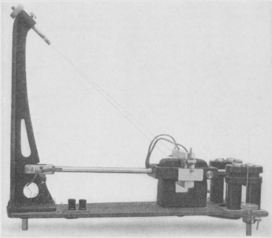
Fig. 5. Type of seismograph used: photographic side view.
