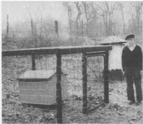
Fig. 10. Temporary housing of the microbarograph at Florissant. The instrument worked, for the most part, within the seismic vault.
