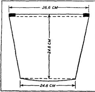
Fig. 6. Shape and dimensions of brass kettle.
