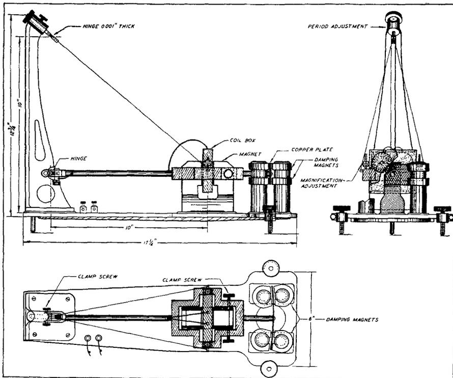
Fig. 4. Type of seismograph used, as seen from one side, one end, and from above.
