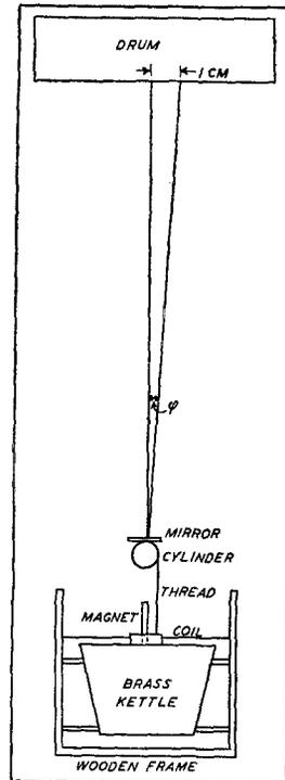
Fig. 7. Device for testing magnification.
