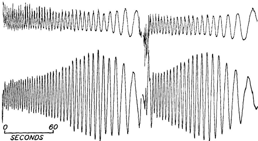
Fig. 8. Galvanometric magnification (bottom) and mechanical-optical magnification (top) when the microbarograph membrane was forced to vibrate with a slowly and evenly increasing period.
