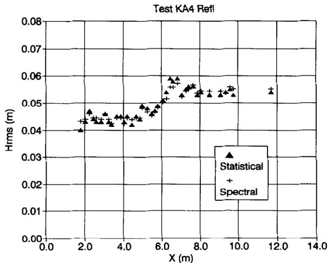
Fig. 14. Statistical and spectral wave height profiles (with reflection).
