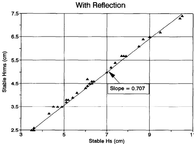
Fig. 16. rms stable wave height as a function of significant wave height (with reflection).
