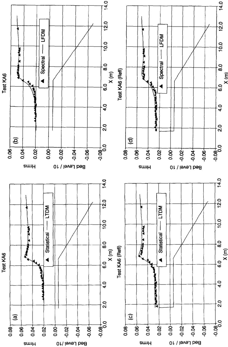
Fig. 20. (a) LFTDM for Test KA6 without reflection. (b) LFTDM for Test KA6 with reflection. (c) LFTDM for Test KA6 without reflection. (d) LFTDM for Test KA6 with reflection.
