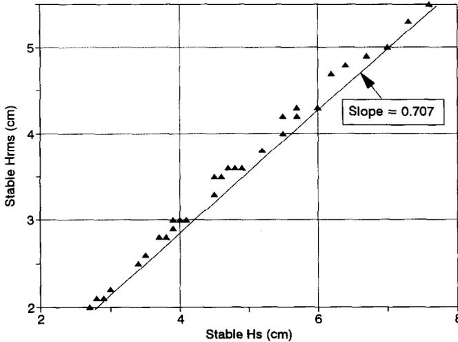
Fig. 8. rms stable wave height as a function of significant wave height.
