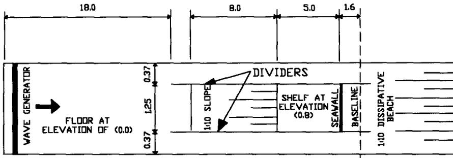
Fig. 3. Plan of 2 m wave flume (dimensions in meters).
