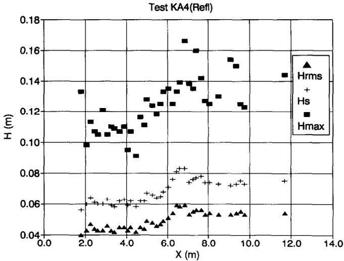
Fig. 15. Wave decay for different wave statistics (with reflection).
