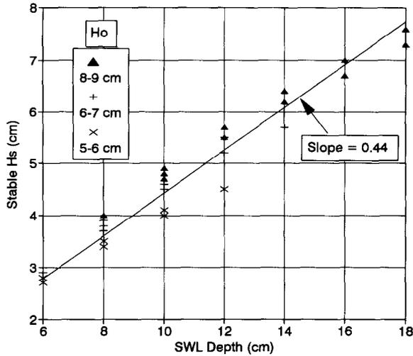
Fig. 6. Stable wave height as a function of SWL depth.
