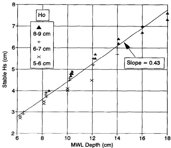
Fig. 7. Stable wave height as a function of MWL depth.
