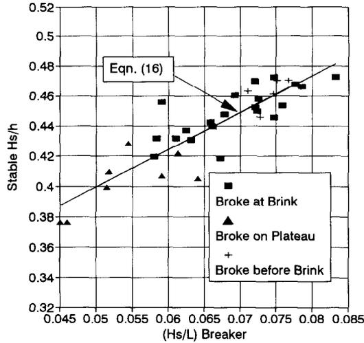
Fig. 11. Effect of breaker wave steepness on  $\Gamma_s$ .
