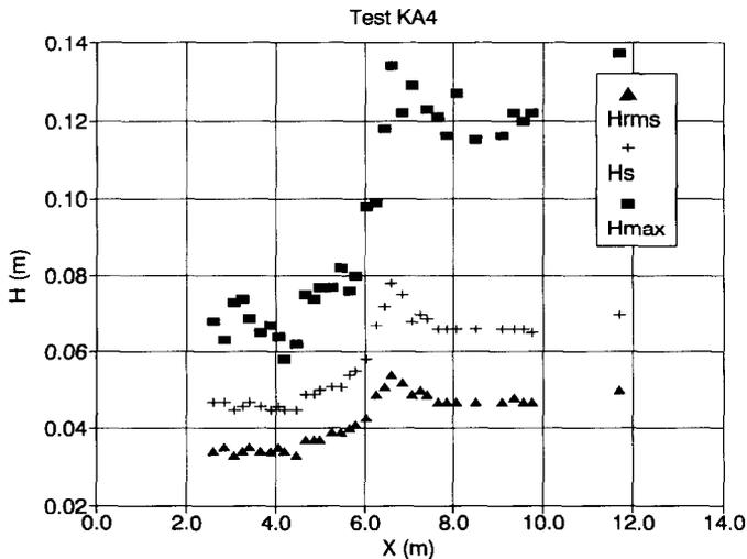
Fig. 5. Wave decay for different wave statistics.
