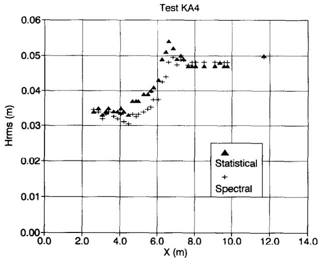
Fig. 4. Statistical and spectral wave height profiles.
