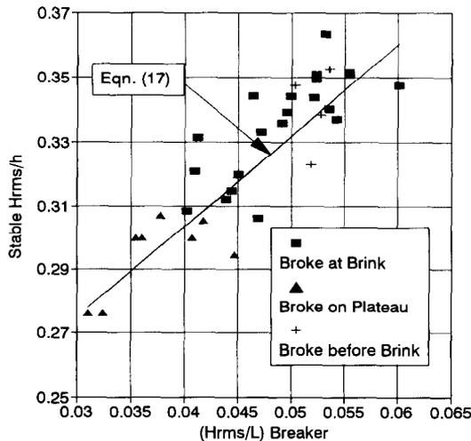
Fig. 12. Effect of breaker wave steepness on  $\Gamma_{rms}$ .
