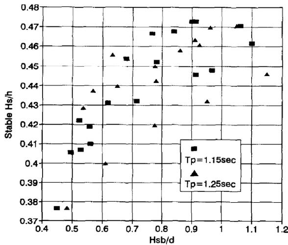
Fig. 10. Effect of breaker index and wave period on  $\Gamma$ .
