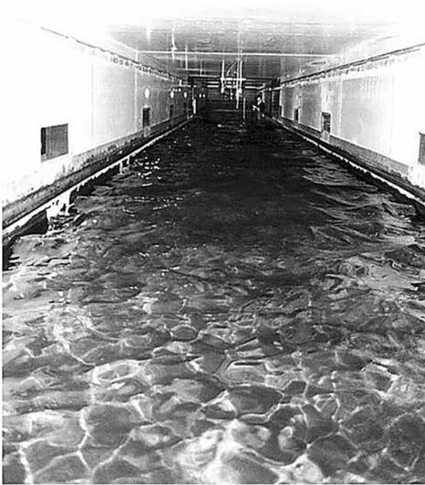
Figure 1. Inside of the wind-wave tank at Luminy, France. At the far end of the tank is the carriage holding the wind- and wave-monitoring equipment.
