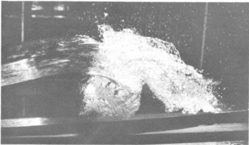
Figure 5 Wedge of clear water apparently pushed up by the plunging jet of a wave breaking from the left on a 1:35 beach. Photograph taken at ISVA, Technical University of Denmark. (The upper sloping black strip is a support for the flume.)
