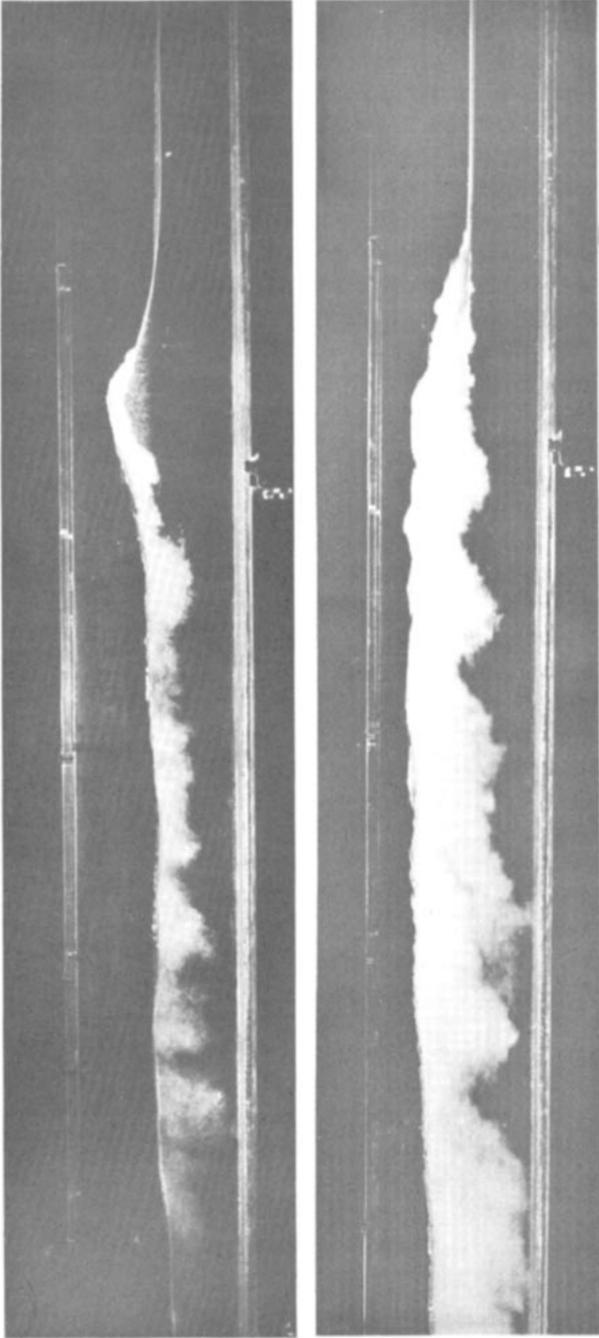
Figure 9 Flow visualization showing the approximate extent of turbulence behind (top) a spilling breaker and (bottom) a bore. Photographs courtesy of I. A. Svendsen, ISVA, Technical University of Denmark.
