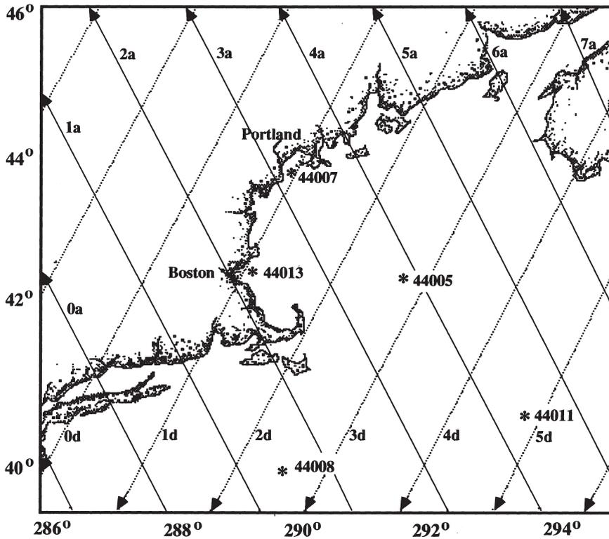
Fig. 1. Ascending and descending GEOSAT tracks in the Gulf of Maine. Asterisks show buoy locations.
