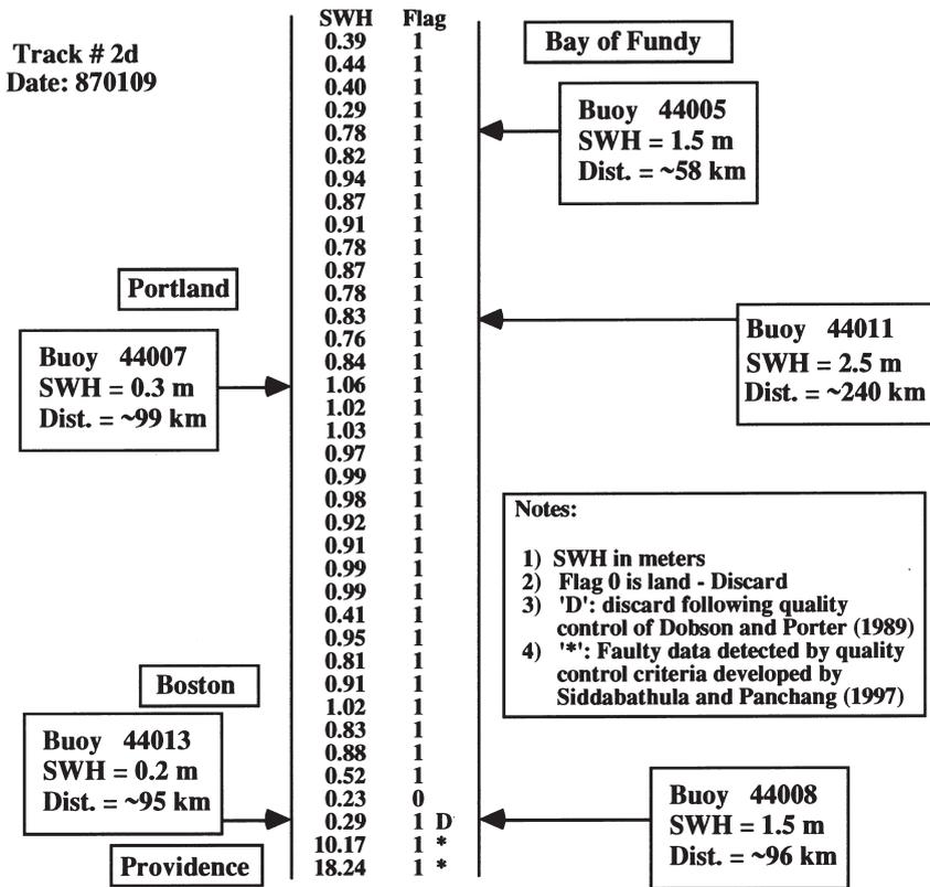
Fig. 2. Wave data in the Gulf of Maine for 9 January 1987. GEOSAT wave heights mostly at 1 second intervals. Buoy data at closest half-hour.
