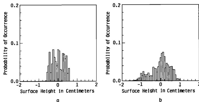
Fig. 8. First-year ice surface height histograms for a homogeneous ice sheet. (a) Data acquired June 14 are typical of early summer pre-melt, late fall, winter, and spring conditions. Height range, variance, and skewness were 0.932 cm, 0.044 cm<sup>2</sup>, and 0.0003, respectively. (b) Data acquired June 20 are typical of early summer melt conditions. Superimposed ice increased the height range to 2.778, the variance to 0.243, and skewness to -0.588.
