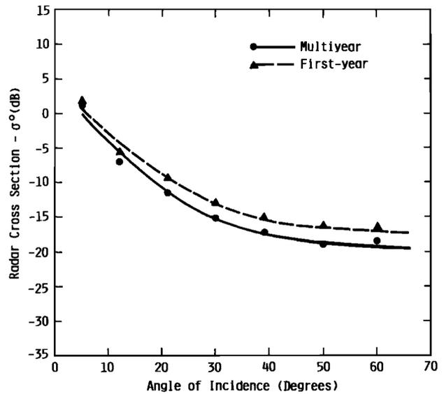
Fig. 3. Scattering coefficients of multiyear and first-year ice under summer melt conditions at 9.6 GHz and HH-polarization (June 19 and 22, 1982).
