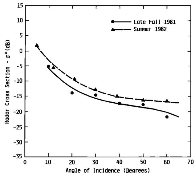
Fig. 7. Scattering coefficients of first-year ice under cold late fall and early summer melt conditions at 9.6 GHz and HH-polarization (October 1981 and June 19 and 22, 1982).
