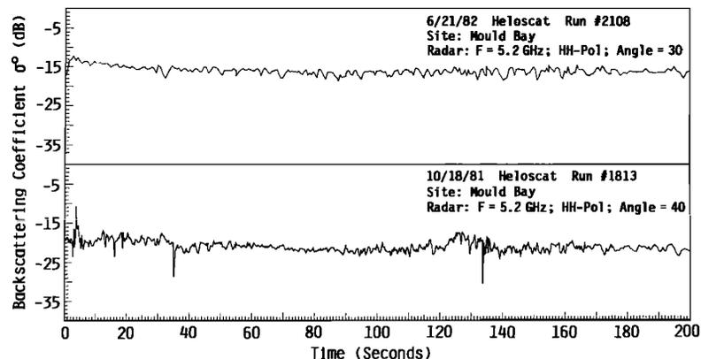
Fig. 9. Scattering cross-section profile of an 8-km line across the homogeneous first-year ice in Mould Bay acquired under late fall and early summer conditions at 5.2 GHz, HH-polarization, 30° and 40°.
