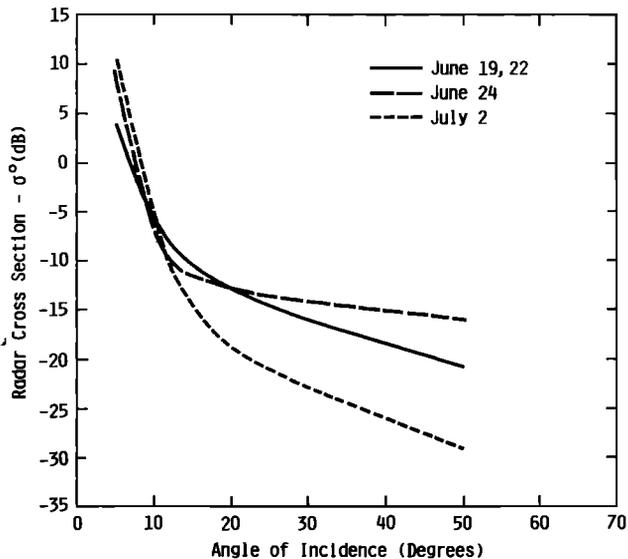
Fig. 10. Scattering coefficients of first-year ice during premelt, melt, and peak-melt conditions at 5.2 GHz and HH-polarization.
