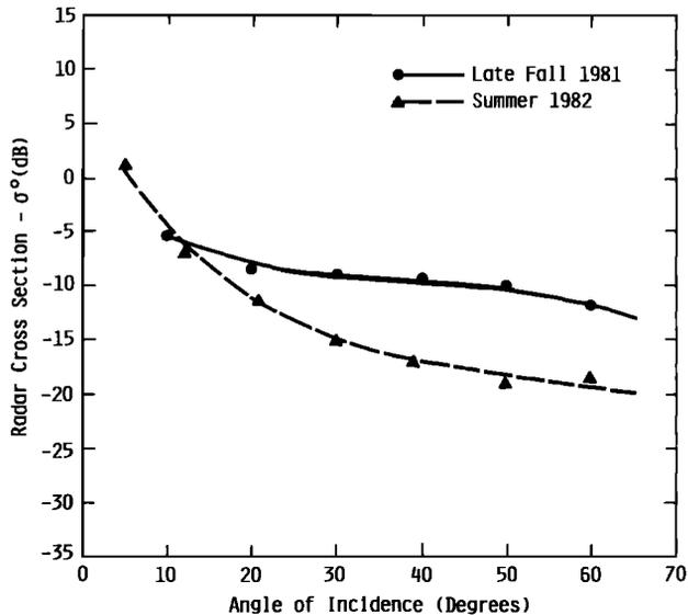
Fig. 6. Scattering coefficients of multiyear ice under cold late fall and early summer melt conditions at 9.6 GHz and HH-polarization (October 1981 and June 19 and 22, 1982).
