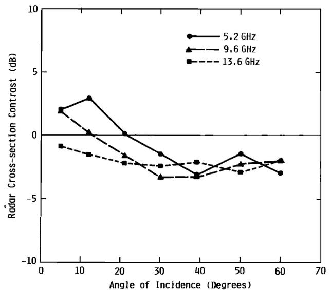
Fig. 5. Radar cross-section contrast between multiyear and first-year ice at 5.2, 9.6, and 13.6 GHz with HH-polarization for early summer melt conditions (June 19 and 22, 1982).
