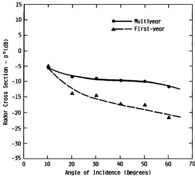
Fig. 2. Scattering coefficients of multiyear and first-year sea ice under cold late fall conditions at 9.6 GHz and HH-polarization (October 1981).
