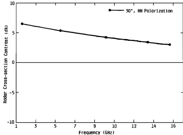
Fig. 11. Radar cross-section contrast between multiyear and first-year ice as a function of frequency for peak melt conditions (July 2).
