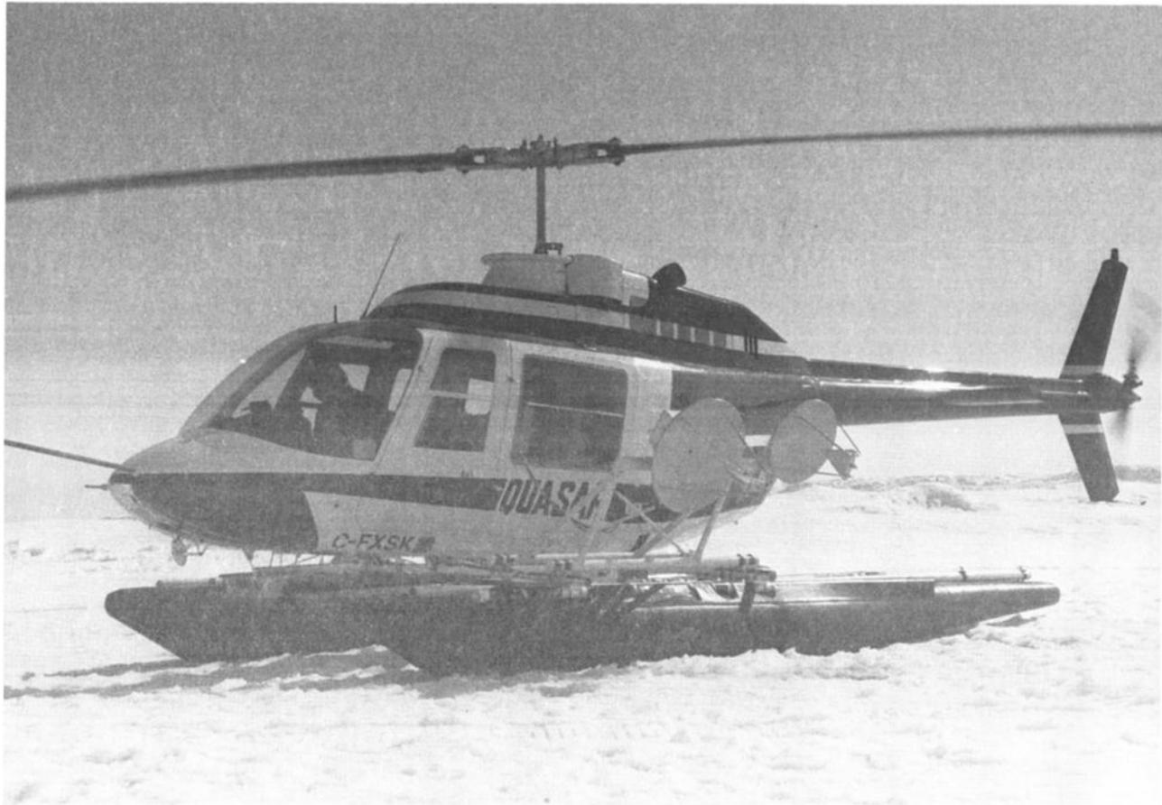
Fig. 1. University of Kansas helicopter-borne side-looking spectrometer/scatterometer.
