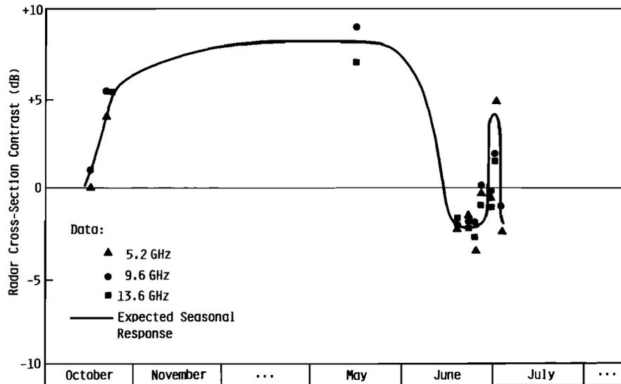
Fig. 4. Expected and measured radar cross-section contrast history for multiyear and first-year ice at 5.2, 9.6, and 13.6 GHz with HH-polarization and an angle of 30°.
