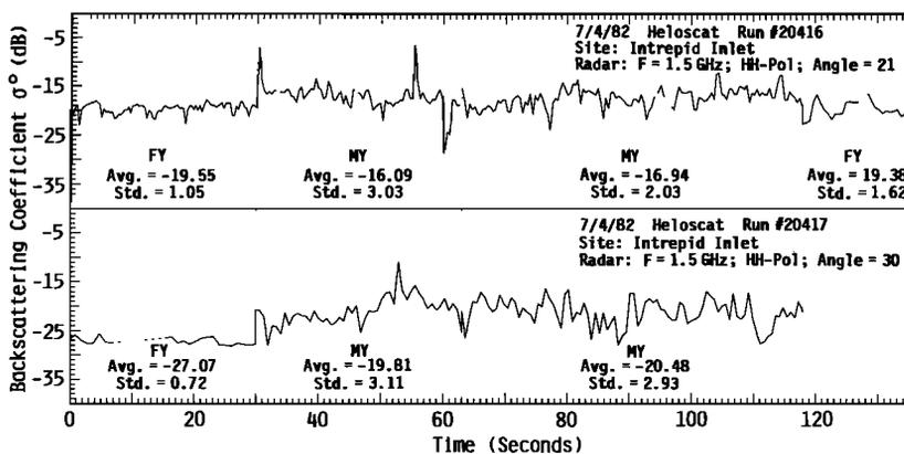
Fig. 12. Scattering cross-section profile across an old multiyear floe frozen in first-year ice in Intrepid Inlet. The radar parameters are 1.5 GHz, HH-polarization, 21° and 30° (July 4).
