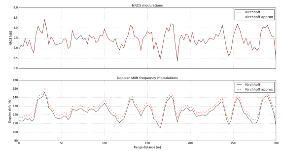
Fig. 4. Ka band NRCS and Doppler shift frequency range modulations versus range distance at a 12 degrees incidence radar. 8 m/s wind speed and 20 km long fetch Elfouhaily spectrum is considered. Solid curve is for Kirchhoff Assumption (KA) and dashed curves are for approximations (31) and (33)
