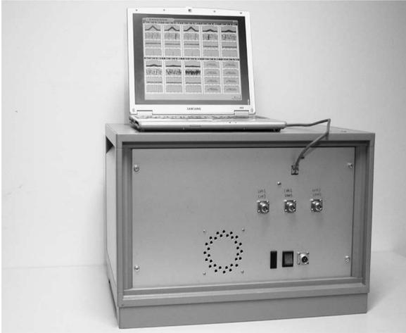
Fig. 2. View of the GOLD-RTR instrument setup. Below are the rack electronics and the back panel interface. The three-jack, N-type antenna input connectors, the power connector and switch, the ventilation outlets, and the Ethernet connector can be identified. The UTP cable links the rack and the laptop; the latter stores the real-time computed waveforms sent through the Ethernet.
