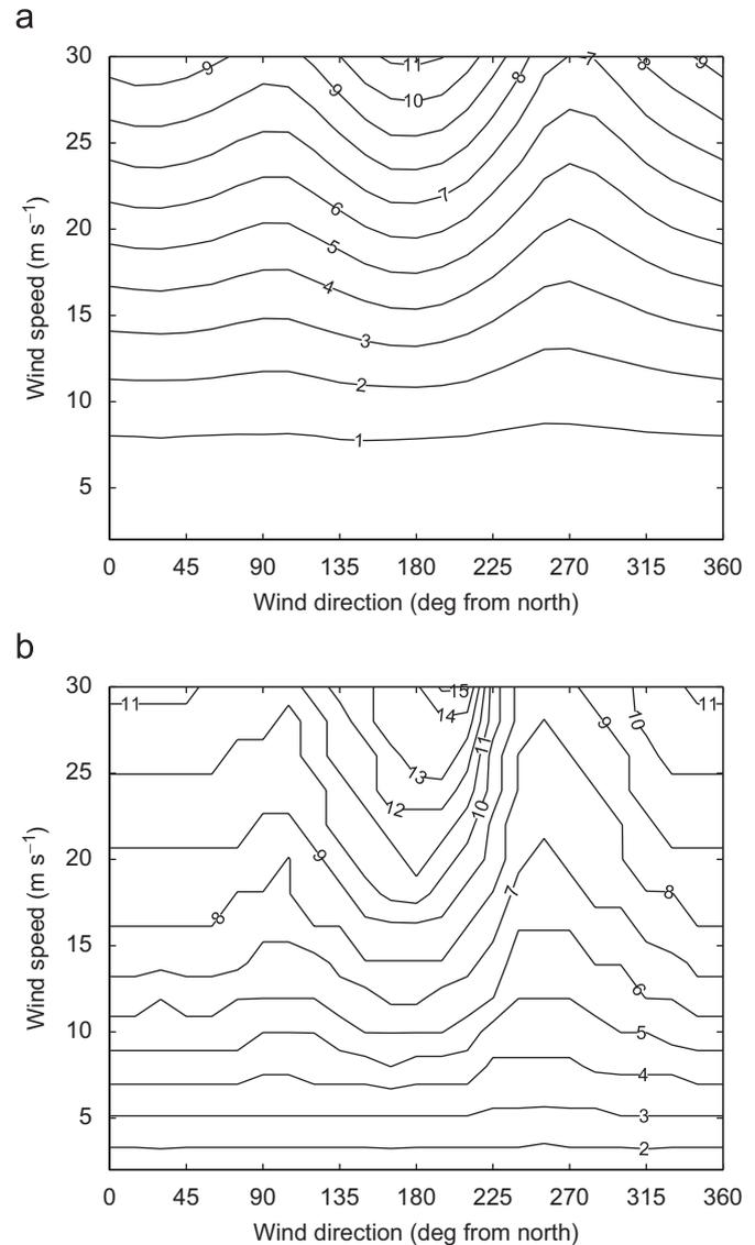
**Fig. 7.** Graphical representation of significant wave height and peak wave period matrices at M2 buoy (for location, see Fig. 5a) based on SWAN stationary wave model of a range of wind speeds and directions. (a)  $H_s$  (m) and (b)  $T_p$  (s).
