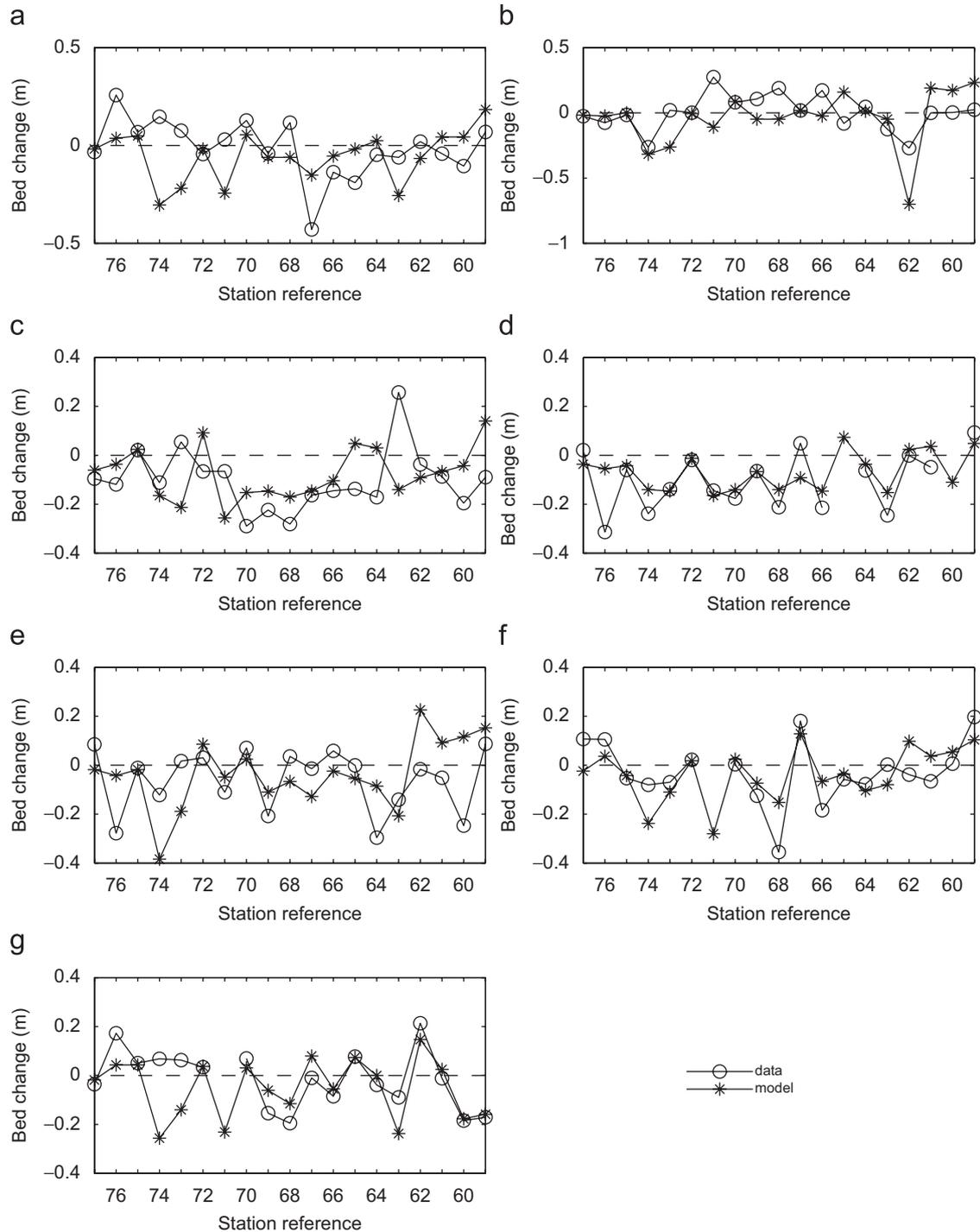
**Fig. 12.** Comparison between modelled and observed change in beach level for all years for all 19 stations: (a) 1997–1998, (b) 1998–1999, (c) 1999–2000, (d) 2000–2001, (e) 2001–2002, (f) 2002–2003 and (g) 2003–2004.
