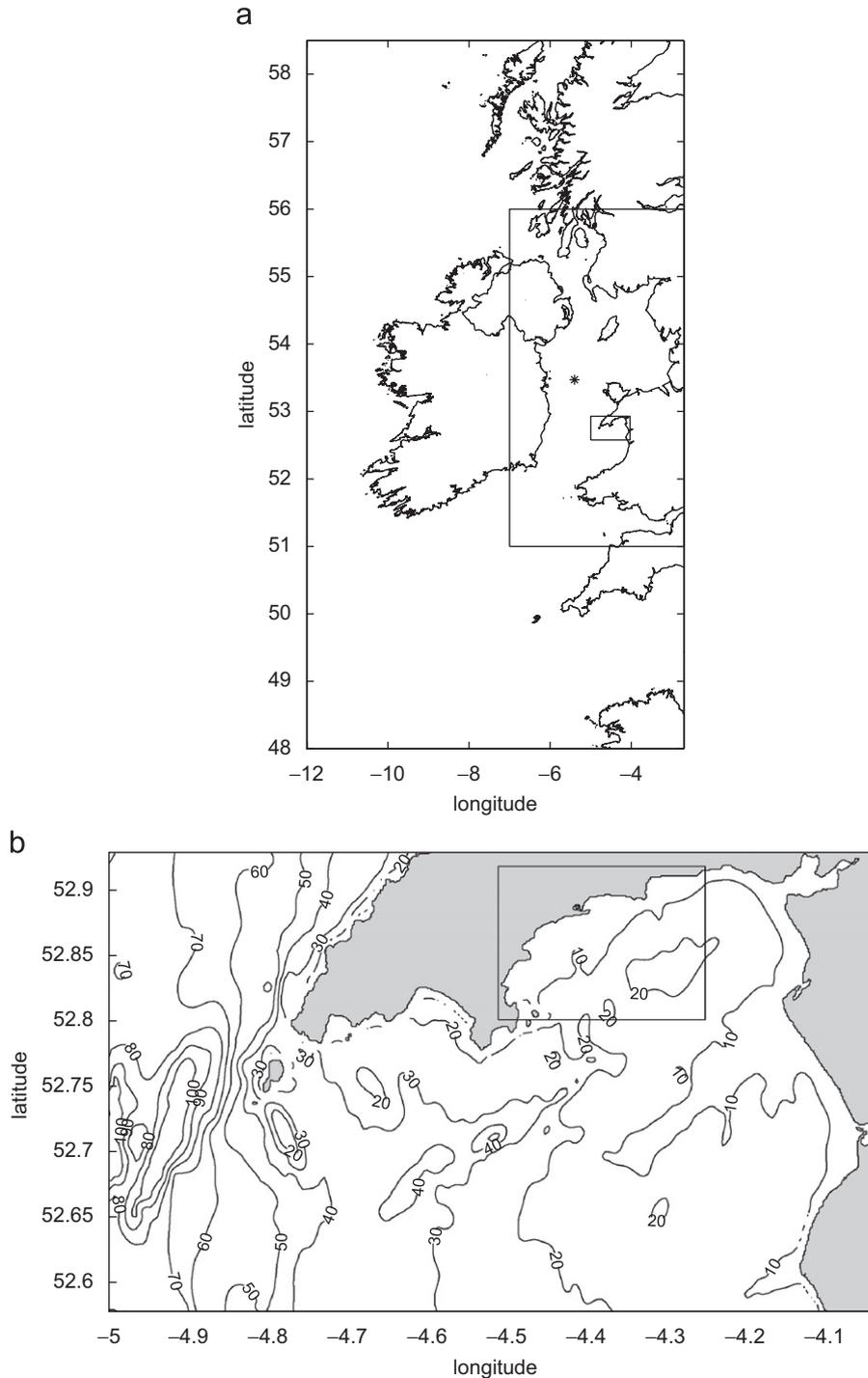
**Fig. 5.** Wave model nests. The asterisk shows the position of the M2 wave buoy (used for validation of the wave model): (a) Shelf Sea, Irish Sea and Tremadoc Bay nests. (b) Tremadoc Bay and Traeth Crugan nests. Contours are of bathymetry (in metres) relative to mean sea level.
