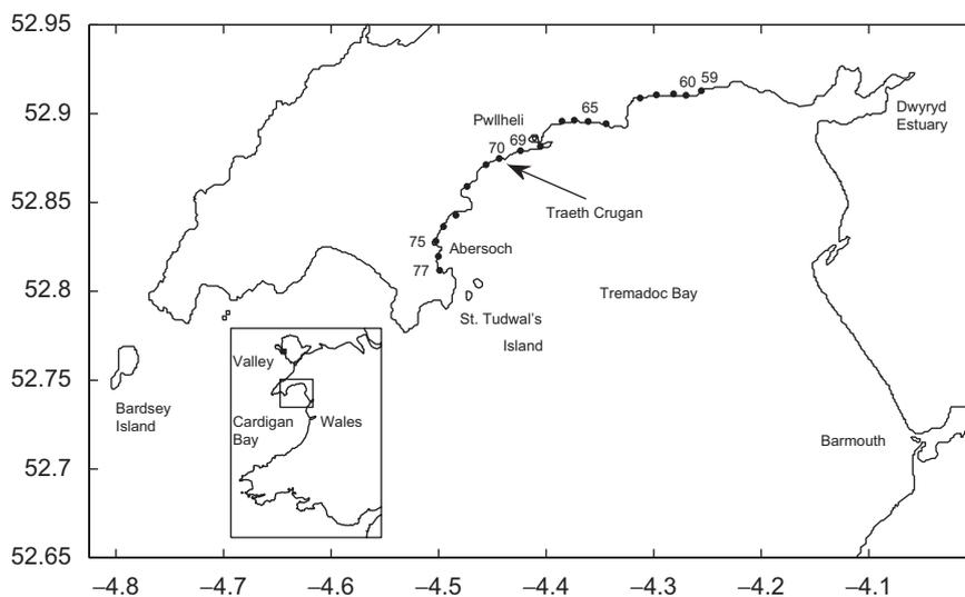
**Fig. 1.** Location of Tremadoc Bay and Traeth Crugan. The 19 beach profile locations are plotted as filled circles, with reference numbers shown for selected stations. Beach profile data was obtained for all stations twice per year from 1997 to 2004.
