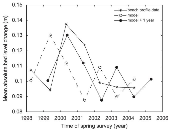
Fig. 13. Mean absolute bed level change for all 19 stations for all 7 years: in situ beach profile data and model data. The model data is also shown lagged by 1 year.
