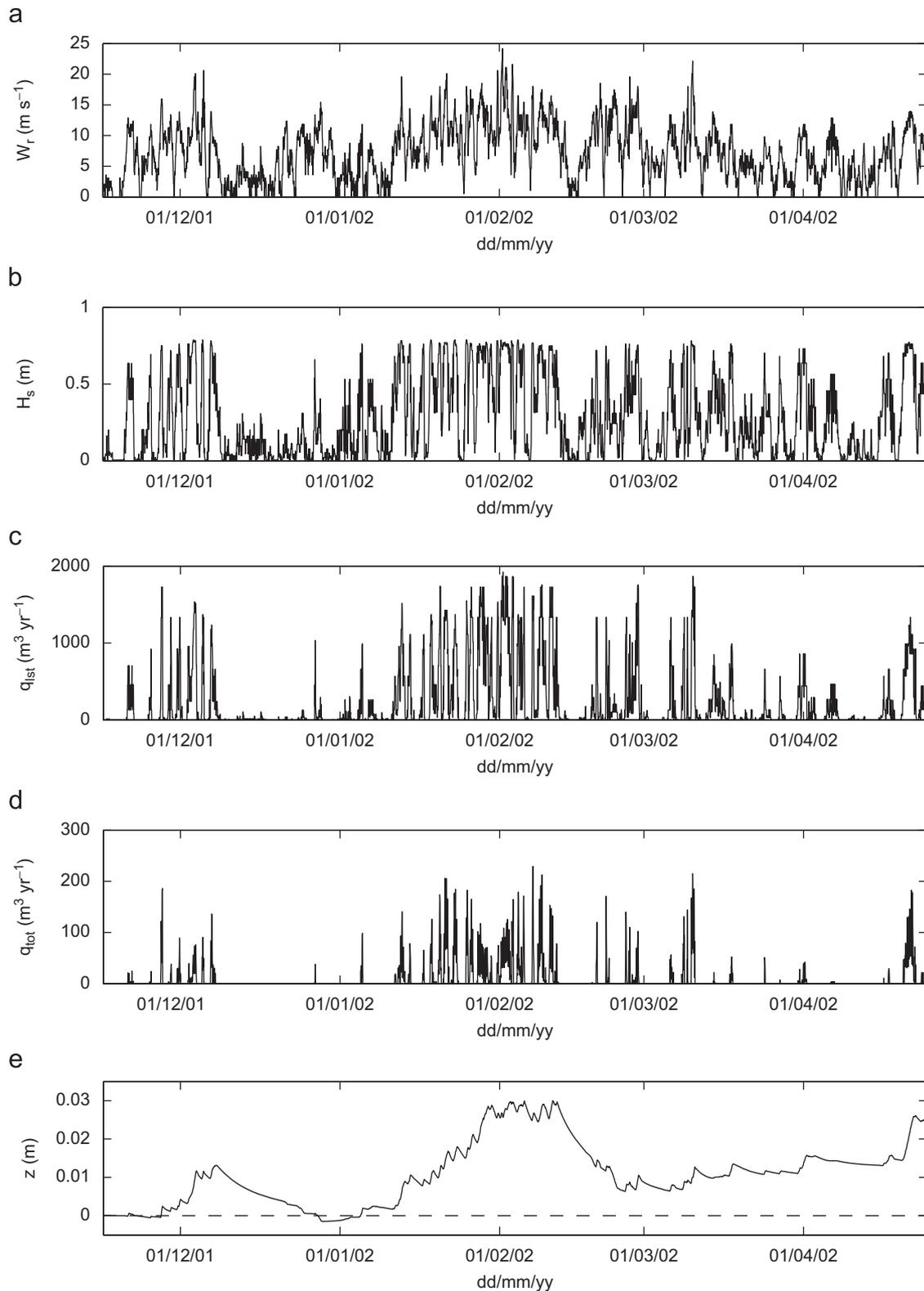
**Fig. 11.** Time series of wind speed (at Valley), significant wave height, longshore transport, total transport and bed level change at Traeth Crugan (station 70) from 16/11/01 to 25/04/02. Longshore transport, wave height and bed level change are output at model grid cell adjacent to the coastline. Total transport is output at the second model grid cell normal to the coastline: (a) wind speed, (b) significant wave height, (c) longshore transport, (d) total transport and (e) bed level change.
