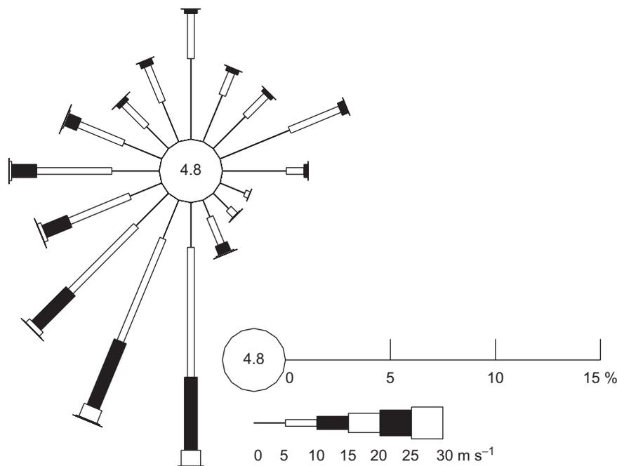
Fig. 2. Wind rose for Valley meteorological station, 1992–2004.
