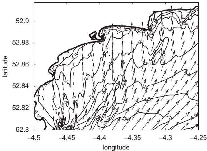
**Fig. 6.** SWAN output from Traeth Crugan model of  $H_s$  contours (m) and vectors of direction  $\theta_p$  with magnitude  $H_s$  for SW wind with speed  $24 \text{ m s}^{-1}$  ( $\sim 47 \text{ kn}$ ). Every tenth modelled vector is shown for clarity.
