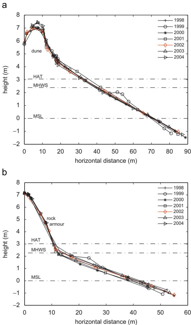
**Fig. 3.** Annual (spring) beach profile surveys for years 1998–2004. The levels of mean sea level (MSL), mean high water springs (MHWS) and highest astronomical tide (HAT) are plotted as dot-dashed lines: (a) station 69 (dune system) and (b) station 70 (rock armour).
