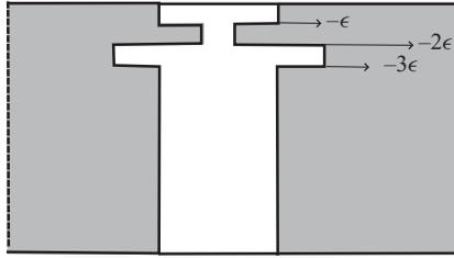
FIGURE 11. Obstacle producing trapped modes and violating the sufficient condition.
