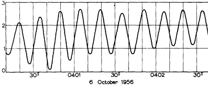
Fig. 2. Short section of Vibrotron record at the protected station of Guadalupe Island. The scale gives inches of water pressure on the sea bottom.
