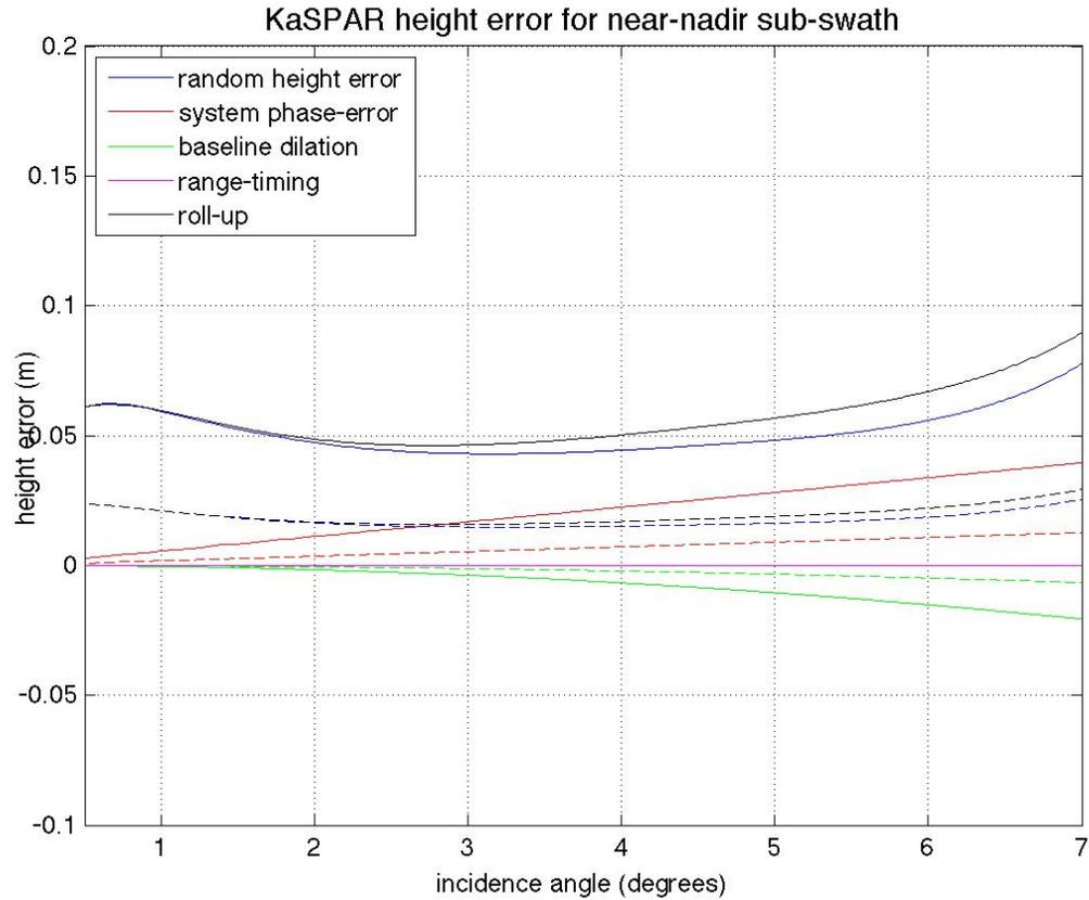
**Figure 2:** Elevation accuracy of the inner subswath. The solid lines are for the short “SWOT-like” elevation baseline, while the dashed line are for the longer cross-track baseline. The posting is 20m in range, but ~80m along-track as limited by the ~3ms decorrelation time assumed for a 6m/s wind.
