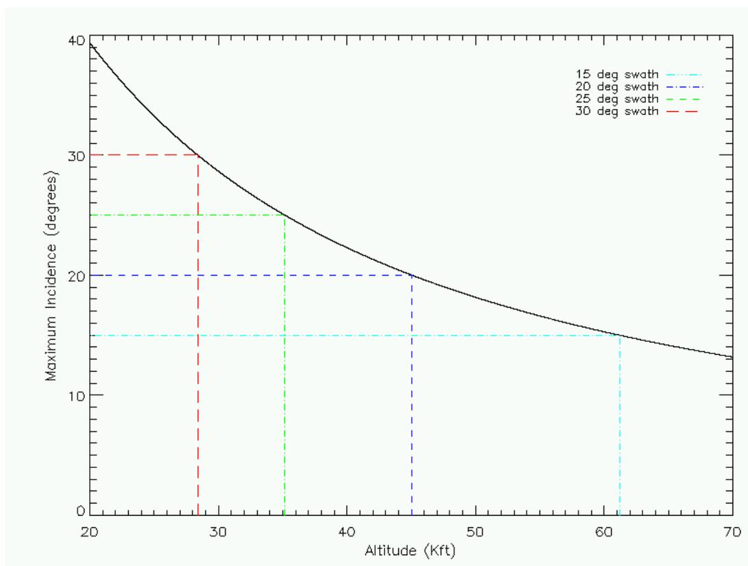
**Figure 2:** Trade of aircraft altitude versus incidence angle to meet a 5km swath. Because the scattering cross-section of water falls off quickly at large incidence angles, there is a distinct advantage to higher operational elevations.
