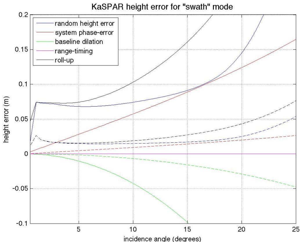
**Figure 3:** Elevation accuracy of the inner subswath. The solid lines are for the short “SWOT-like” elevation baseline, while the dashed line are for the longer cross-track baseline and assume ping-pong. The posting is 50m in range, but ~80m along-track as limited by the ~3ms decorrelation. In order to meet requirements a nadir altimeter mode is necessary to correct the systematic biases.
