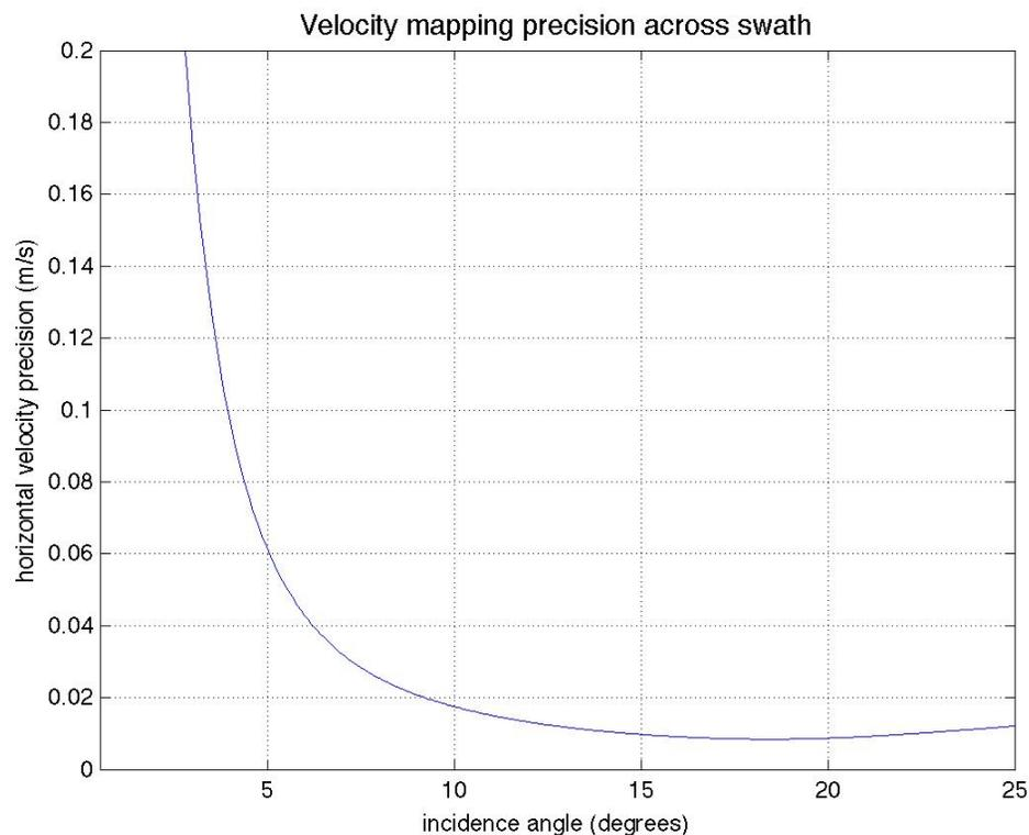
**Figure 4:** Radial velocity performance across swath. As a supporting measurement the velocity can be used in conjunction with slope in discharge estimation for example, or give supporting hydraulics information. The radial component only is measured. The posting is 50m in range, but ~80m along-track as limited by the ~3ms decorrelation.
