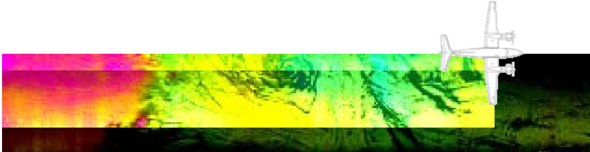
**Figure 1: Cartoon concept of KaSPAR with two overlapping swaths**
