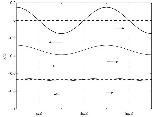
**Fig. 5** The wave velocity field and streamlines at an instant in time. From Eqs. 10a and 10b. Notice that  $D = \hat{\eta} + h$
