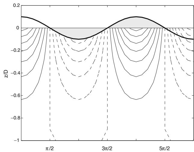
**Fig. 6** The wave pressure field at an instant in time. In the range,  $0 > z > -D$ , pressure is given by Eq. 14b. At  $z=0$ , the interior pressure (solid are positive, dashed lines are negative) is balanced hydrostatically by the product of  $g$  and the elevation, Eq. 14a
