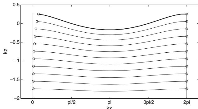
**Fig. 2** Particle trajectories (and streamlines) under a wavy wall for particles launched at  $kx=2\pi$  and after a time,  $2\pi/(ku_0)$ . In this example,  $ka=0.2$ . The arrival deviation at  $kx=0$  is Stokes drift
