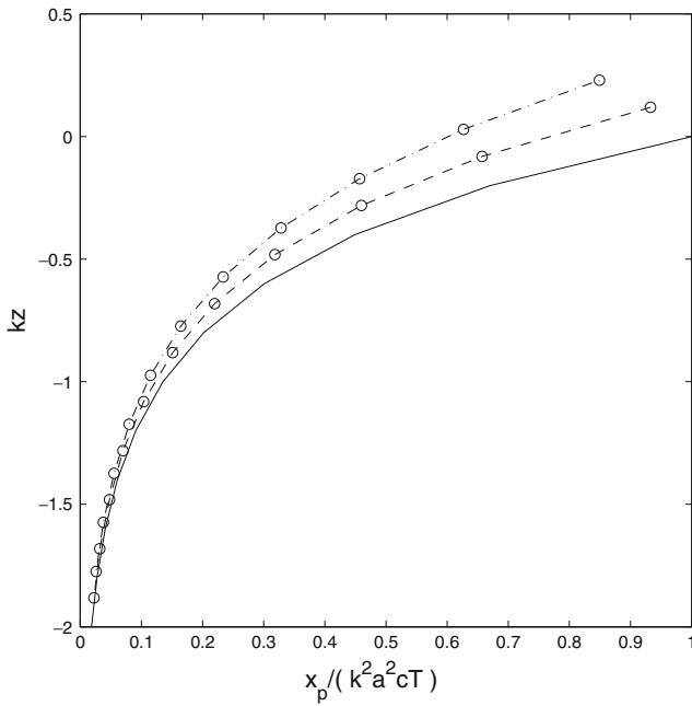
**Fig. 3** Stokes drift for a progressive wave showing the distance traveled by particles after a wave period. The curves are labeled as in Fig. 1. The curve for  $ka=0.2$  yields the Stokes drift “deviation” in Fig. 2 after multiplication by  $2\pi(ka)^2$ . The solid line is the theoretical Stokes drift,  $x_p=(ka)^2cTe^{2kz}$  as determined in “Appendix 1”
