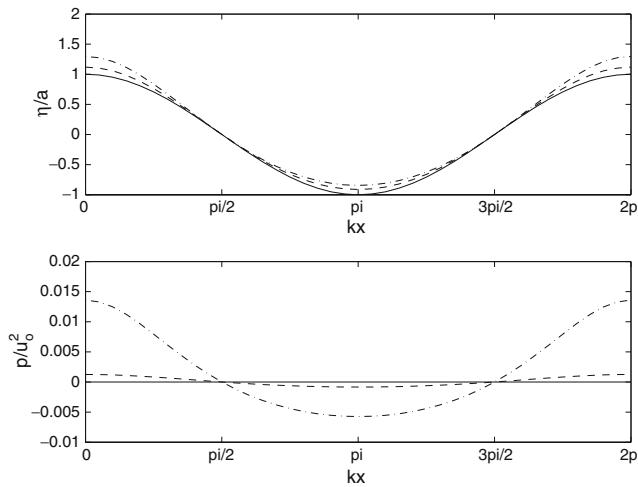
**Fig. 1** Top panel: wall boundary for  $ka=0$  (solid line),  $ka=0.1$  (dashed line),  $ka=0.2$  (dot-dashed line). Bottom panel: wall pressure for the same values of  $ka$
