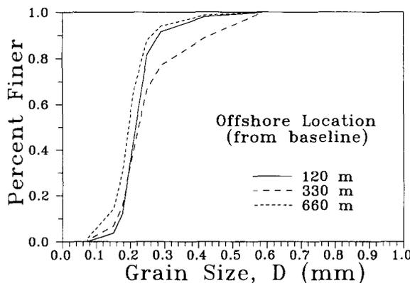
Fig. 8. Grain size distributions at different offshore locations determined by the eigenvector combinations associated with the first temporal eigenvector.
