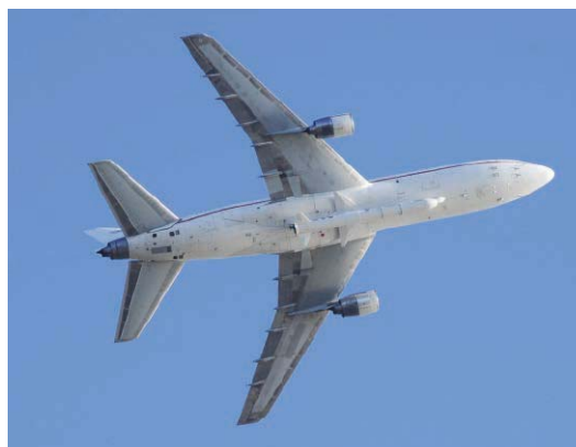
Photo. Pegasus XL expendable rocket affixed to the bottom of the L-1011 Stargazer. Image credit: NASA
