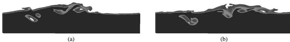
Fig. 3. Counter-rotative and co-rotative vortices – zoom, frontside view of the domain. (a) t = 0.35 s, (b) t = 0.41 s.
