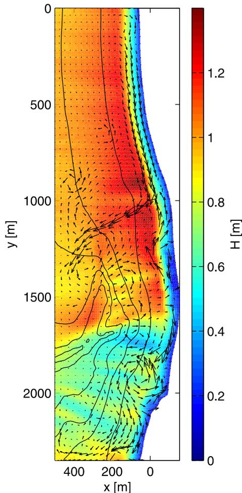
**Figure 4.** Predicted root-mean-square wave height for October 10, 2003 at 1900 GMT within the circulation model domain (Blacks Beach). Black vectors represent the predicted 10-minute averaged circulation patterns. Depth contours (black) correspond to the 0, 5, 10, 15, 25, 50, and 100 m contours.
