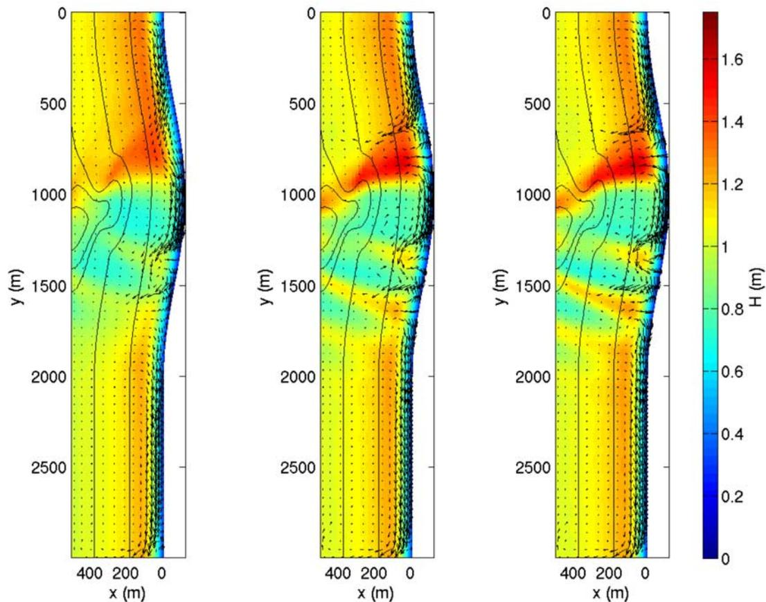
**Figure 18.** Predicted velocity field (black vectors) superimposed on the predicted root-mean-square wave height for the following wave conditions: JONSWAP spectrum with  $H_s = 1.5$  m,  $T_p = 10$  s,  $\theta_p = 285$  degrees,  $\gamma = 10$ , and (left)  $m = 4$ , (middle)  $m = 24$ , (right)  $m = 40$ . Depth contours (black) correspond to the 0, 5, 10, 15, 25, and 50 m contours.
