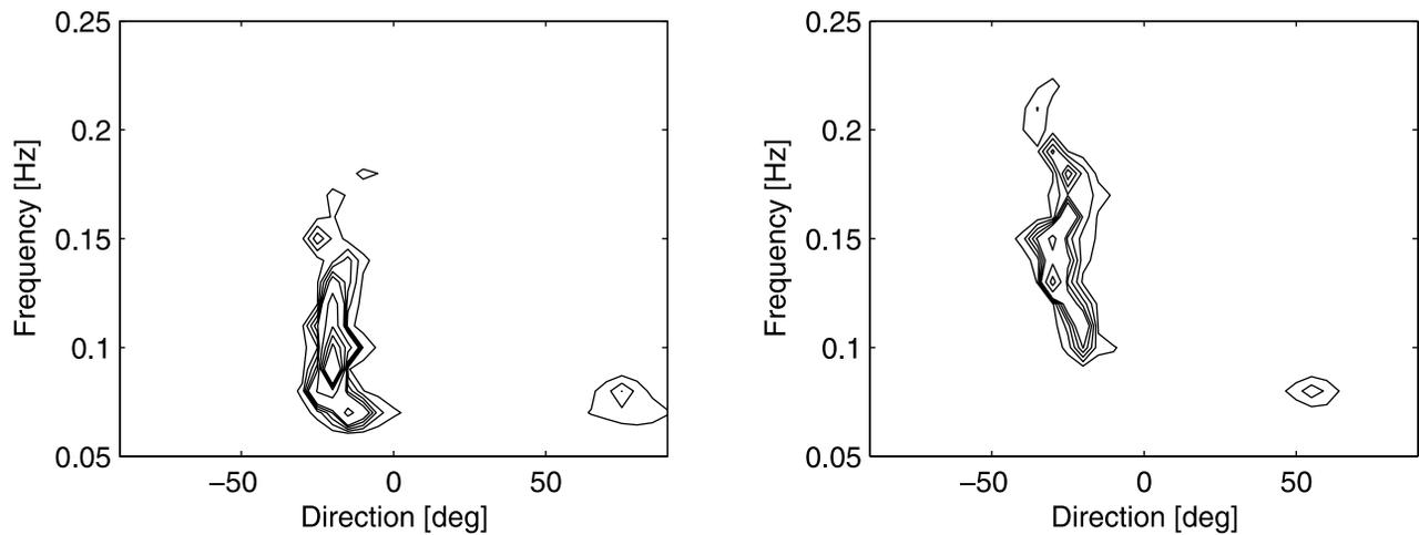
**Figure 2.** Variance density ( $\text{m}^2/\text{Hz}/\text{degree}$ ) of the wave spectra collected at the offshore wave buoy for October 10, 2003 at 1900 GMT (left) and October 31, 2003 at 1500 GMT (right). Contour lines of variance density correspond to the 0, 0.01, 0.02, 0.03, 0.04, 0.05, 0.1, 0.15, 0.2, and 0.25  $\text{m}^2/\text{Hz}/\text{degree}$  contours.
