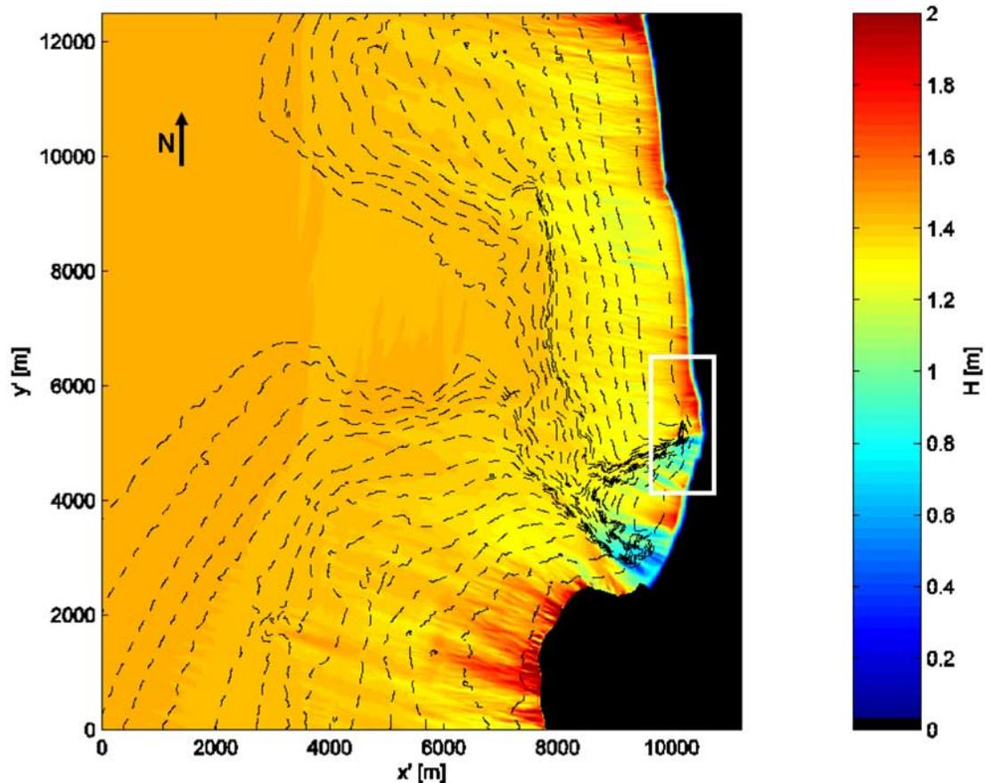
**Figure 3.** Predicted significant wave height for October 10, 2003 at 1900 GMT. Depth contours are shown in black in 10 m increments from the 0 m to 100 m contours and in 50 m increments from the 100 m to 300 m contours. Highlighted region denotes the circulation model domain.
