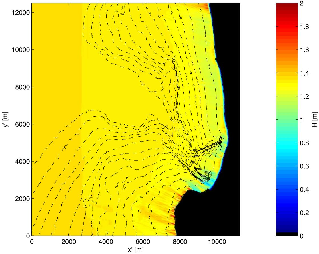
**Figure 6.** Predicted significant wave height (SWAN) for October 31, 2003 at 1500 GMT. Depth contours are shown in black in 10 m increments from the 0 m to 100 m contours and in 50 m increments from the 100 m to 300 m contours.
