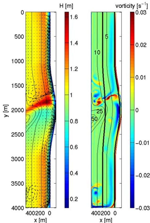
**Figure 10.** Predicted root-mean-square wave height variation (left) and final snapshot of vorticity (right) for the theoretical case described by an oblique canyon and curved shoreline. Thick black lines in the right panel indicate the transects where the alongshore momentum balances will be evaluated as discussed in section 4.2.
