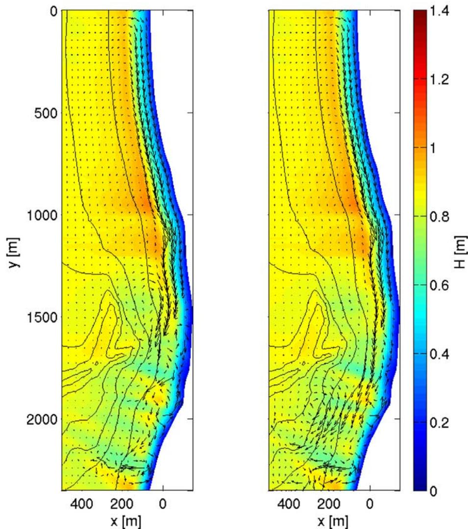
**Figure 8.** Predicted root-mean-square wave height for October 31, 2003 at 1500 GMT within the circulation model domain (Blacks Beach). Black vectors represent the predicted 10-minute averaged circulation patterns after a 45-minute simulation (left) and a 90-minute simulation (right). Depth contours (black) correspond to the 0, 5, 10, 15, 25, 50, and 100 m contours.
