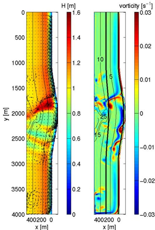
**Figure 12.** Predicted root-mean-square wave height variation (left) and final snapshot of vorticity (right) for the theoretical case described by an oblique canyon with undulating contours and curved shoreline. Thick black lines in the right panel indicate the transects where the alongshore momentum balances will be evaluated as discussed in section 4.2.
