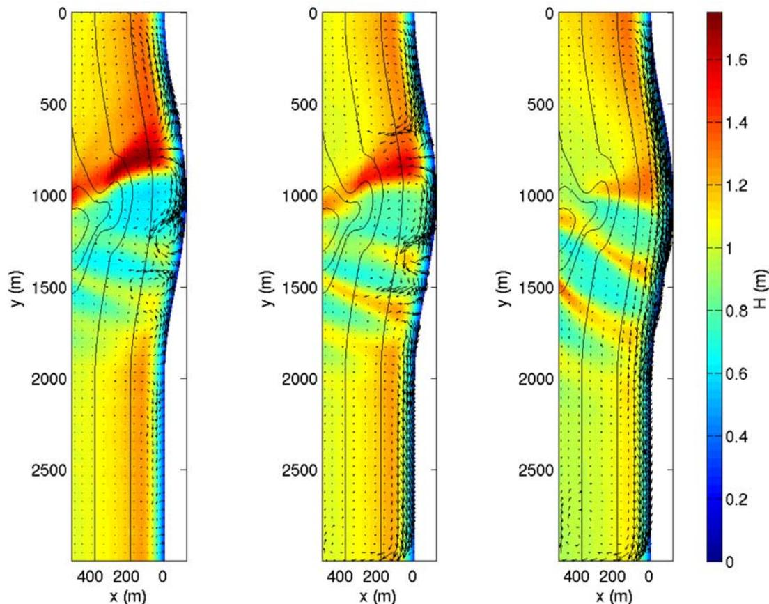
**Figure 17.** Predicted velocity field (black vectors) superimposed on the predicted root-mean-square wave height for the following wave conditions: JONSWAP spectrum with  $H_s = 1.5$  m,  $T_p = 10$  s,  $\gamma = 10$ ,  $m = 40$  and (left)  $\theta_p = 270$  degrees (normally incident), (middle)  $\theta_p = 285$  degrees, (right)  $\theta_p = 315$  degrees. Depth contours (black) correspond to the 0, 5, 10, 15, 25, and 50 m contours.
