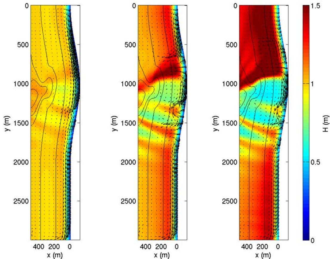
**Figure 16.** Predicted velocity field (black vectors) superimposed on the predicted root-mean-square wave height for the following wave conditions: JONSWAP spectrum with  $H_s = 1.5$  m,  $\theta_p = 285$  degrees,  $\gamma = 10$ ,  $m = 40$ , and (left)  $T_p = 6$  s, (middle)  $T_p = 10$  s, (right)  $T_p = 14$  s. Depth contours (black) correspond to the 0, 5, 10, 15, 25, and 50 m contours.
