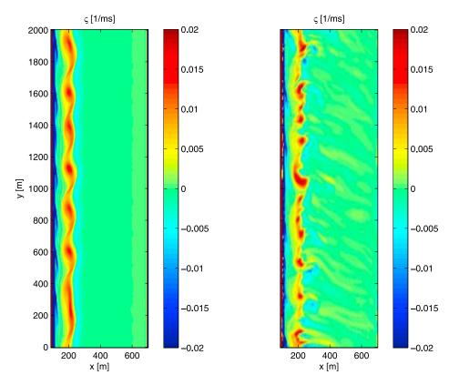
**Figure 15.** Oblique random wave group sequence. Snapshots of the vorticity field in two cases: (left) no offshore wave groups and (right) a wavefield with the same offshore peak characteristics ( $H_{mean} = 1 \text{ m}$ ,  $T_p = 10 \text{ s}$ ,  $\theta = -20^\circ$ ) and an offshore groupiness factor of GF = 0.6. The snapshot is taken at t = 75 min.
