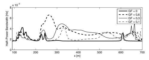
Figure 19. Unstable alongshore mean current. Half-power bandwidth of the frequency–wave number spectra of potential vorticity (integrated over all wave numbers) versus cross-shore distance for GF = 0(thick solid line), GF = 0.1 (thin dashed line), GF = 0.3 (thin solid line), and GF = 0.6 (thick dashed line).
