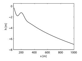
**Figure 1.** Alongshore uniform barred beach profile used as model bottom boundary condition.
