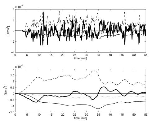
**Figure 9.** Normally incident random wave group sequence. (top) Enstrophy balance integrated over all alongshore positions and from the bar trough to the offshore boundary. Thick solid line,  $ENS_t$ ; dashed line,  $PROD_{wave}$ ; dotted line, MIX; thin solid line, FRIC. (bottom) The low-pass-filtered (T > 200 s) potential enstrophy balance.
