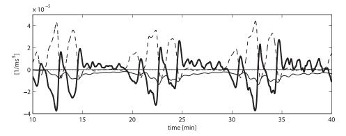
**Figure 6.** Simplified wave group sequence. Enstrophy balance integrated over all alongshore positions and from the bar trough to the offshore boundary. Thick solid line,  $ENS_t$ ; dashed line,  $PROD_{wave}$ ; dotted line, MIX; thin solid line, FRIC.
