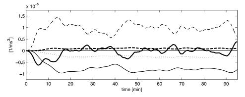
**Figure 12.** Random wave groups with stable alongshore mean current. Low-pass-filtered (T > 200 s) potential enstrophy balance integrated over all alongshore positions from the bar trough to the offshore boundary. Thick solid line,  $ENS_t$ ; thick dashed line,  $PROD_{shear}$ ; thin dashed line,  $PROD_{wave}$ ; dotted line, MIX; thin solid line, FRIC.
