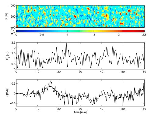
**Figure 7.** Normally incident random wave group sequence. (top) Time-space plot of root-mean-square wave height at the offshore boundary with GF = 0.63, where the white line denotes the location of (middle) the time series at y = 344 m. (bottom) Time series of cross-shore velocity (solid line) and low-pass-filtered (T > 200 s) cross-shore velocity (dashed line) at x = 223 m, y = 344 m (inside the surf zone).
